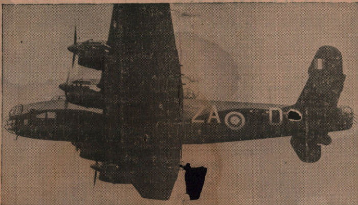
The Handley Page Halifax bomber which, with the Stirling and other heavy types, forms the spearhead of the sustained British R. A. F. offensive on Germany, has been engaged on many heavy raids, some on Berlin when the devastating effect of its huge bomb-load has been brought home forcibly to the enemy. An all-metal mid-wing monoplane, its wing span is 99 ft., length 70 ft., and height 22 ft. Powered with four Rolls-Royce Merlin 12-cylinder liquid-cooled engines, it has three-bladed airscrews and carries heavy defensive armament. A Halifax bomber is here shown in flight.
