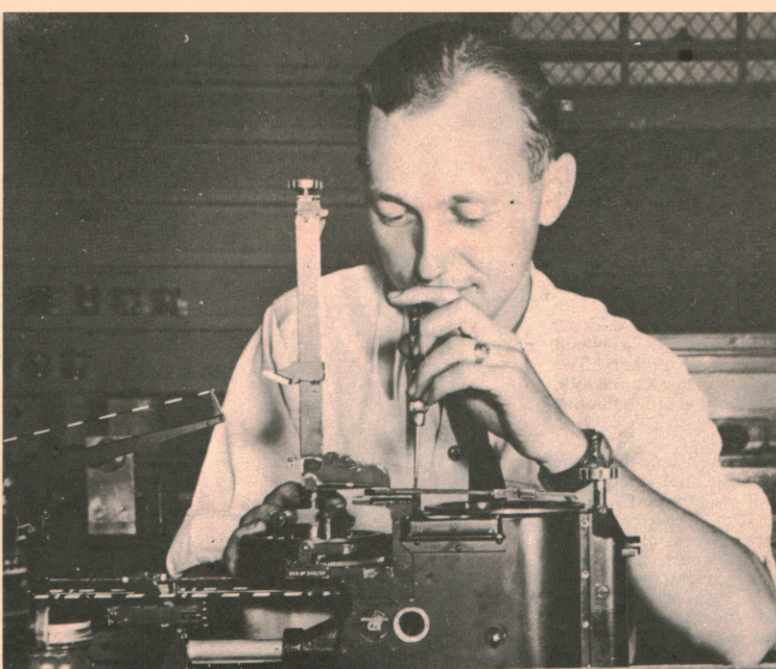
Air bombers rely on the craftman hands of instrument mechanics. Here LAC Stanley Topping, Toronto, repairs a bombsight calibrated to one ten-thousandth of an inch.
