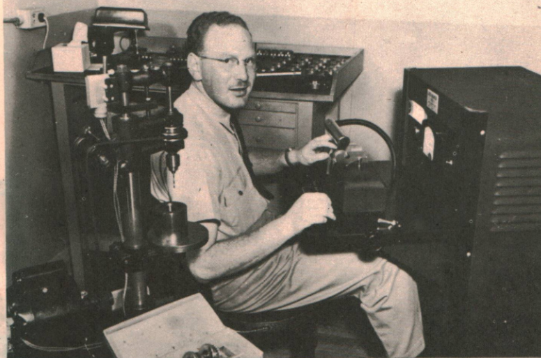
The rotor is the brain of "George", automatic pilot. Correcting a rotor's balance is exclusive job of LAC Cy Harris, operating the only balancing machine in Canada.
