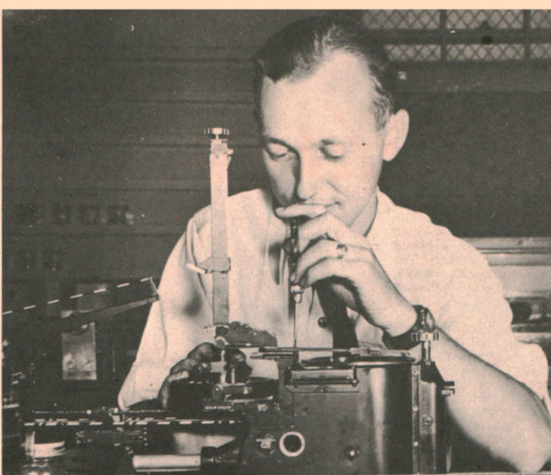
Air bombers rely on the craftman hands of instrument mechanics. Here LAC Stanley Tepping, Toronto, repairs a bombsight calibrated to one ten-thousandth of an inch.
