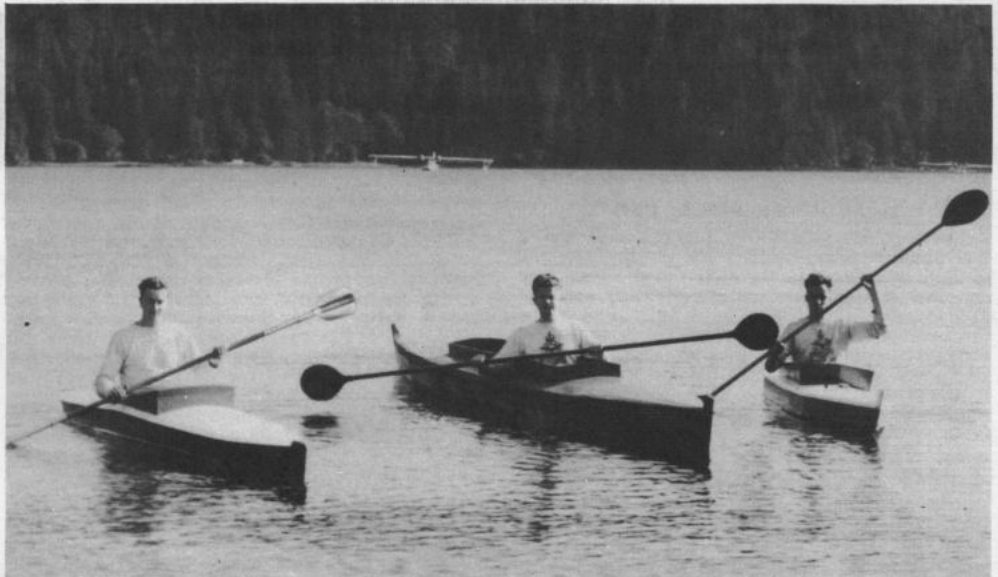
Scrounged aircraft fabric doped to Queen Charlotte spruce created kayaks for these contriving Eskijoes. L. to R.: LACs F. G. Cameron, Glace Bay, H. T. Rouse, Hamilton, and E. A. Lockert, Regina.
