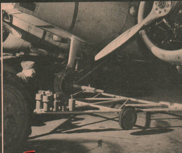
FS HARRY FEINBERG'S UNIVERSAL TOWING GEAR DESIGNED TO HAUL ANY SIZE KITE
