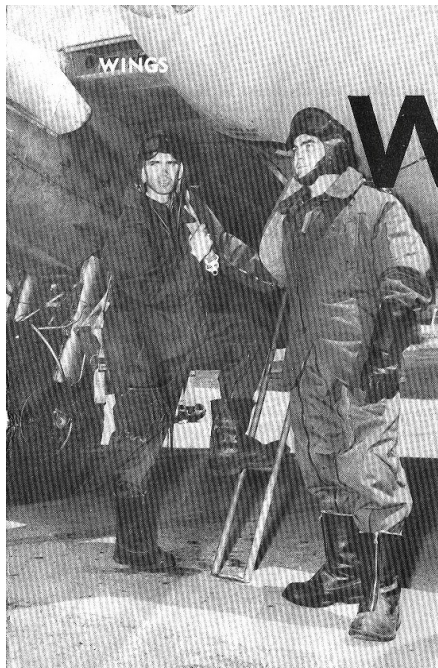
NEW TWO PIECE winter flying suit, right, in contrast with present issue. Both coat and pants have "disengage" zippers for quick escape in emergency. Pencil pocket on sleeve, watch pocket on chest, were asked for by aircrew.
