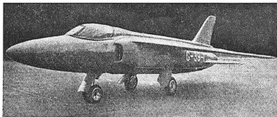
Powered by an Armstrong Siddeley Viper ASV 5 engine of 1,610lb. thrust, the Folland Midge is the prototype of the Gnat light fighter, which will have the much more powerful Bristol Orpheus turbo-jet.
