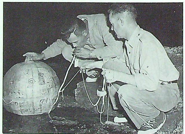
S/L R. G. Connick, Officer Commanding the RCAF's Survival Training School (left) and Sgt. L. M. Murrie of the Institute of Aviation Medicine, check the solar still which is processing sea water into drinking water.
