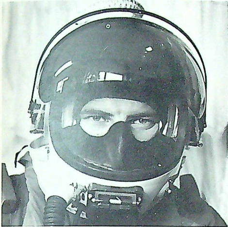
F/L J. R. Chisholm, RCAF, wears personally-fitted helmet, designed to permit pressure breathing at high altitude.
