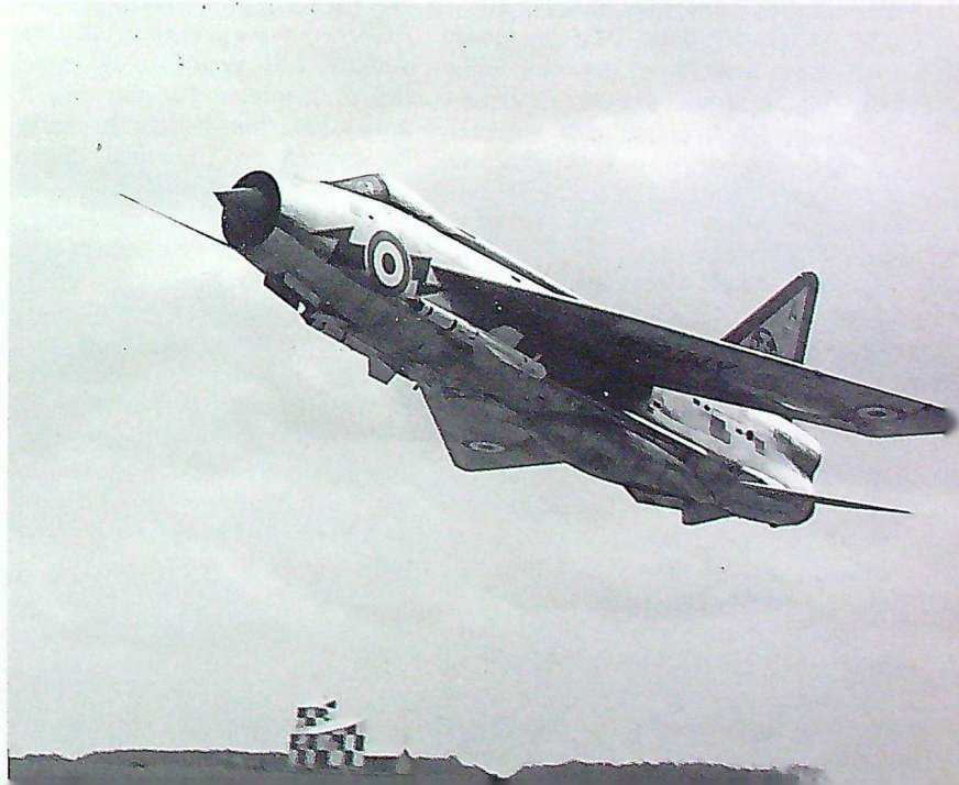
The firestreak-equipped Lightning, with reheat (afterburner), takes one and a half minutes to reach the tropopause (approx. 36,000 ft.).
