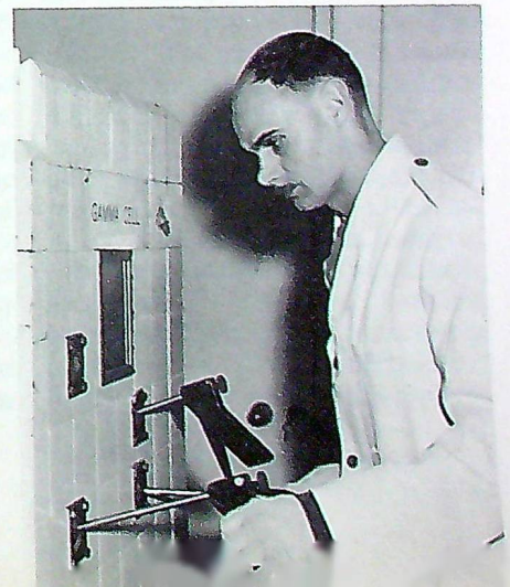
Capt. R. N. Patterson, Black Watch Regt. of Canada, uses remote handling equipment to open isotope can behind lead shielding in radio-chemistry lab.
