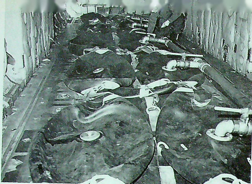
Five four-ply butyl rubber tanks, each capable of holding 800 gal. of fuel-oil, are installed in Hercules' cargo hold for spring re-supply of arctic bases.
