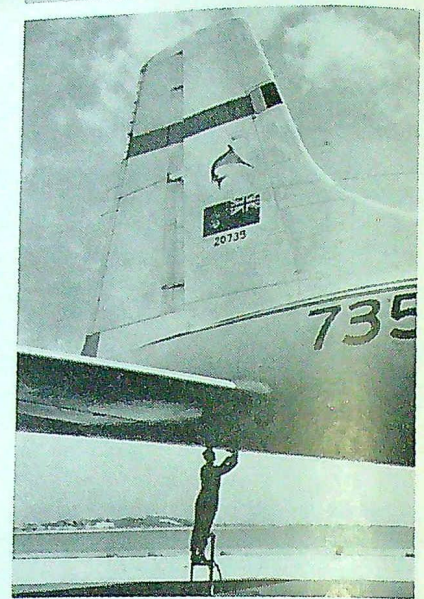
Airman inspects retro-launch doors beneath tail of a No. 415 (Swordfish) Sqn. Argus .
