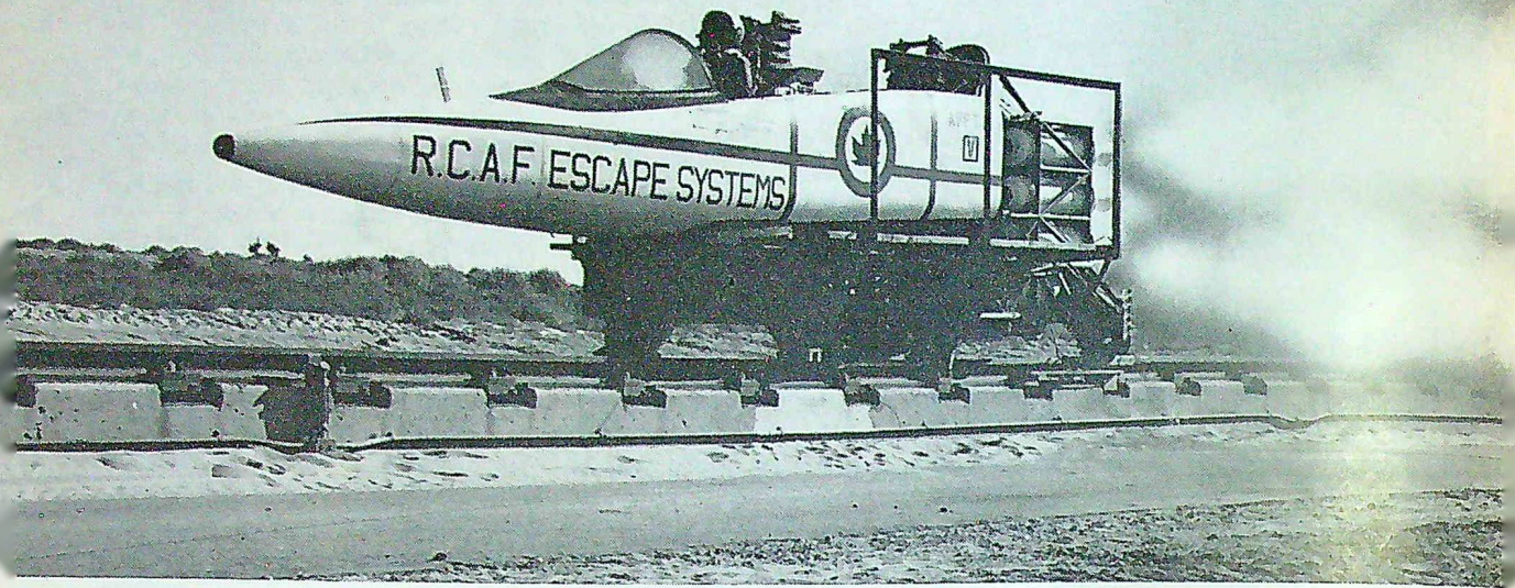
The rockets light up and the sled is on its way down the 20,000 foot track at Edwards USAF base.
