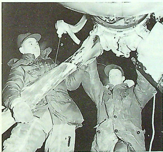
Propeller change for Boxcar in -30^{\circ} at arctic base.
