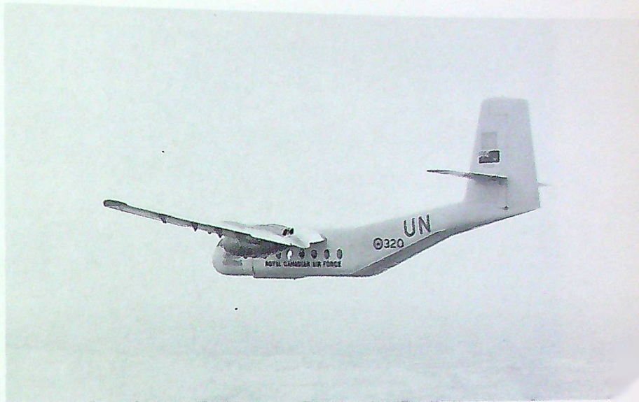
Payload is roughly three tons with fuel for 200 miles. Maximum range (normal tanks) is 1,450 miles. Cruising speed is 182 mph and stalling speed 62 mph.
