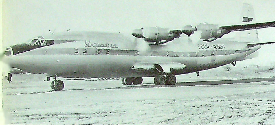
The AN-10 was built to operate from short airfields. It carries 84 passengers and cruises at approximately 370 mph.
