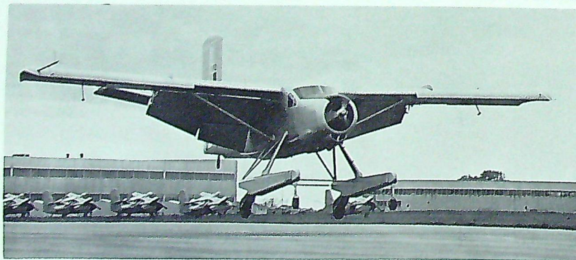
An experimental Otter fitted with special flaps, flies over a Downsview runway at 36 knots.
