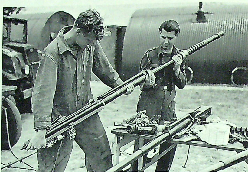
LAC J. Peachell and Cpl. O. Shaw clean the 20mm. cannon from a Nighthawk Mosquito .
