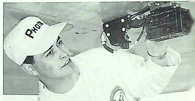
LAC R. Duguay was one of the photo techs responsible for cine cameras, carried under each CF-100 wing, from which assessments of rocket hits were made.
