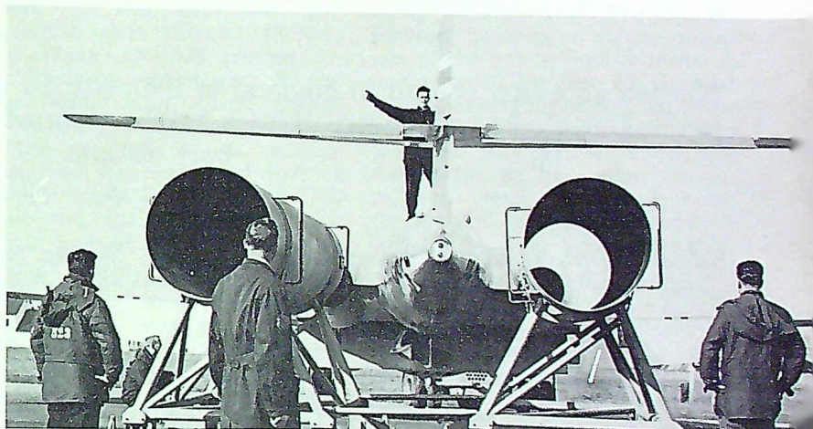
In the last stage of the maintenance cycle a CF-100 is positioned in front of the protective blast tubes for a run-up.
