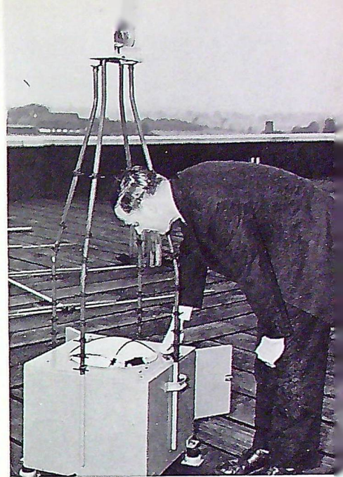
Dr. J. H. Meek, a Defence Research Board scientist, examines an all-sky camera before setting its time clock for automatic pictorial records of the aurora borealis.
