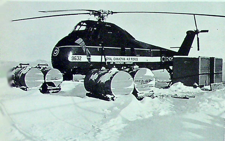
A 108 Comm. Flt. Sikorsky H-34, used to haul diesel fuel for construction vehicles on the MCL.
