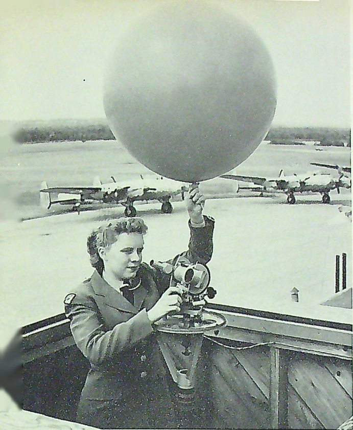
A.W.1 Jean Hay launches a hydrogen-filled balloon preparatory to computing the direction and velocity of the upper winds.
