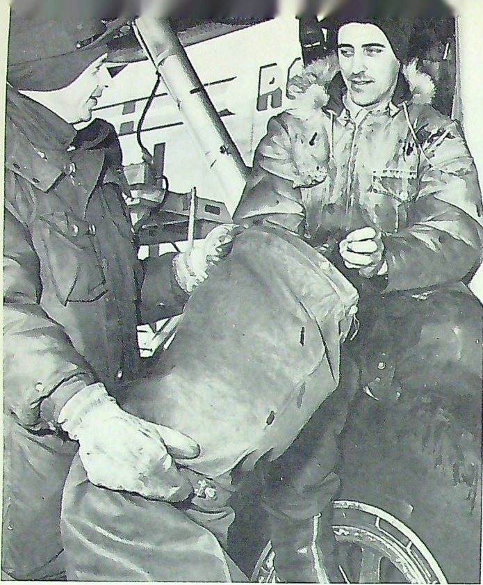
L.A.C. Walls directs a blast of warm air from a Herman Nelson heater towards L.A.C. Rackowski, who is working on the landing-gear of a C-119.
