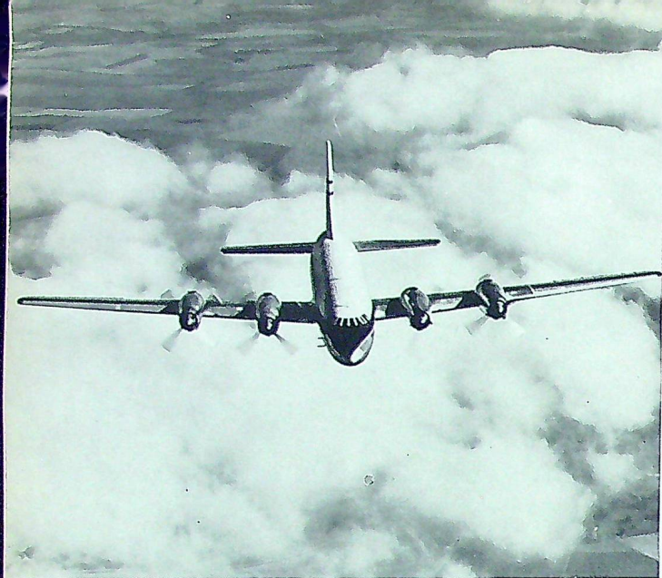
The Bristol Britannia airliner, powered by four Bristol Proteus turbo-prop engines, can carry more than a hundred passengers for 4,000 miles at a cruising-speed of 365 m.p.h.
