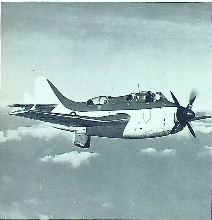
The carrier-borne Fairey Gannet, a three-seater anti-submarine aircraft, can be flown on one of its two Armstrong-Siddeley Double Mamba turbo-prop engines.
