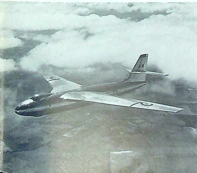
The Vickers Valiant, a long-range bomber with four Rolls-Royce Avon engines.
