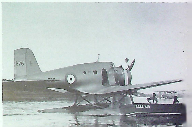
A Delta of No. 8 Squadron being loaded with supplies at Ottawa prior to departure for Sydney, N.S. The Delta, with a cruising speed of about 160 m.p.h. was the first all metal low wing monoplane in the R.C.A.F.
