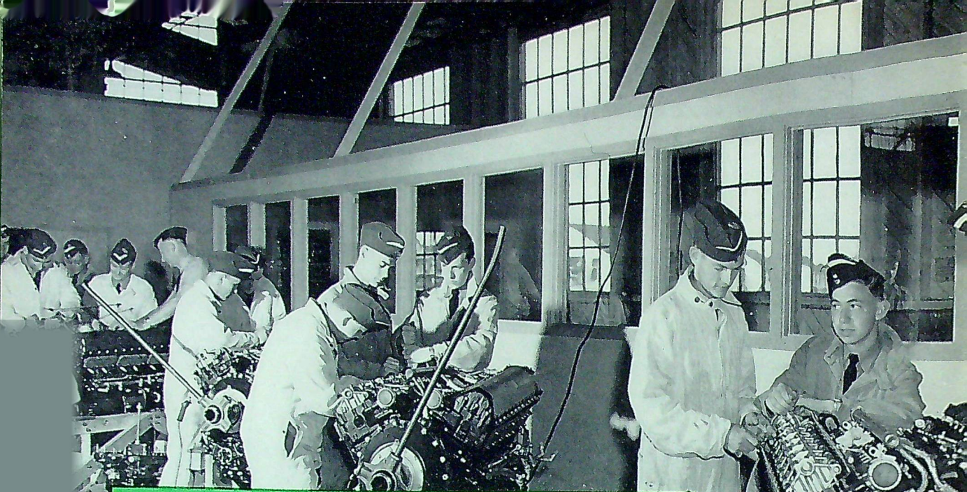
Cadets at Aeronautical Engineering School, Aylmer, timing valves on Merlin engines.
