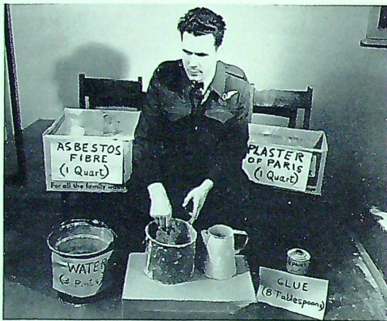
Mixing the plaster. Labels show proportions of ingredients.
