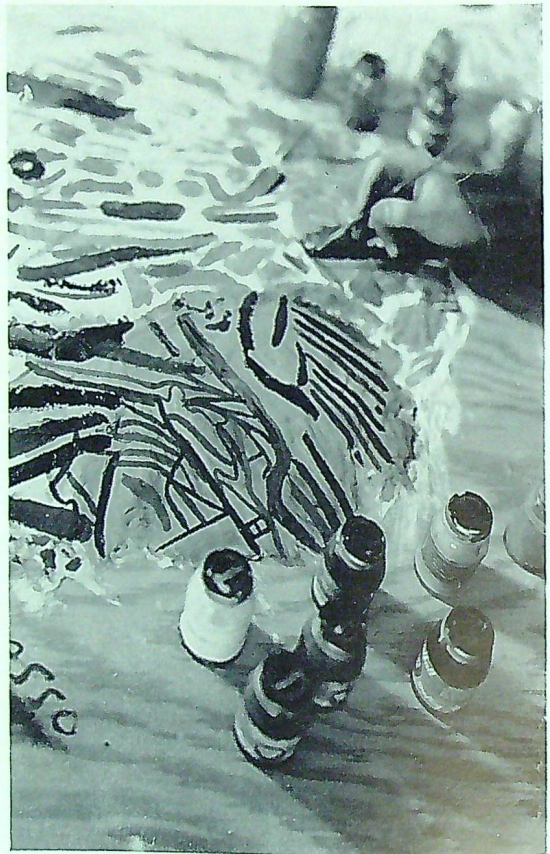
Testing paint colours on samples of hardened plaster
