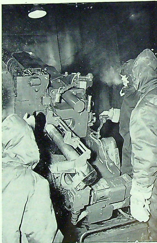
Anti-aircraft gun undergoing low-temperature tests
