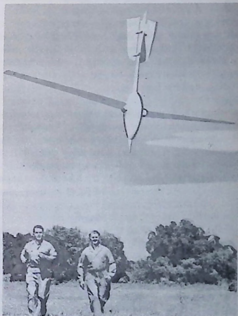
The Rotochute. General Electric Co.'s supersonic parachute for lowering research instruments from rockets. It slows down to 27 m.p.h.
