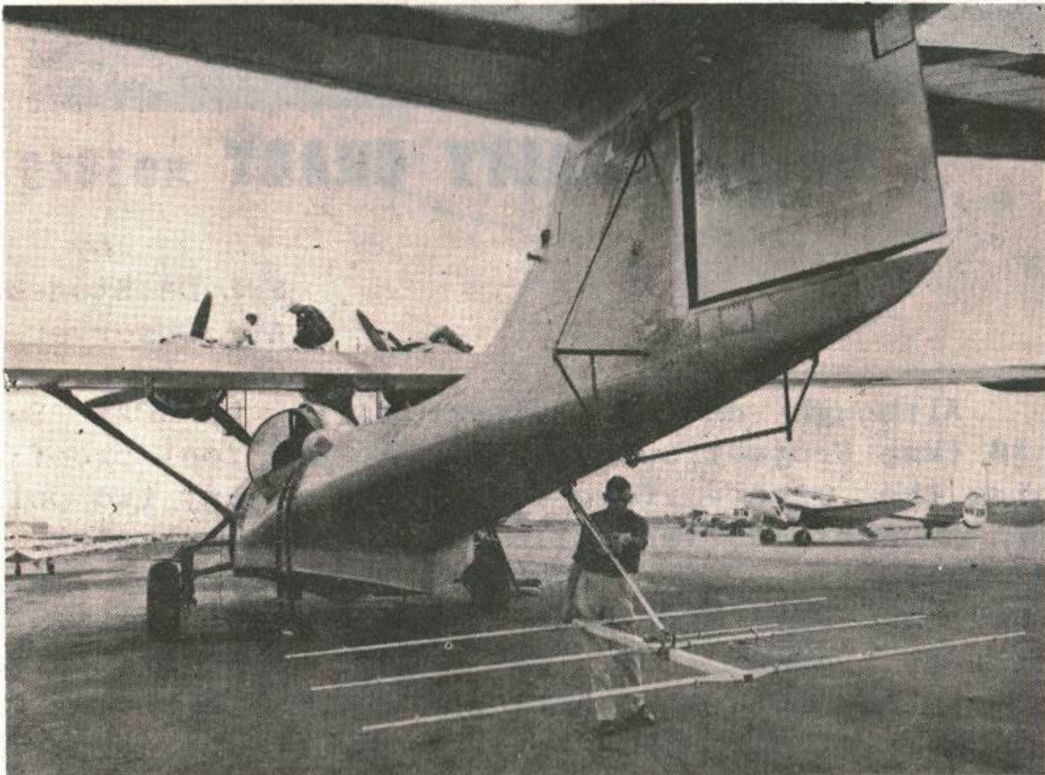
Figure 7 - Aircraft Yagi Antenna for Meteoric Scatter
