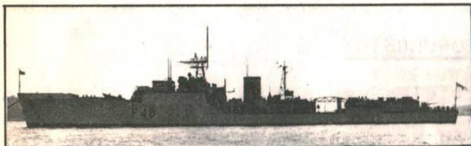
British Coniston Class Coastal Minesweeper Length 152 Ft Beam 29 Ft 360 Tons
