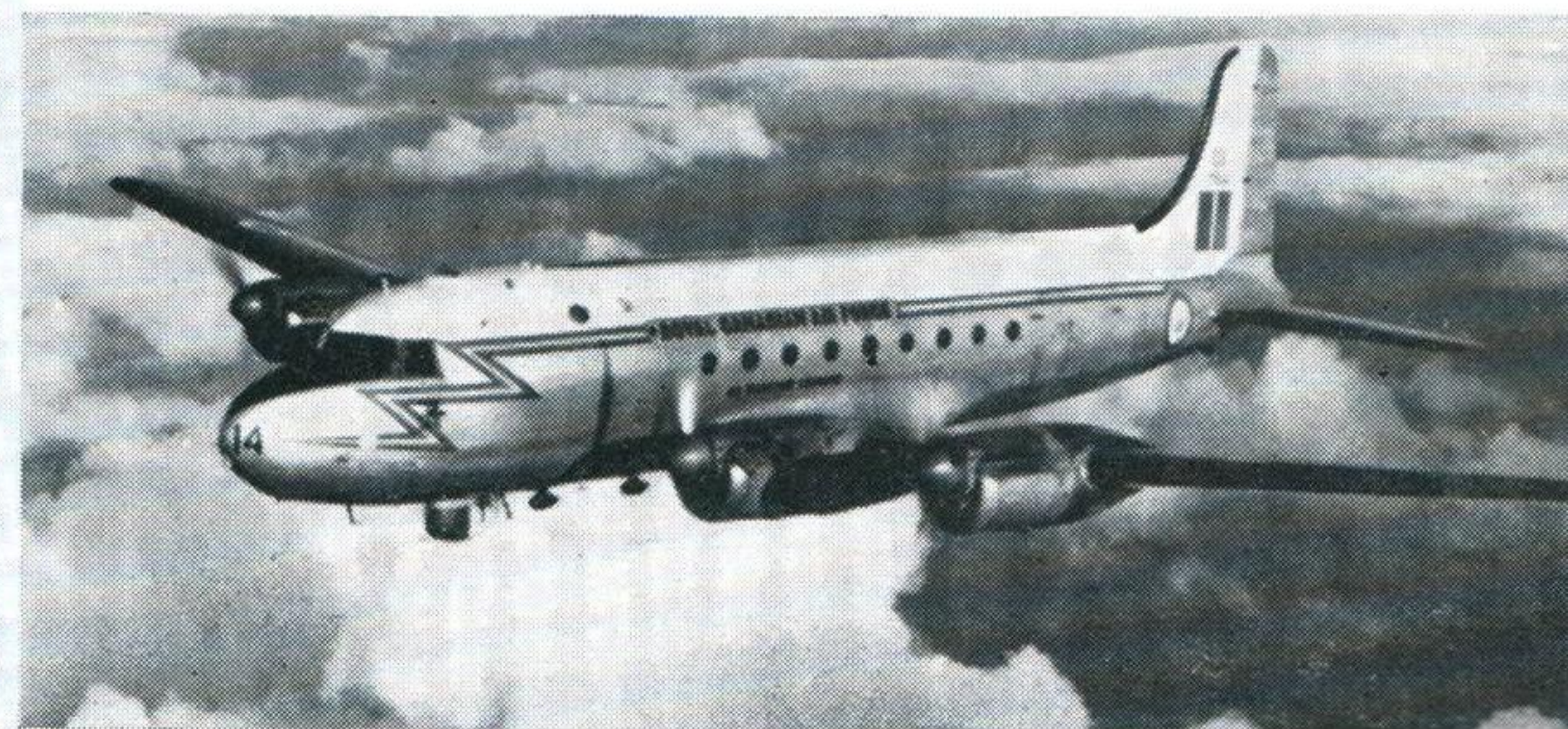
SKYMASTER The DC-4 design, C-54 Skymaster in U.S. service, was built in its thousands. A version built by Canadair for the R.C.A.F. (as per photo) was named North Star. Span 117 feet
