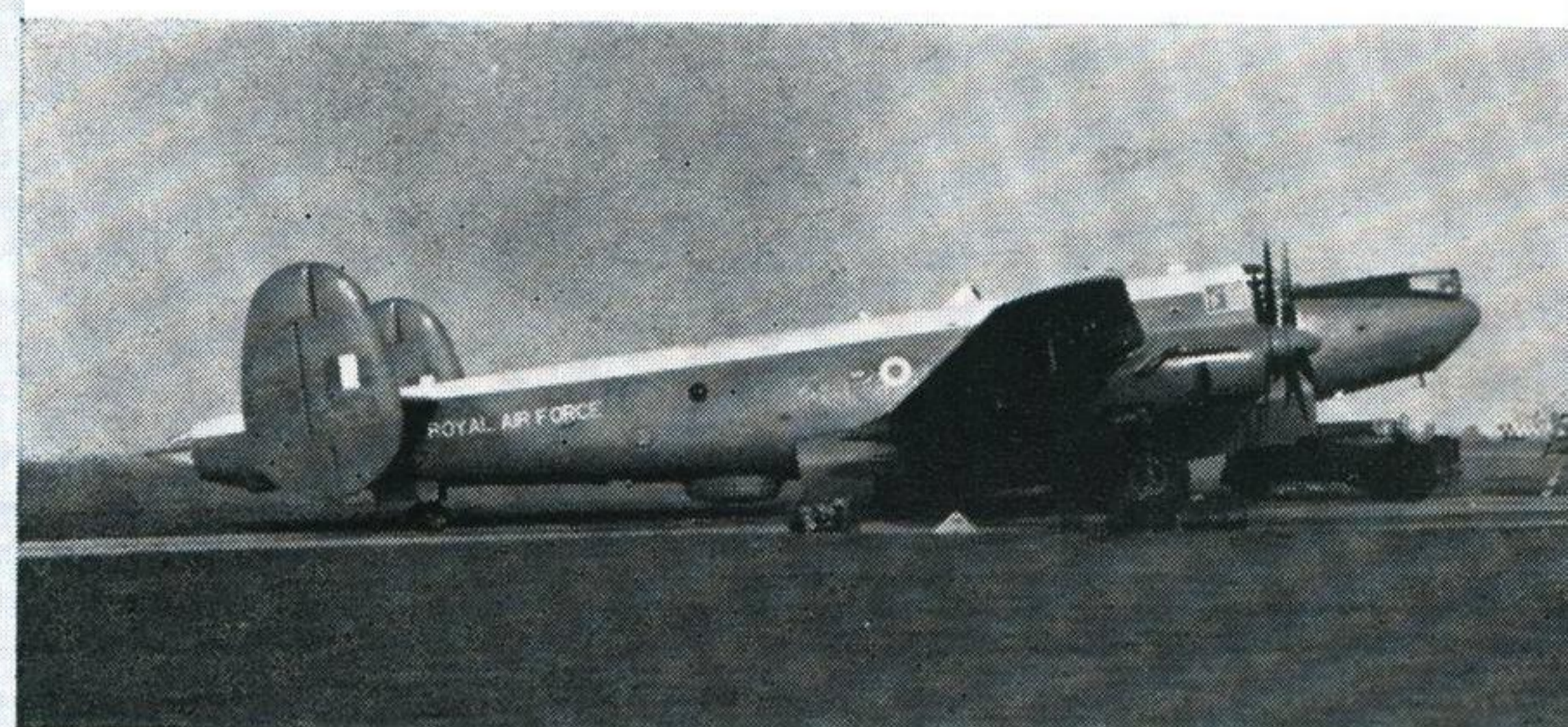
SHACKLETON M.R.2 Developed version of M.R.1 with streamlined nose and faired transparent tail cone, and with nose radome equipment of M.R.1 housed in retractable ventral radome. Span 120 feet
