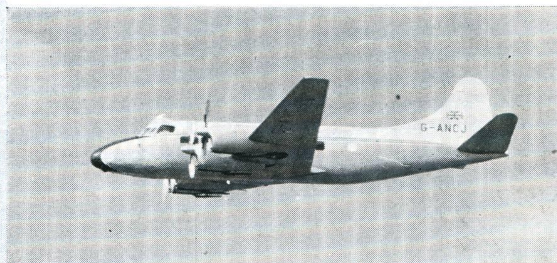
HERON Basically a scaled-up Dove, the Heron is in civil and military use in some 30 countries. Span 71 feet
