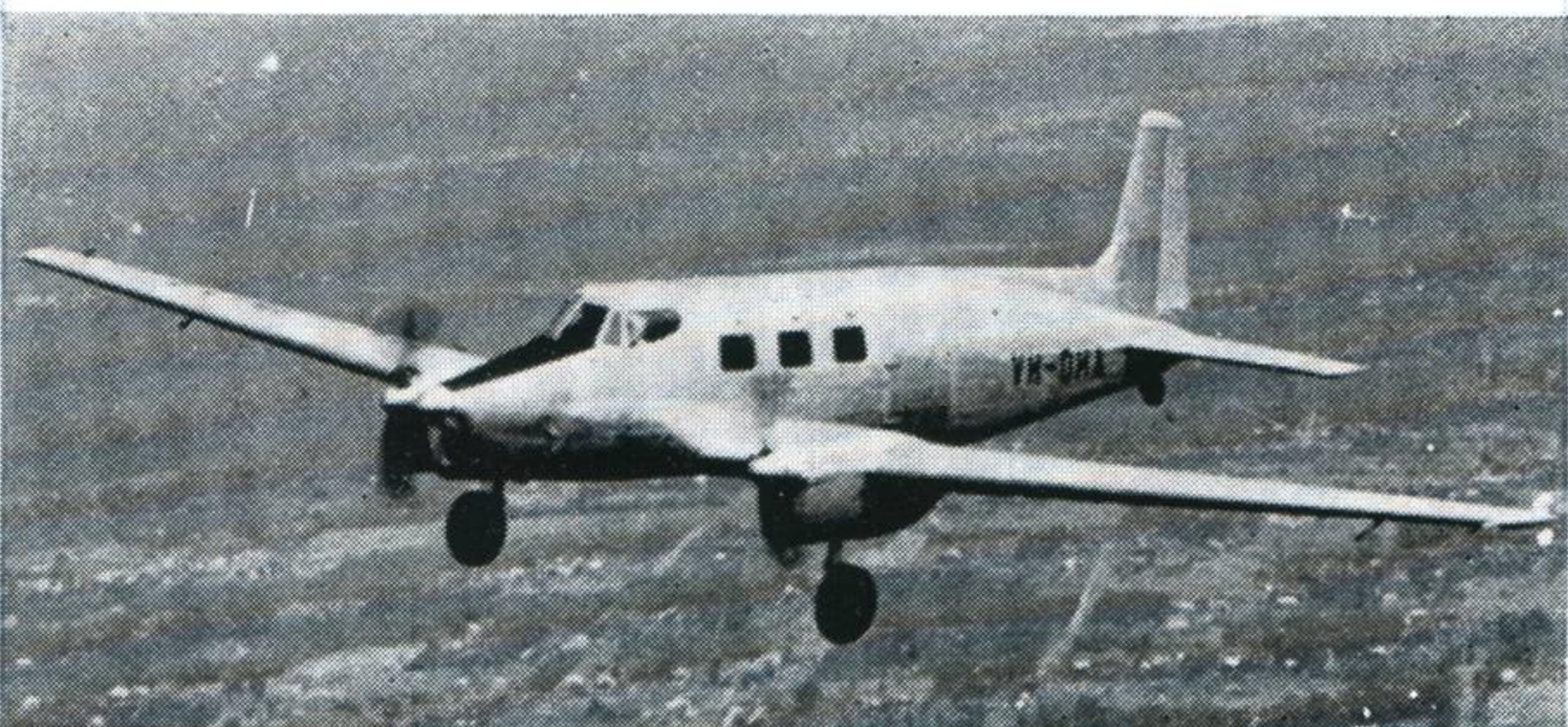
DROVER Basically a three-engined Dove, the Drover was built by De Havilland of Australia in which Commonwealth it is still operated. Span 57 feet
