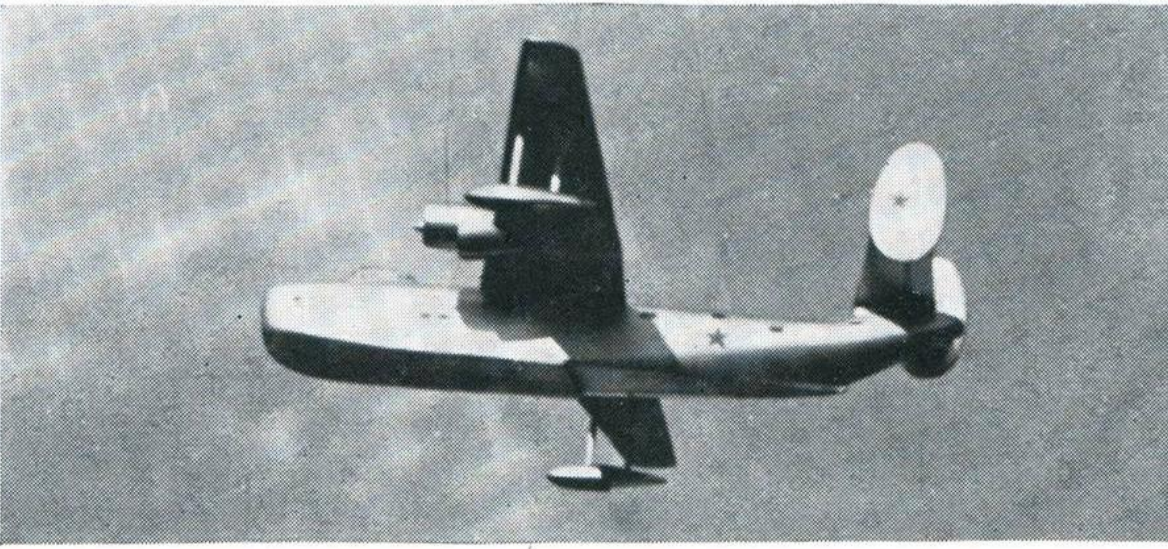
MADGE Long-range reconnaissance flying boat for the Russian fleet, the Madge may be seen with radome extended beneath the hull, or with extended "sting" tail. Span 108 feet
