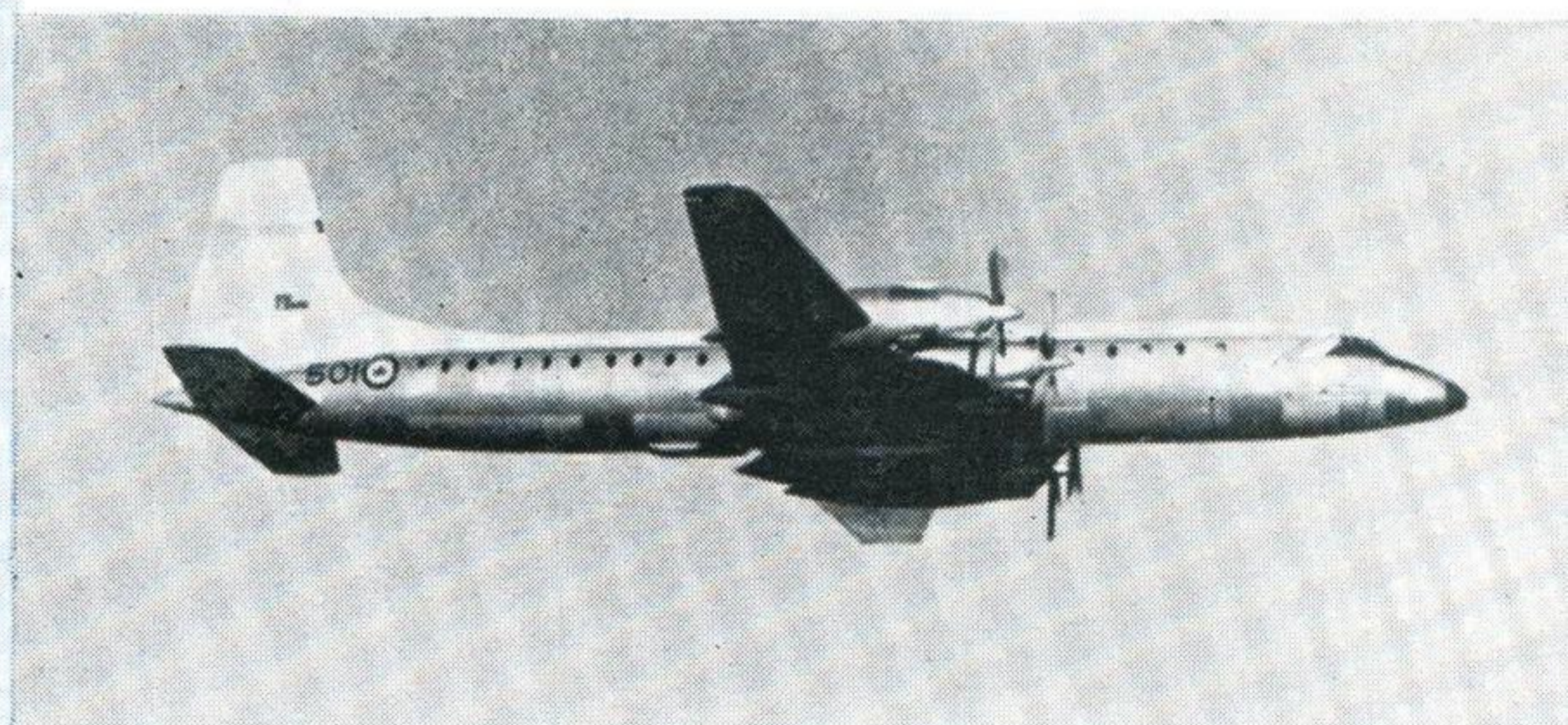
YUKON A "stretched fuselage" version of the Britannia used by the R.C.A.F. and built by Canadair. A civil version, the Canadair CL-44D, has a hinged rear fuselage to facilitate loading. Span 142 feet
