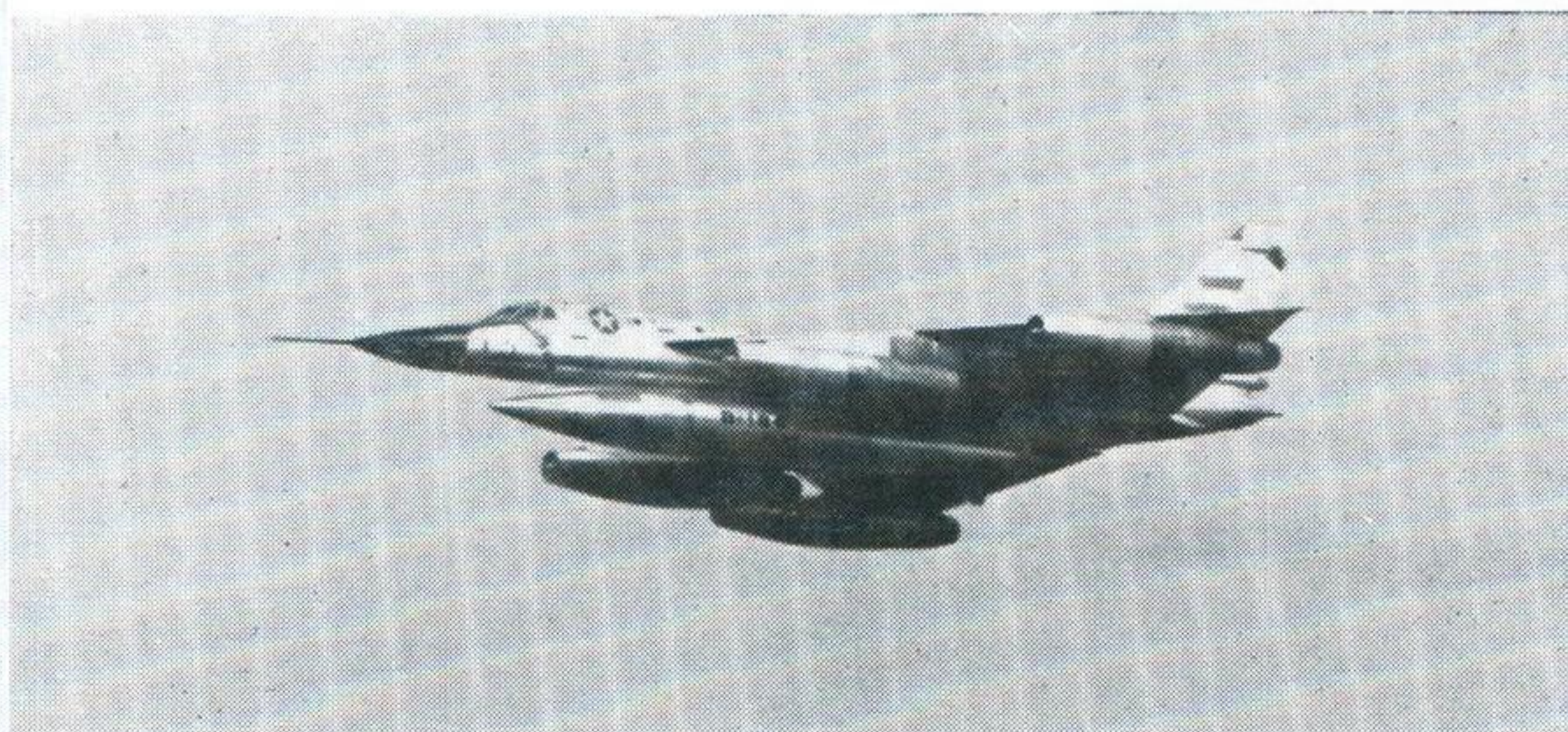
HUSTLER A long-range medium bomber in U.S.A.F. service is their B-58A. Eight have been converted to TB-58A dual control trainers with revised canopy. Span 57 feet
