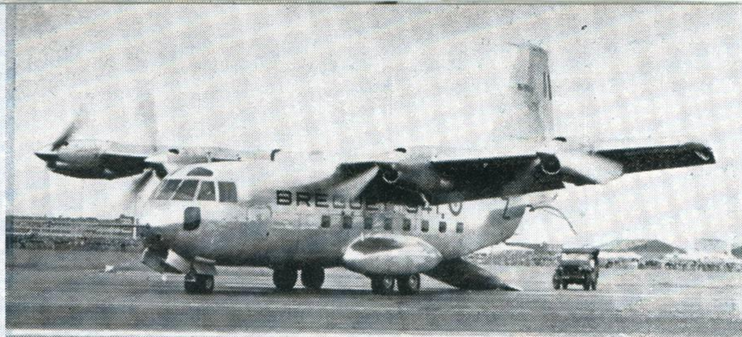
BREGUET 941 Prototype of a STOL tactical transport now in production, this French aircraft can accommodate up to sixty troops or alternatively vehicles, including some A.F.V. types. Span 77 feet
