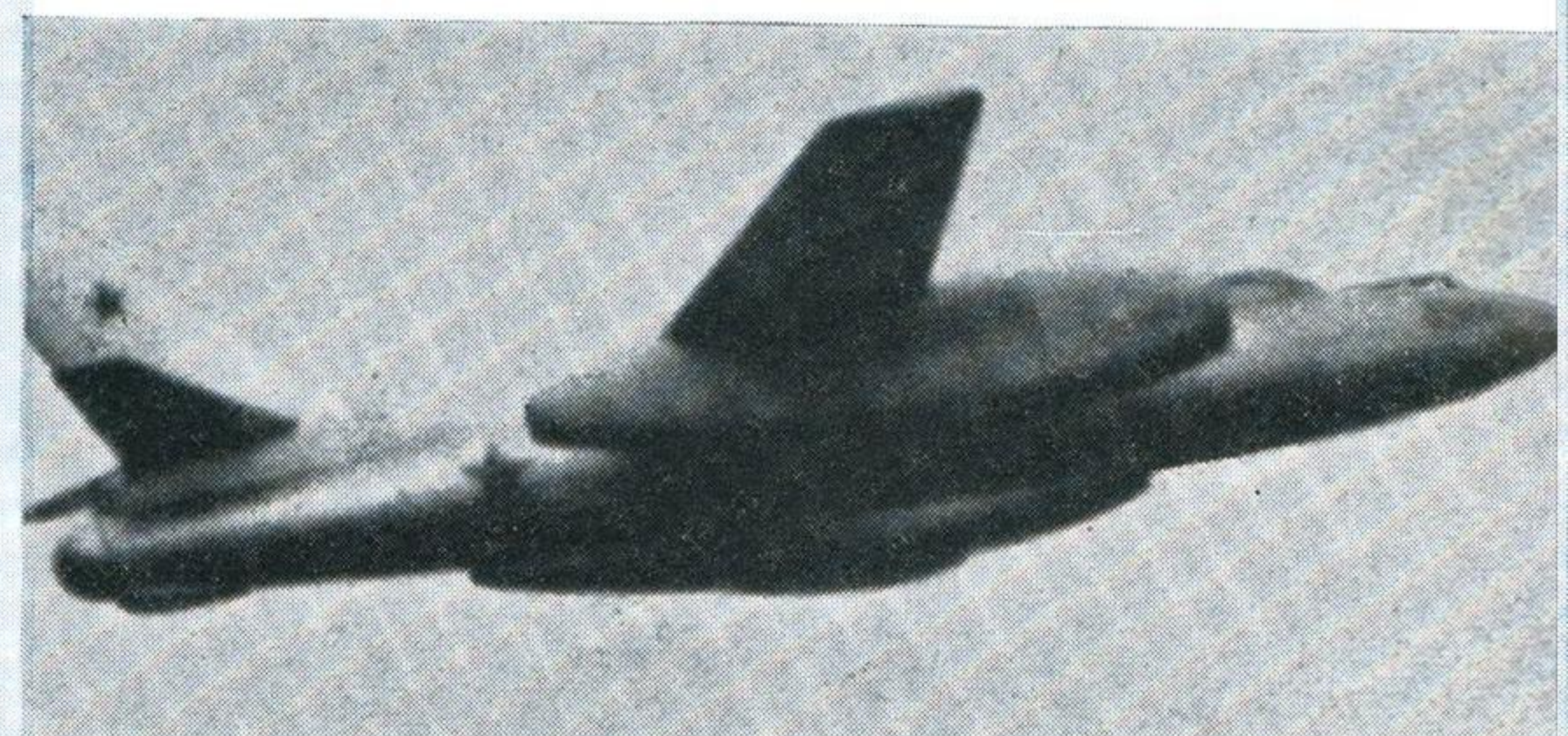
MASCOT Trainer version of the Beagle with revised nose section designated Il-28U. In service in Communist Bloc countries using the Beagle. Span 64 feet
