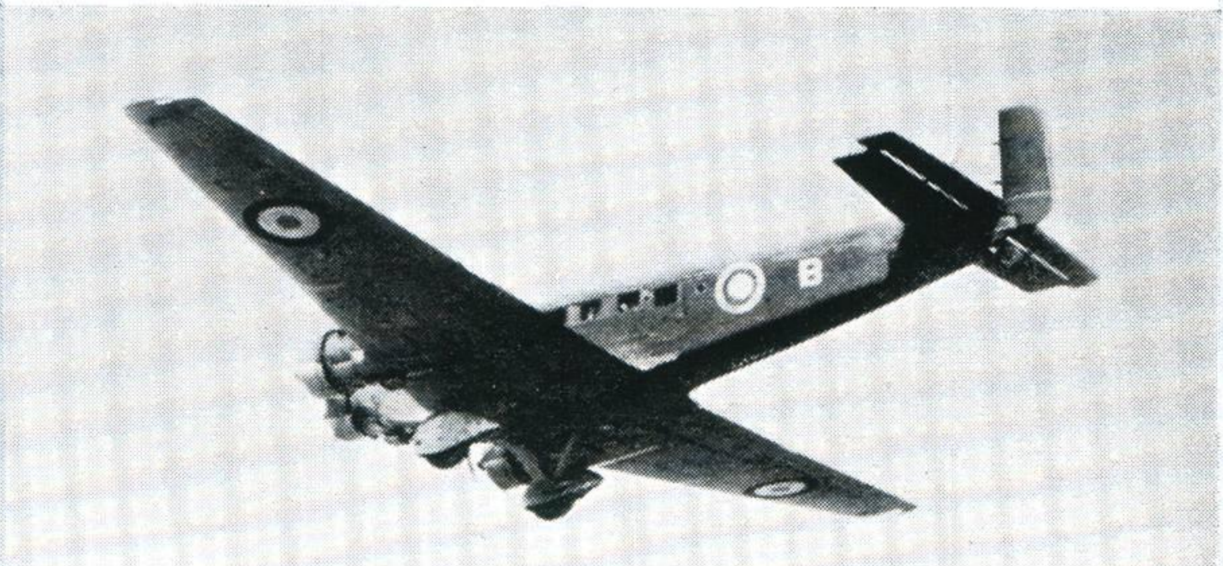
JUNKERS Ju 52/3M Pre-war and wartime troop transport of Germany, the Ju 52/3m is still in limited military use by several countries. The 3m denotes three engines. Span 100 feet
