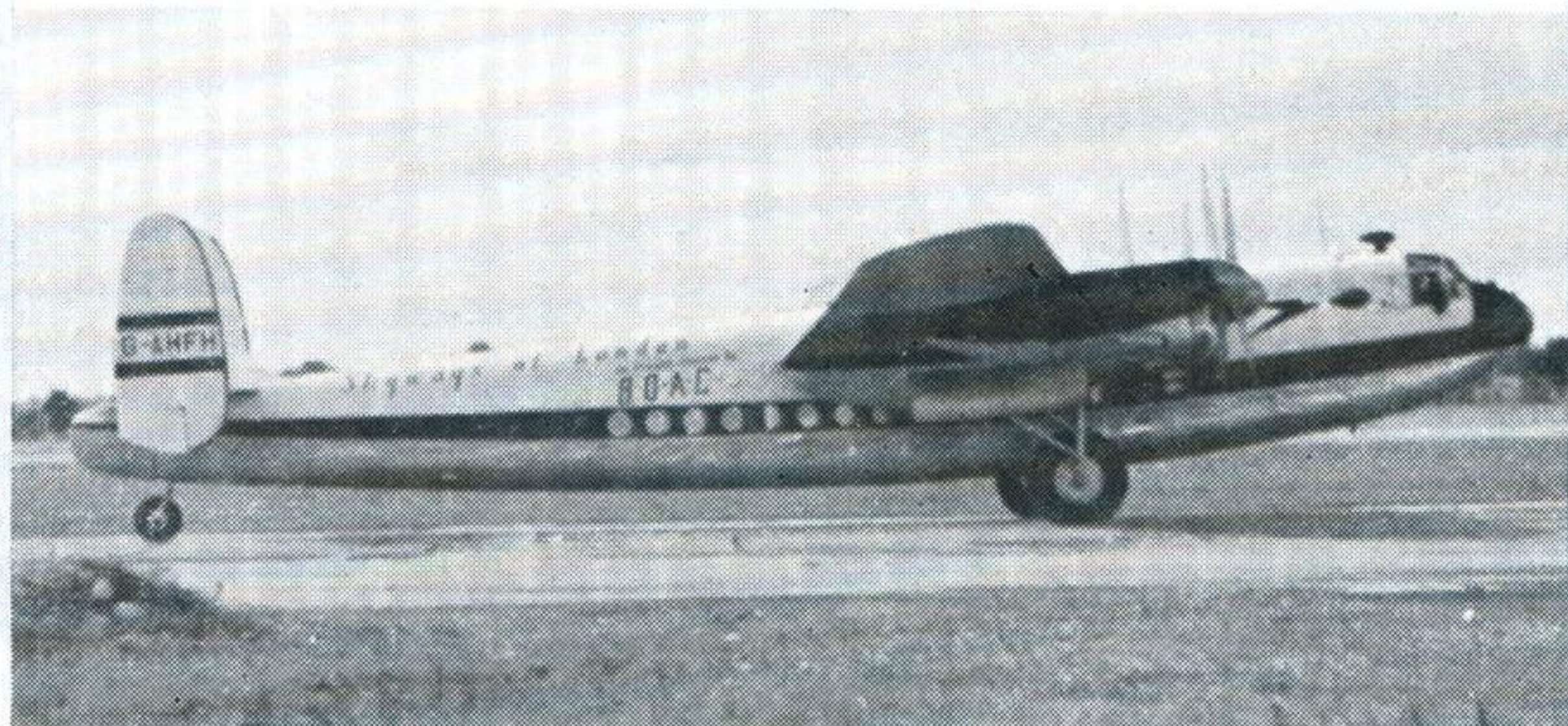
YORK This wartime transport, utilising a standard Lancaster wing form and undercarriage, is still in limited use overseas. Span 102 feet
