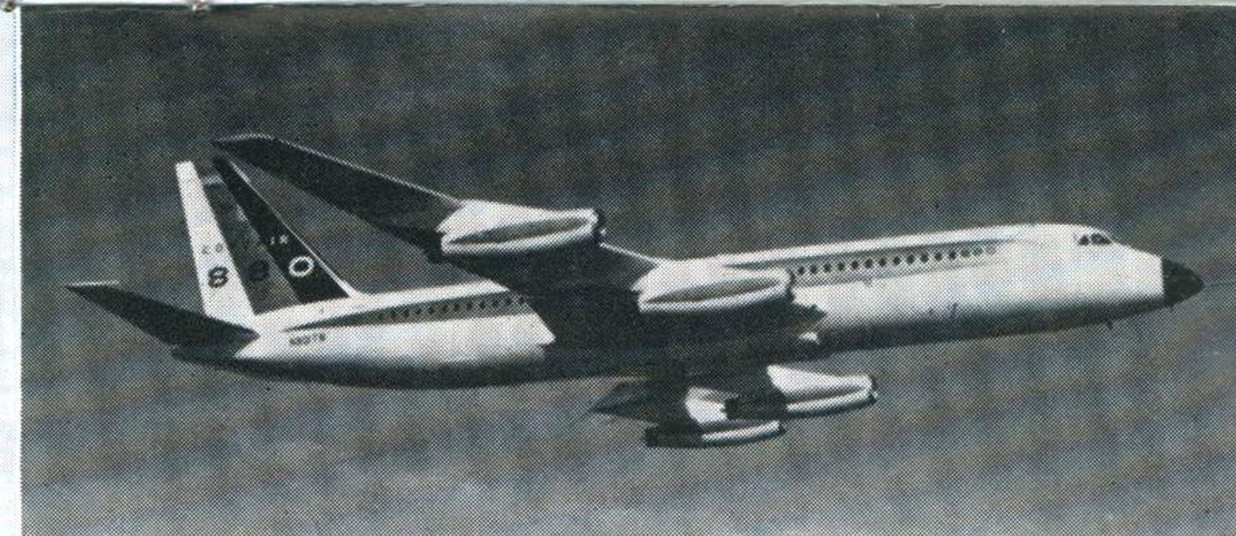
CONVAIR 880 This medium American airliner is used by several airlines world-wide and is produced in the 880 and 880-M versions with variations mainly in detail items. Span 120 feet
