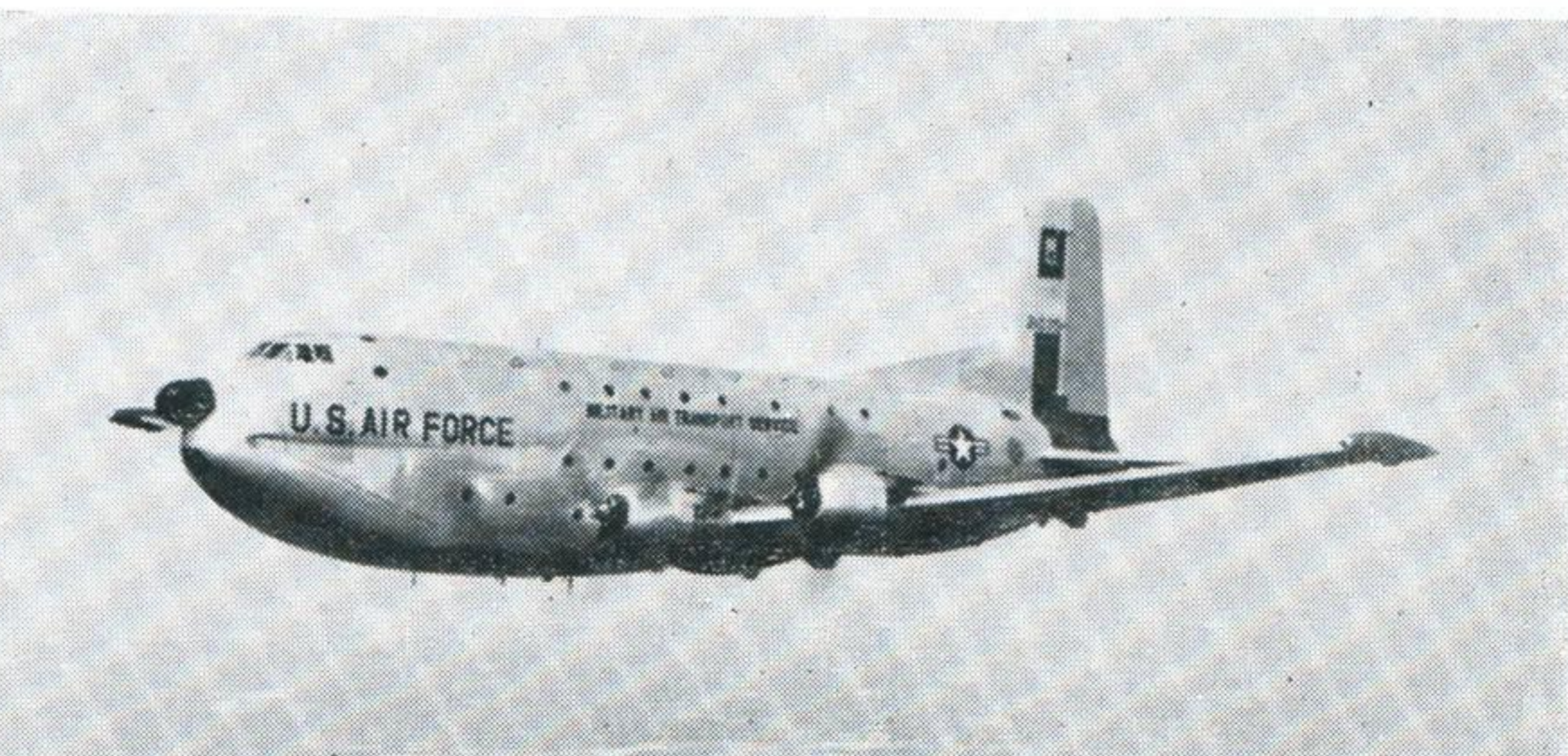
GLOBEMASTER II A U.S.A.F. transport the Globemaster II went into service in two versions, C-124A and C-124C, but the bulk are now to the C-124C standard depicted. Span 174 feet
