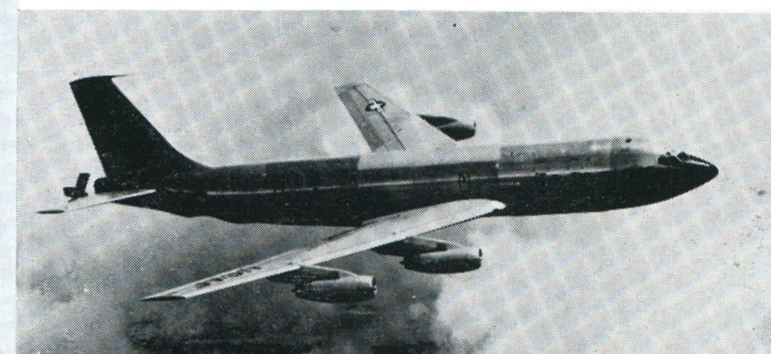
STRATOTANKER From the basic Boeing 707 airliner design, the KC-135A serves the U.S.A.F. as a tanker or long-range transport. Several hundreds are in service. Span 131 feet
