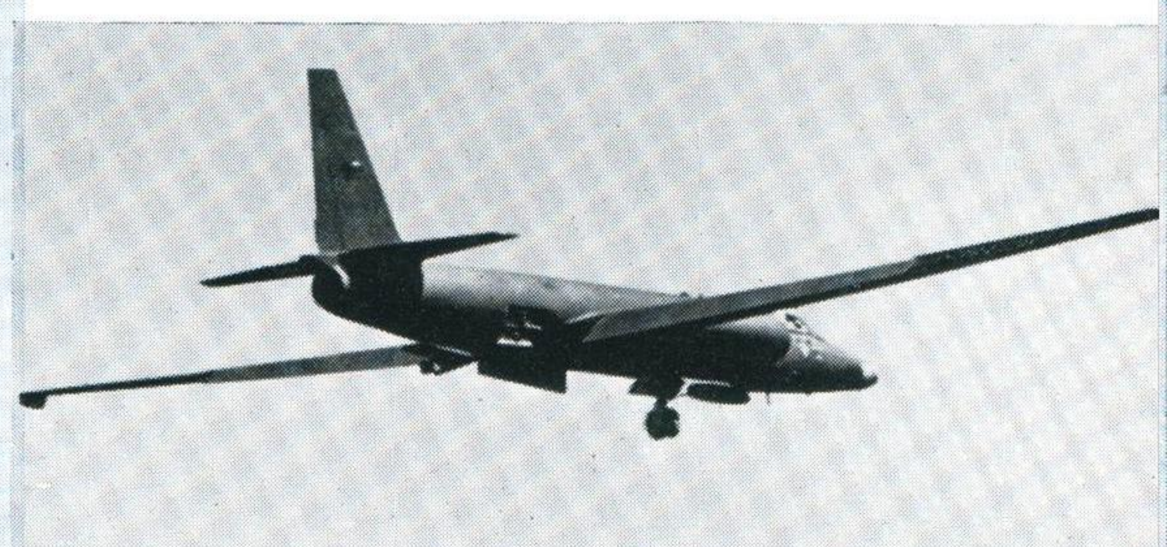
LOCKHEED U-2 Reconnaissance aircraft of unorthodox design, produced in several versions to the same basic configuration. Span 80 feet
