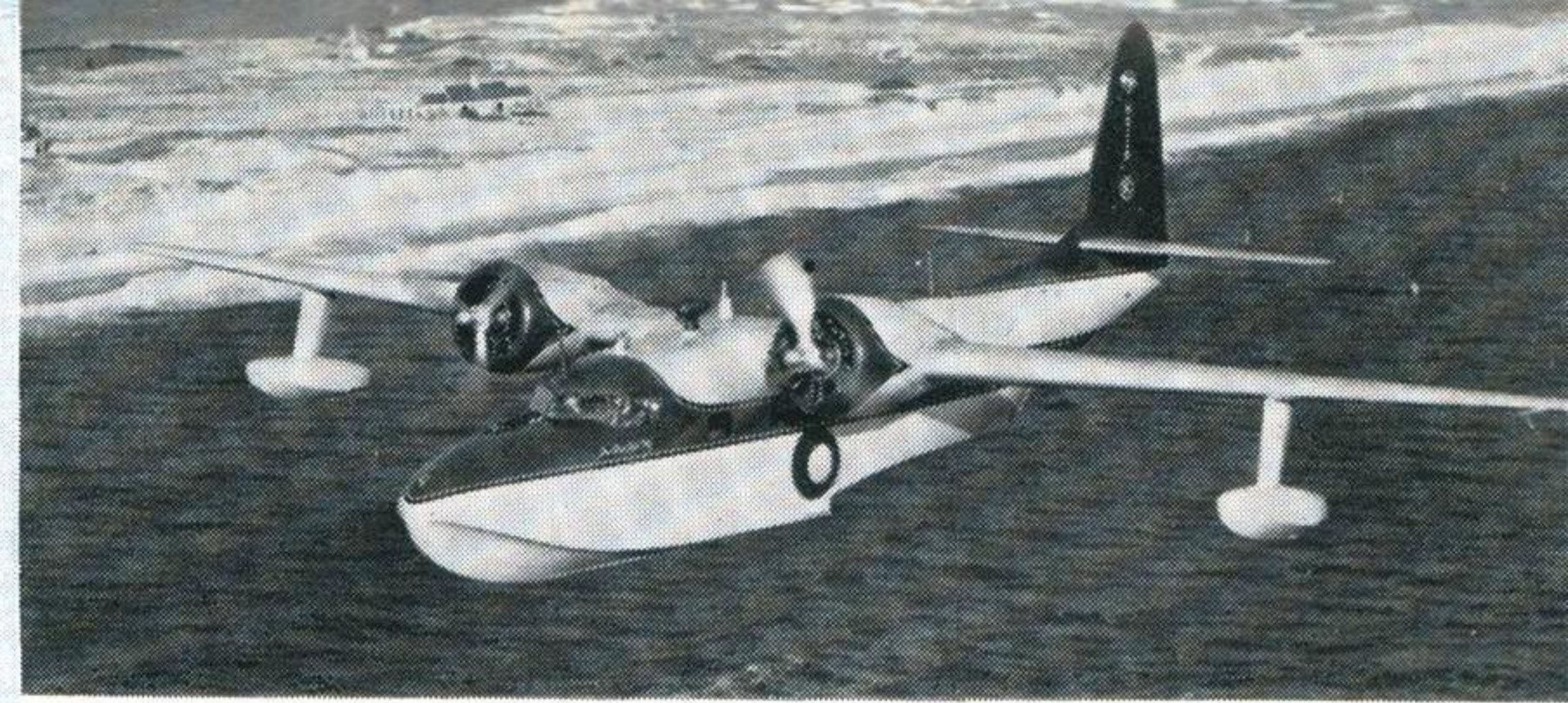
MALLARD Post-war executive amphibian by Grumman, the Mallard is used mainly in the U.S.A. and Canada. Span 67 feet
