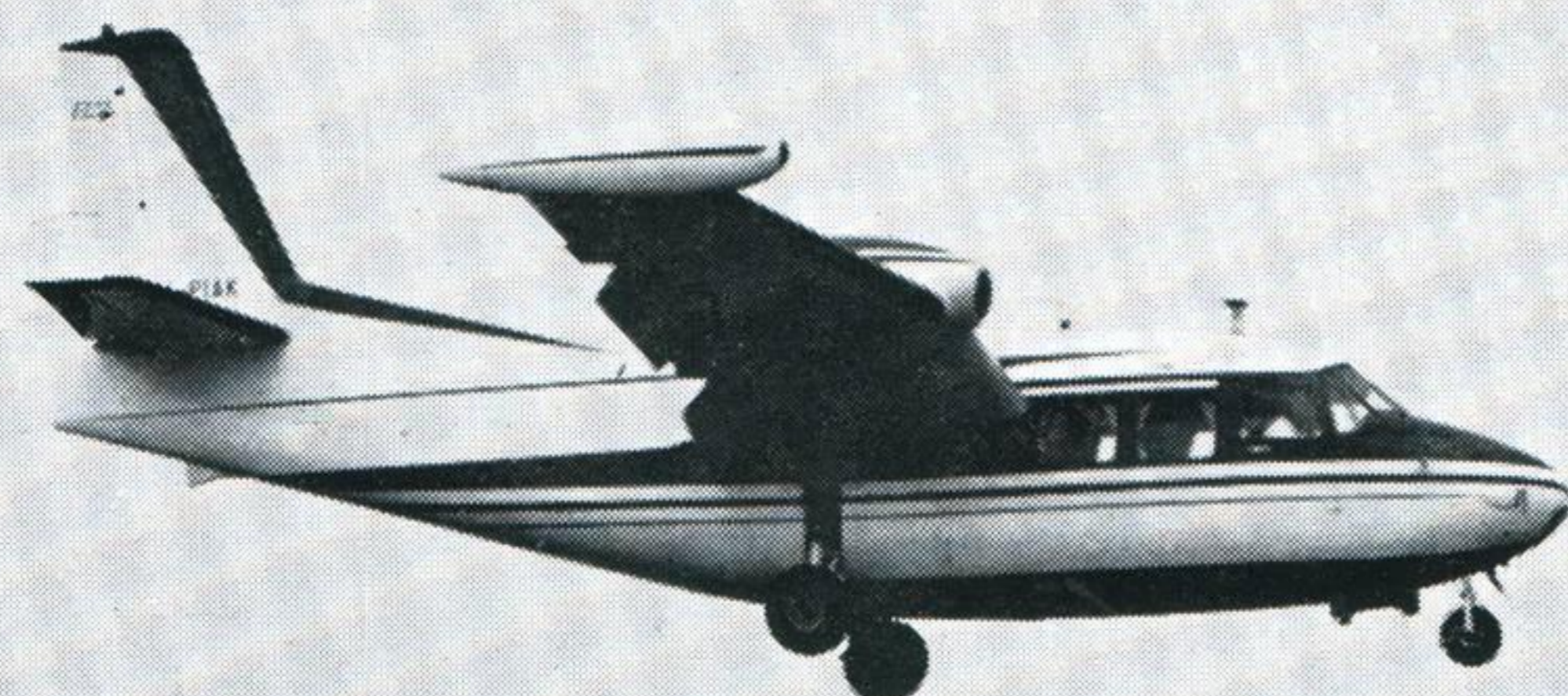
PIAGGIO P.166 An Italian-built military transport (P.166M) and civil transport (P.166B Portofino); the latter version has a re-designed cabin with a lengthened nose. Span 47 feet
