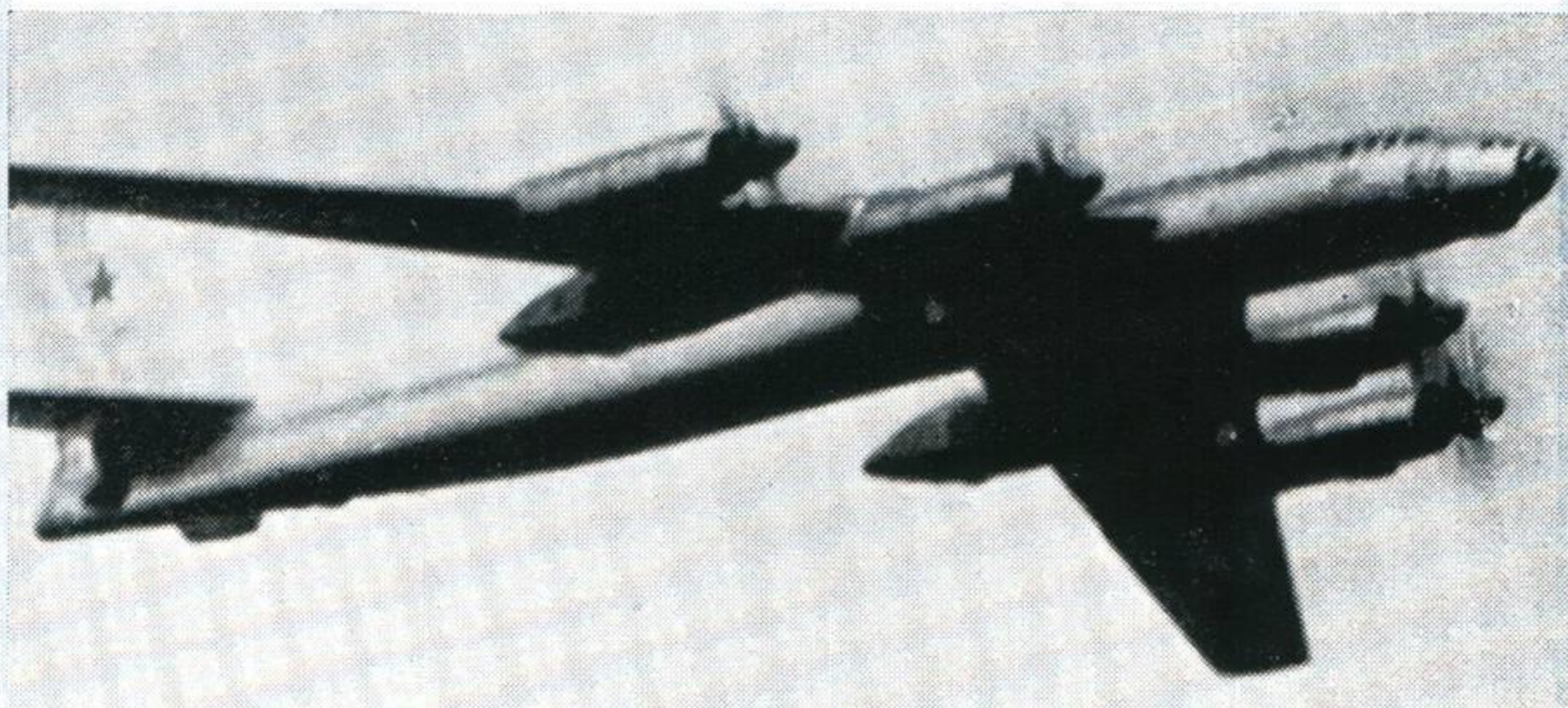
BEAR A and B This Russian Tu-95 bomber appears in two versions, A as in the photograph and B as in the silhouette view. The B version may carry an under-fuselage missile. Span 167 feet
