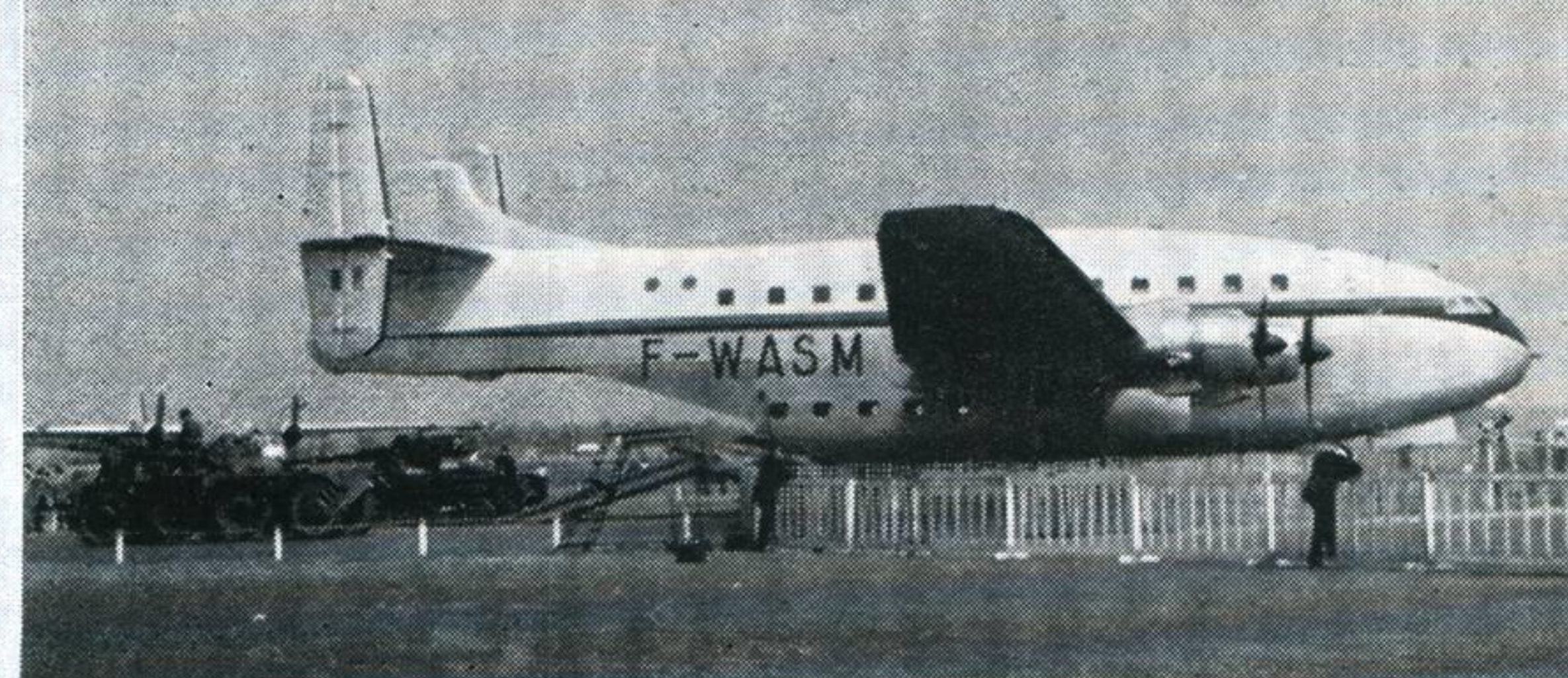
SAHARA The Breguet 765 transport, used by the French Army, can accommodate up to 146 troops or alternatively an AMX tank. Span 141 feet
