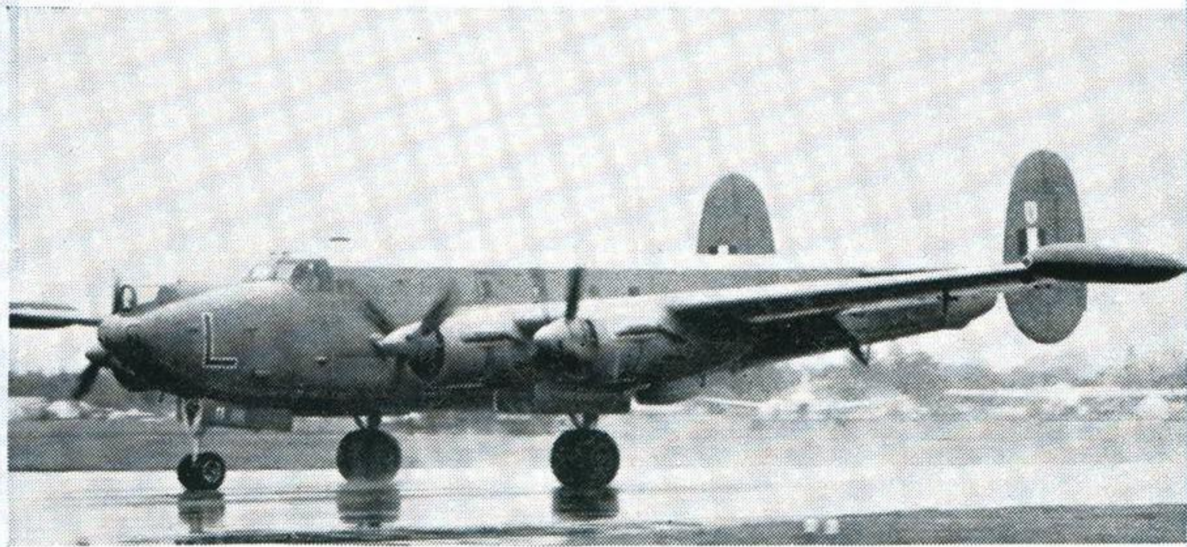
SHACKLETON M.R.3 Final production version of the Shackleton with tricycle undercarriage and wingtip fuel tanks; in R.A.F. and S.A.A.F. service. Span 120 feet
