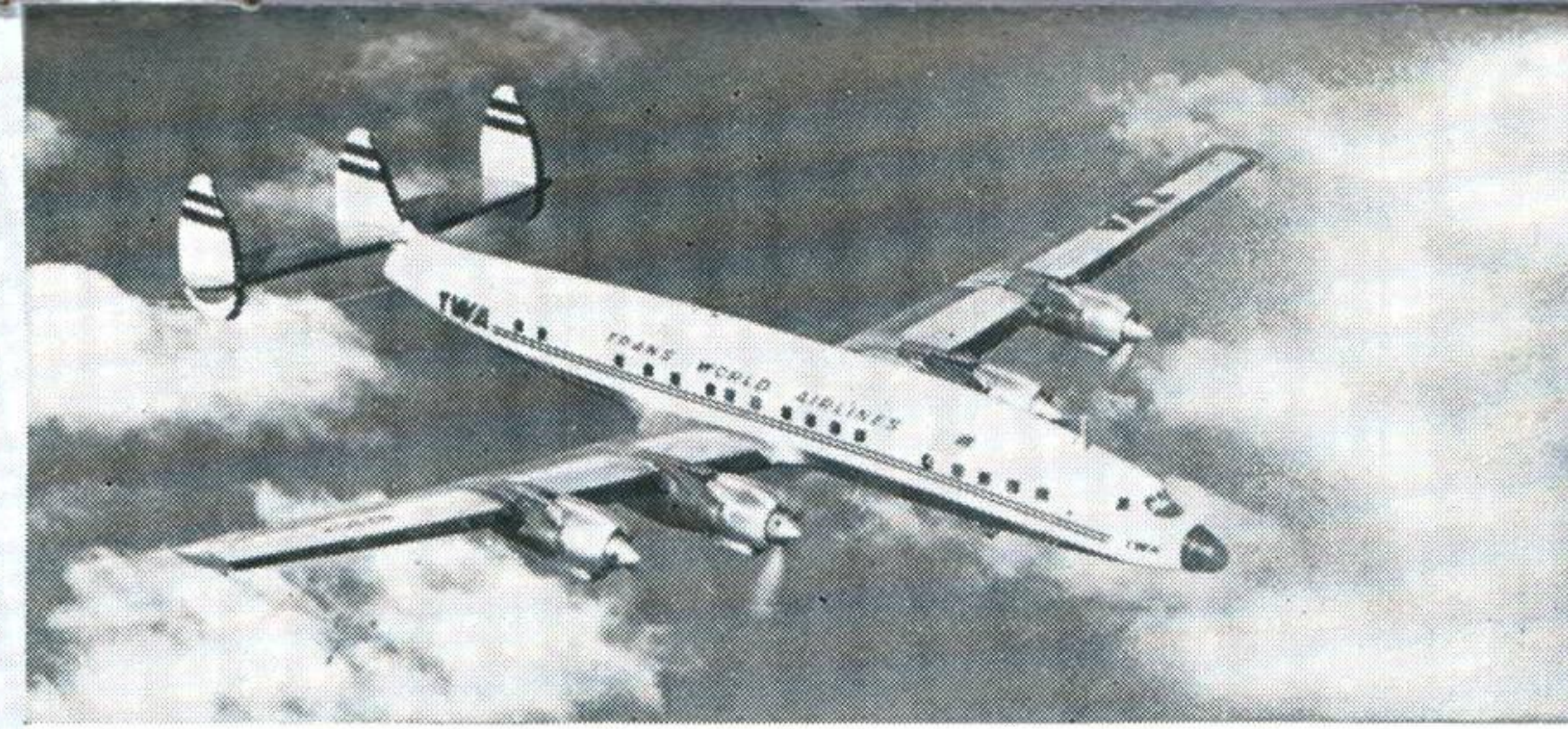
STARLINER Adapted from the Constellation, a limited number of Super Constellations were built with a wing of increased span and differing form. Span 150 feet
