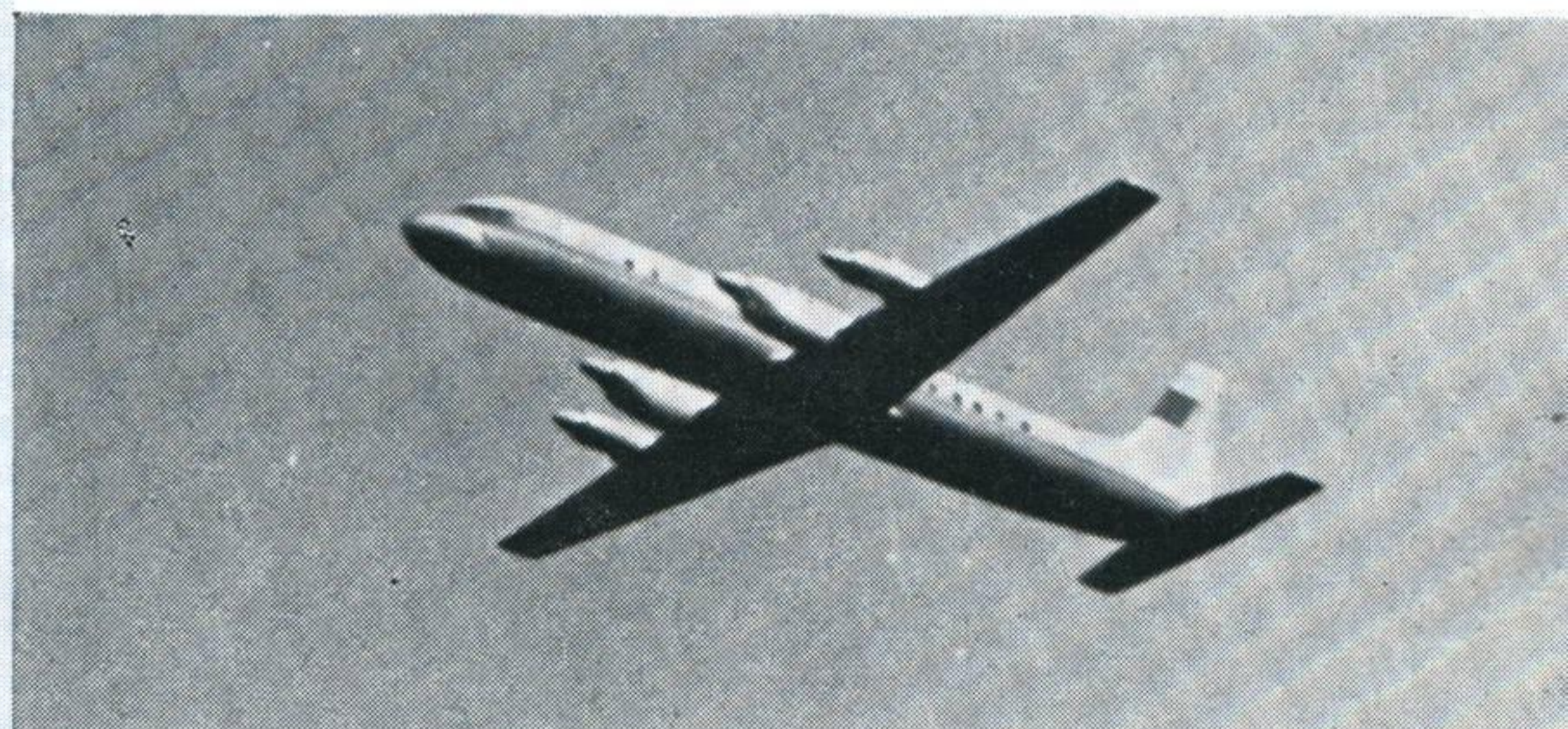
COOT This successful Ilyushin Il-18 airliner, known as the Moskva, is widely used by Aeroflot and is also in use by several airlines in Eastern Europe and in Africa. Span 113 feet
