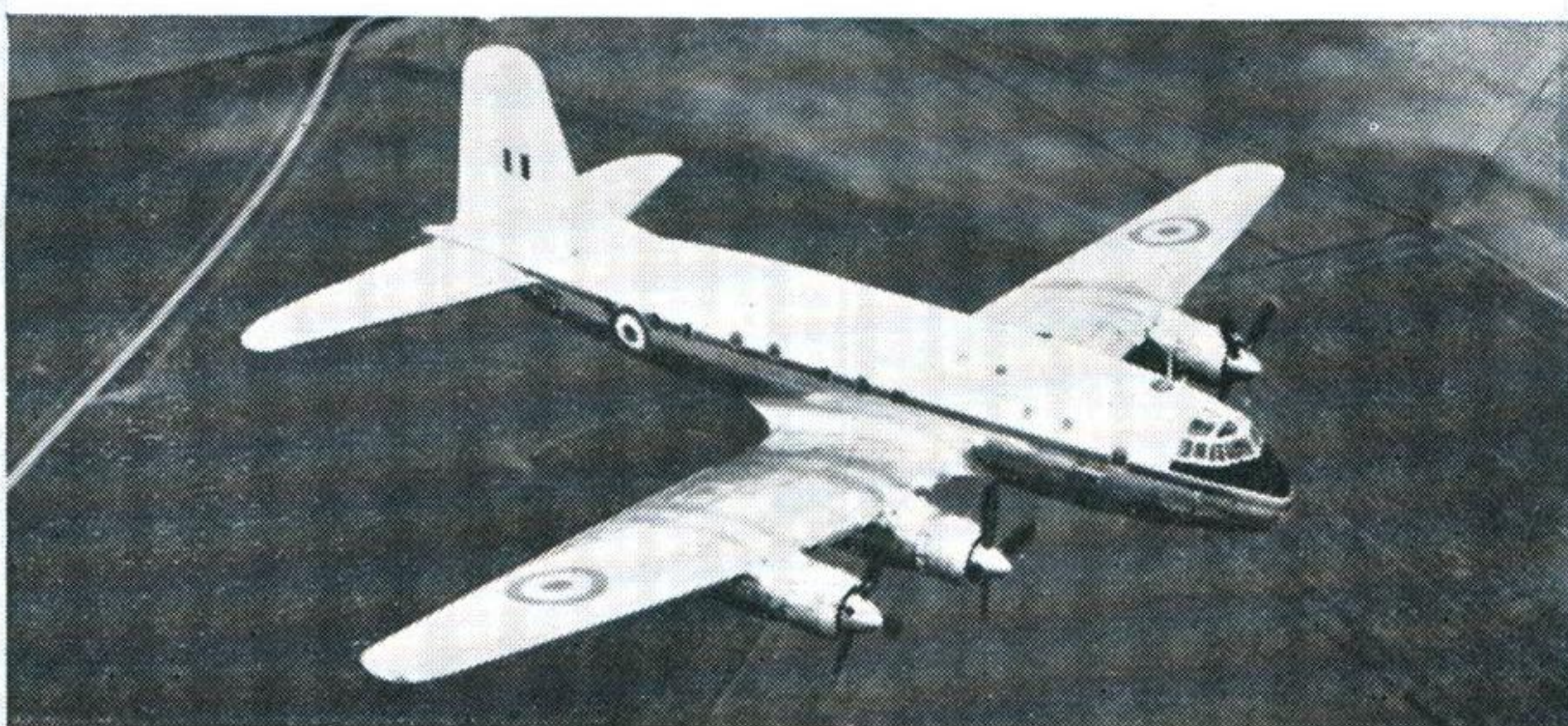
HASTINGS Backbone of R.A.F. Transport Command for many years, the Hastings is still in service. C.1 and C.2 versions vary in the height setting of the tailplane. Span 113 feet
