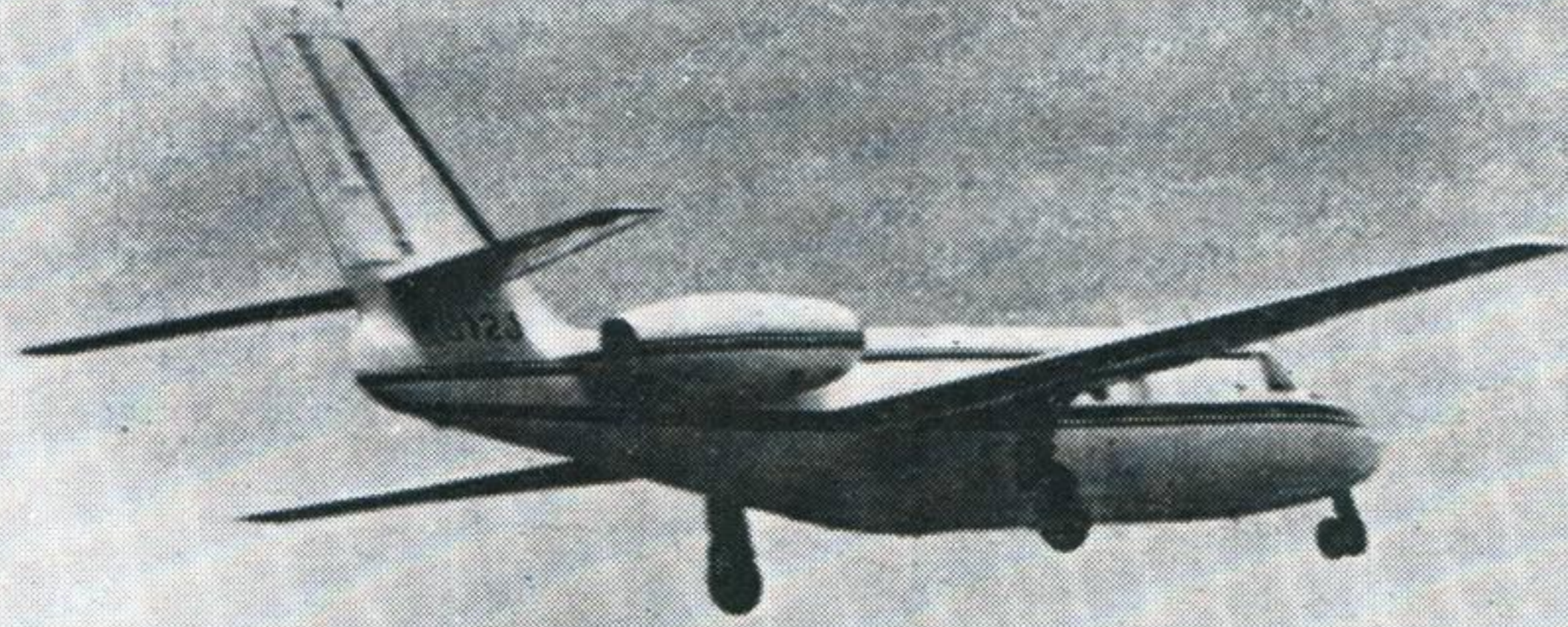
JET COMMANDER The production version of the eight-seat Aero Jet Commander will have a 2½ feet fuselage length increase. Span 43 feet
