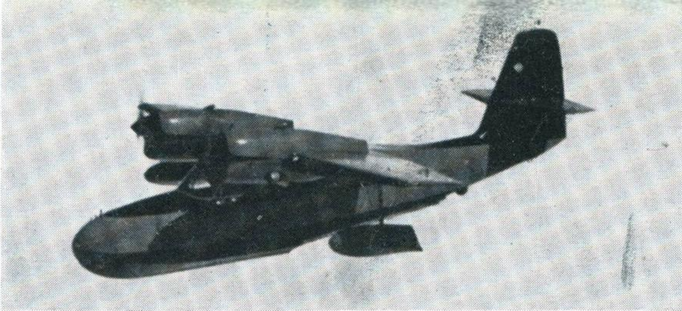
WIDGEON Like the Grumman Goose the Widgeon, by the same firm, was built largely to military orders although designed for a civil market with which it found favour post-war. Span 40 feet
