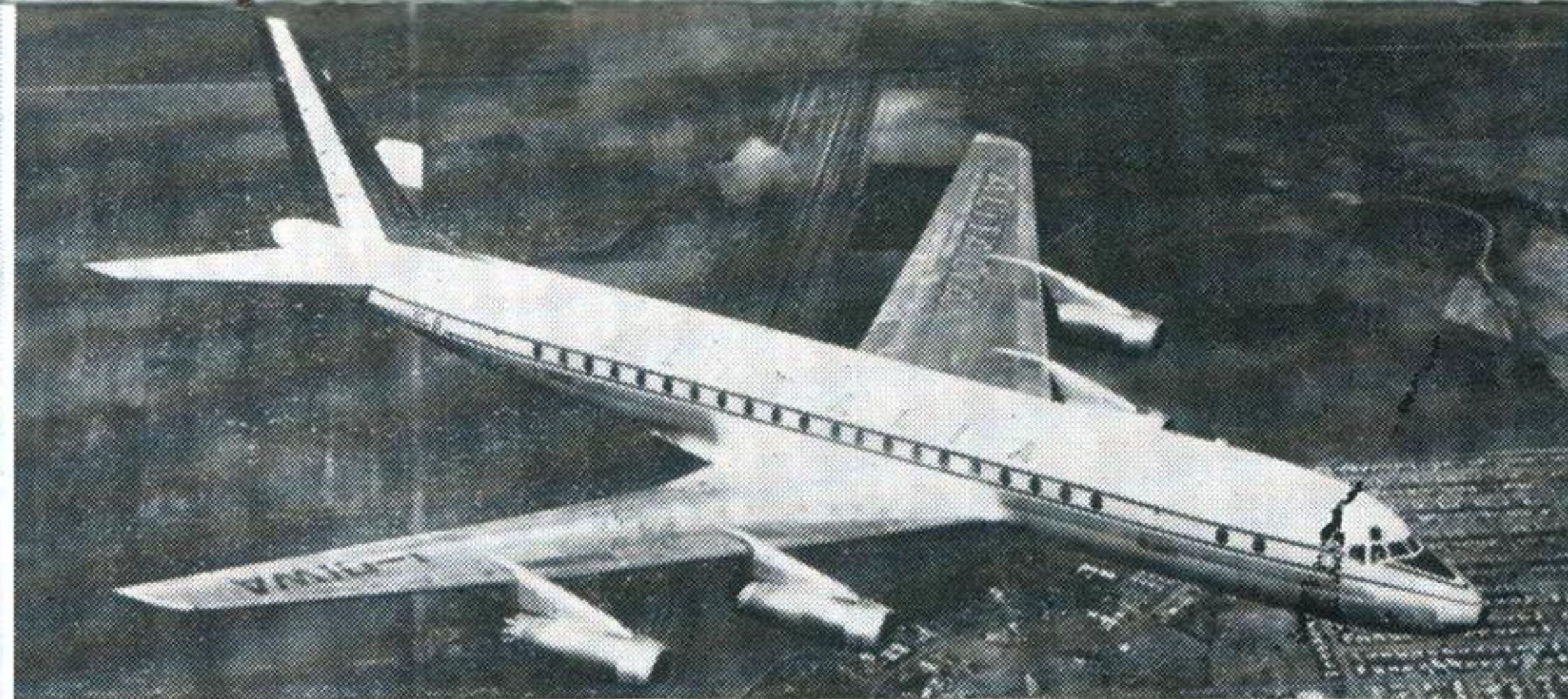
DC-8 Carrying in its several versions up to 173 passengers, the DC-8 series all have the same basic outline which, purely coincidentally, is very similar to the Boeing 707 series. Span 142 feet
