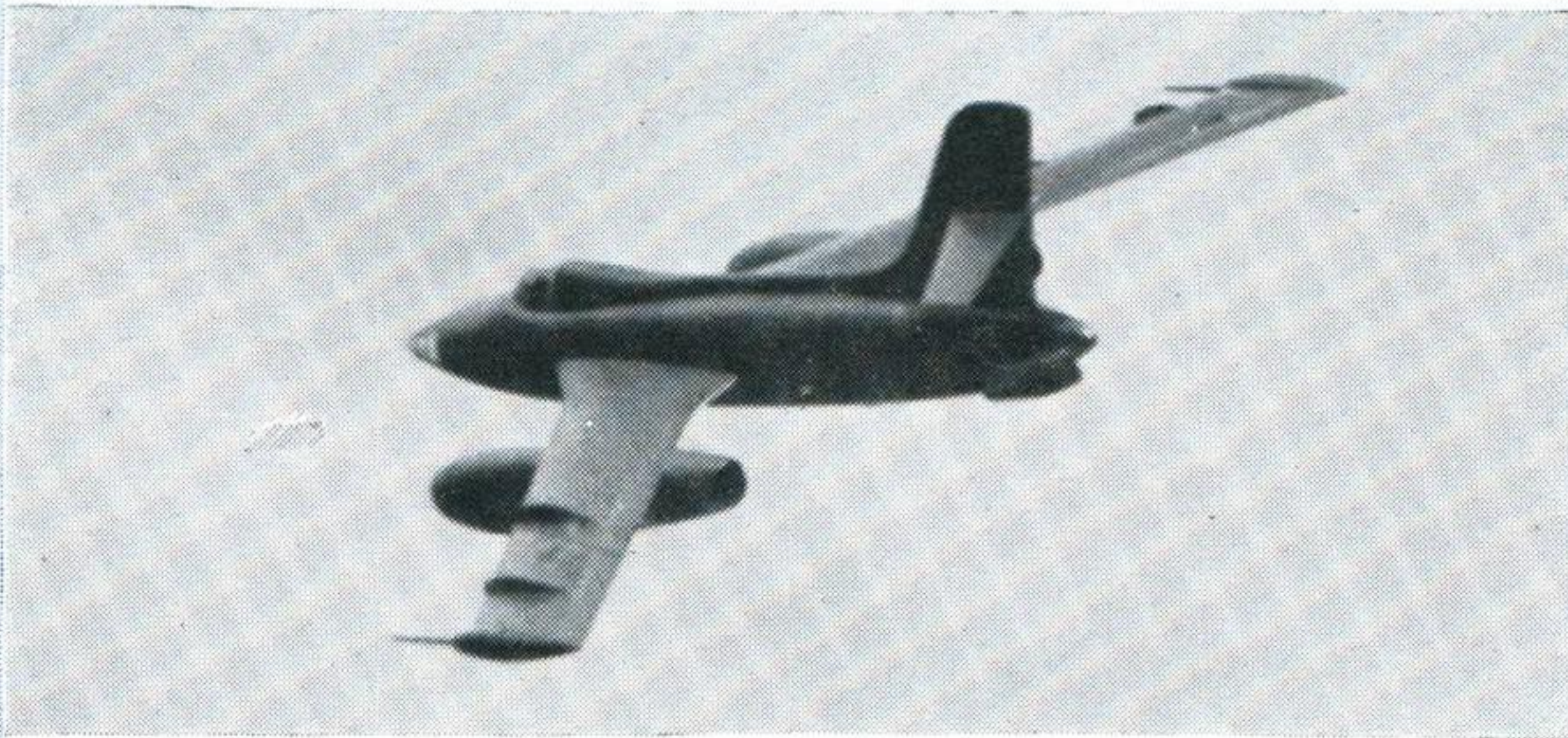
FLASHLIGHT A Russian mid-wing all-weather fighter produced in several versions including a trainer modification named Mangrove. Span 40 feet
