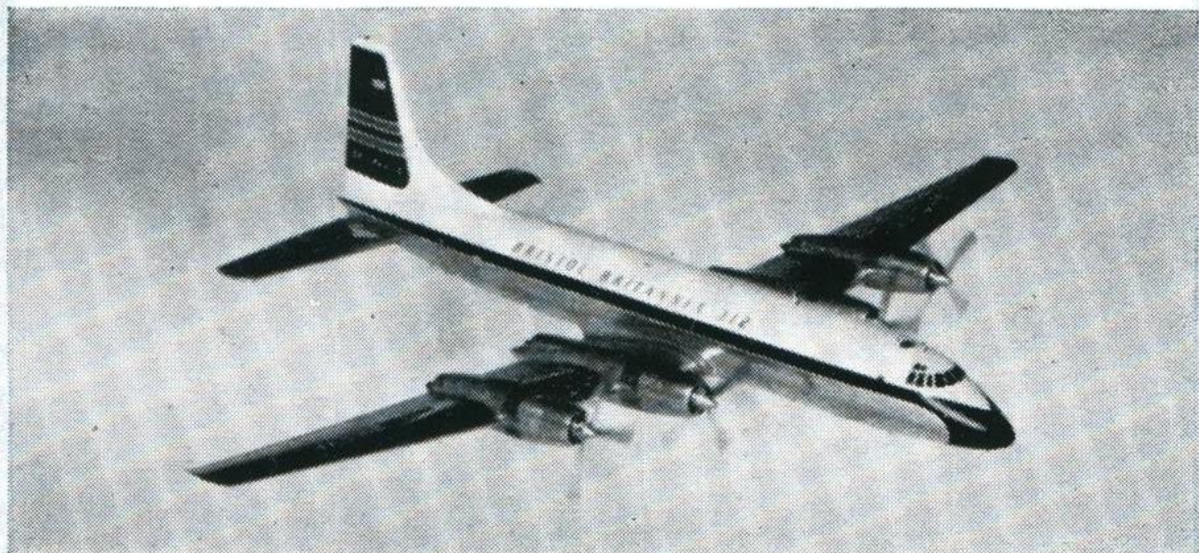
BRITANNIA Produced in different series versions, with main differences in fuselage length, the Britannia is widely used by airlines world-wide and twenty are in R.A.F. use. Span 142 feet
