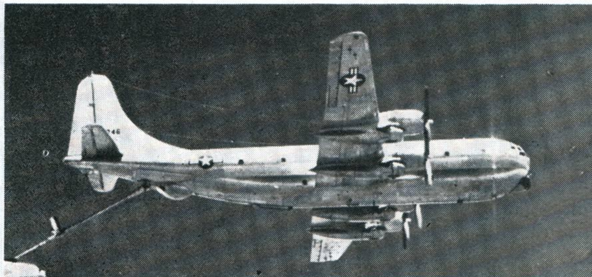
STRATOFREIGHTER Developed as a transport version of the Superfortress, the C-97 Stratofreighter has in later years been used as a tanker/transport and now serves only in reserve units. Span 141 feet
