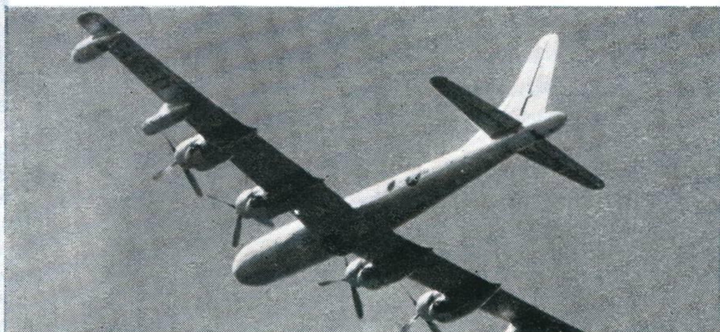
SUPERFORTRESS (B-50) A re-engined version of the B-29, the B-50 series have outlived their prime role, but a few are retained for refuelling, mapping and weather reconnaissance roles. Span 141 feet
