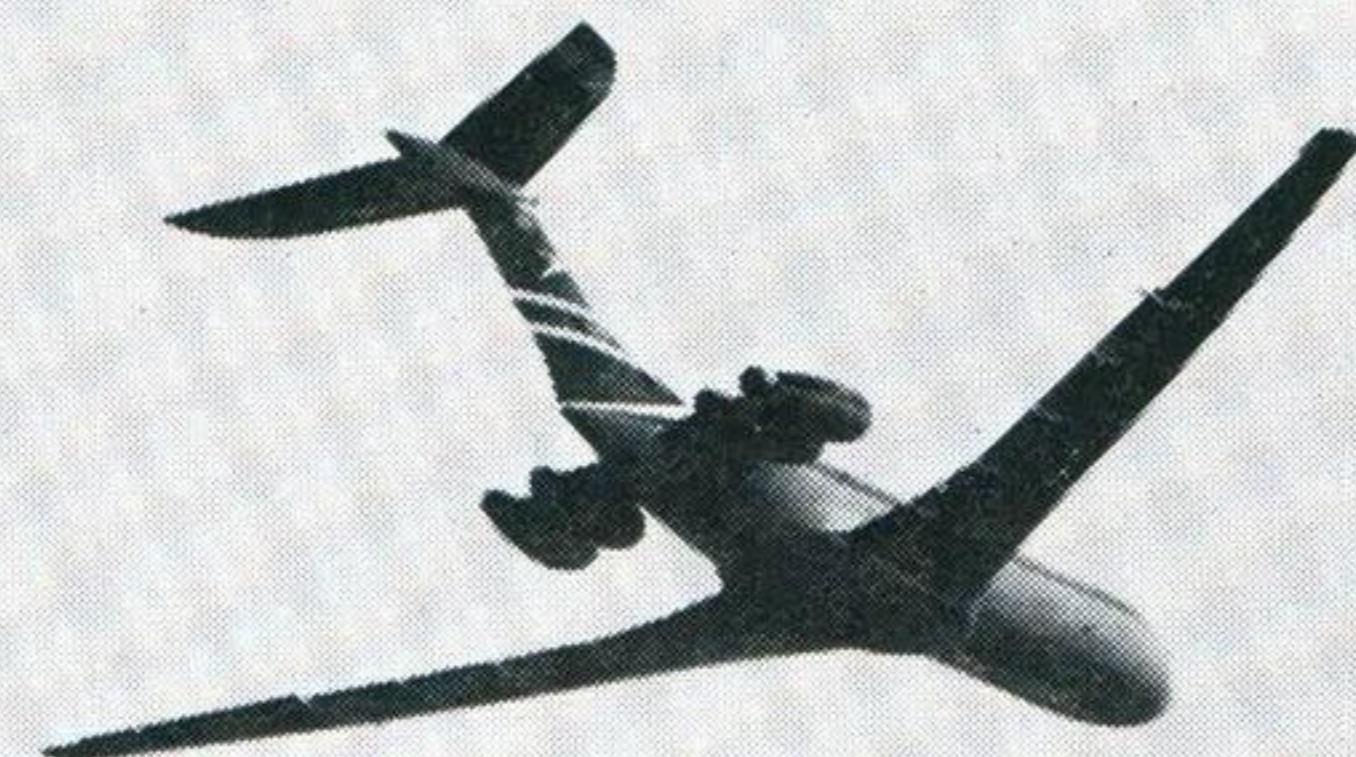
VICKERS VC10 Long range jet airliner ordered for airlines and the R.A.F. Super VC10 with fuselage lengthened by 13 feet now in production. Span 146 feet (VC10) 140 feet (Super VC10)
