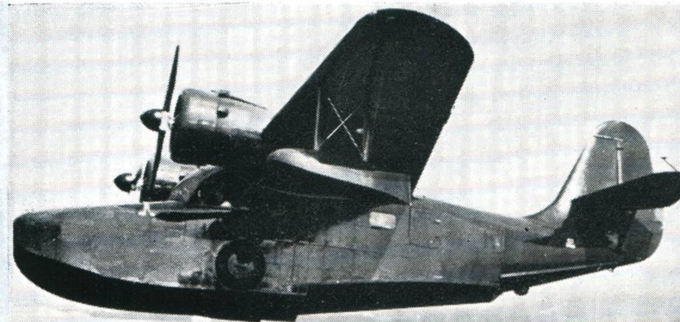
GOOSE A twin-engined amphibian produced mainly to military orders commencing pre-war in the U.S.A., the Goose found a post-war civil market and a number are still in use. Span 49 feet
