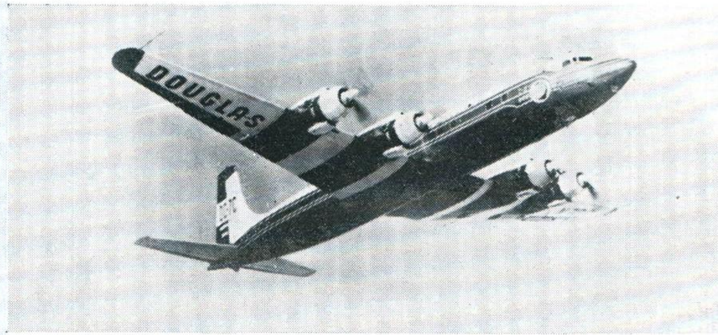
DC-7 A development of the DC-6, the DC-7 has increased span and fuselage length, together with a heightened fin. DC-7B and DC-7C versions have further increases to fuselage lengths and wing-spans. Span 117-127 feet (according to version)
