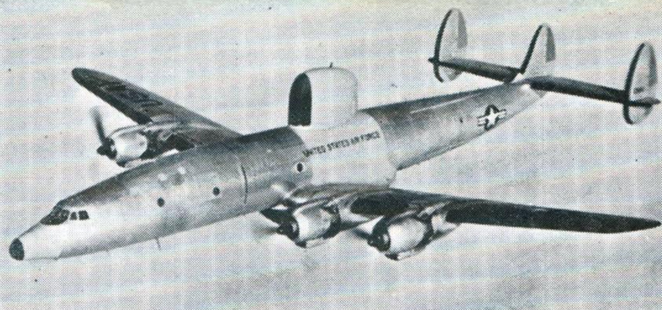
SUPER CONSTELLATION Used by the U.S. Forces as the C-121 Warning Star, the Super Constellation has been adapted for airborne early warning and weather reconnaissance roles. Span 123 feet
