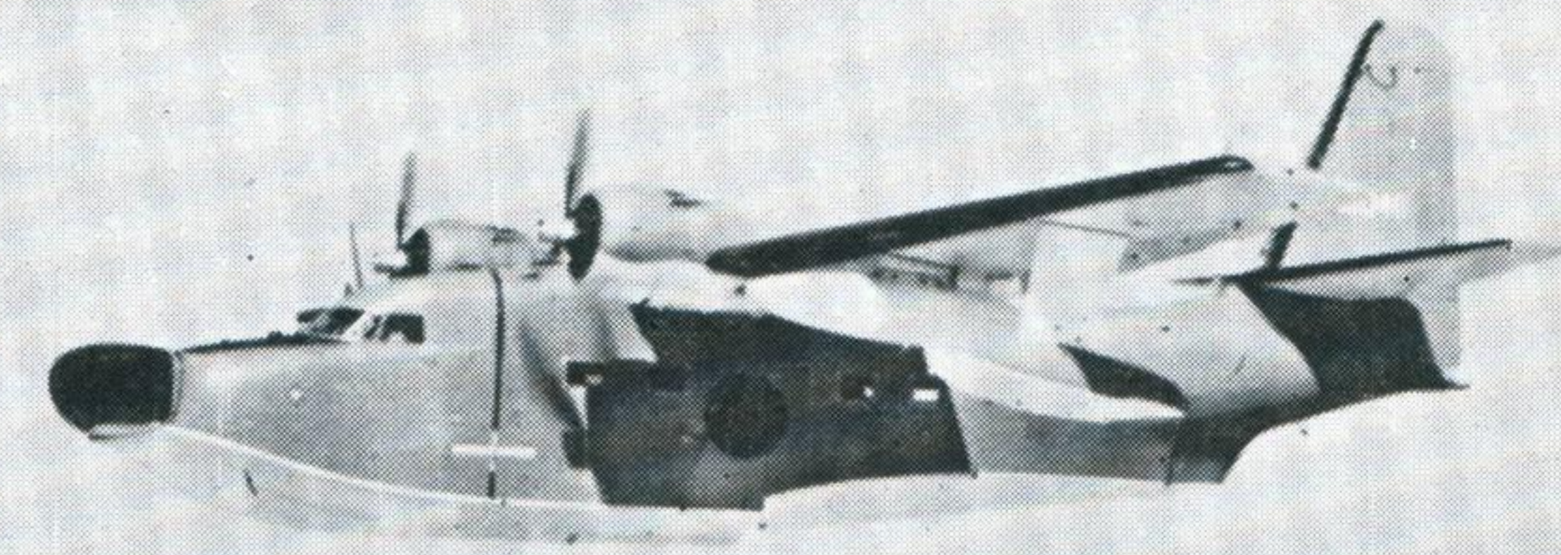
ALBATROSS The several versions of the Albatross in service with various forces vary mainly in span, length, nose radome size and fin and rudder shape. HU-16 in U.S. service. Span 80 and 97 feet
