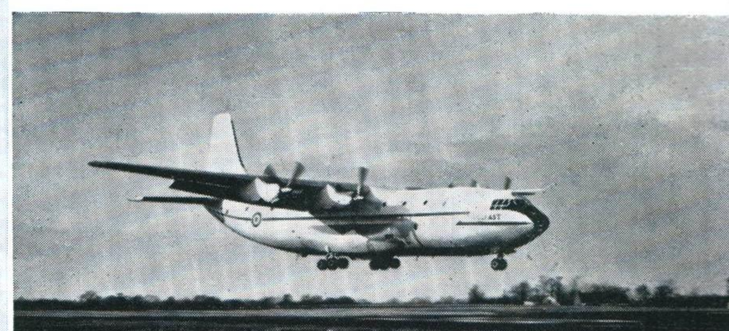
BELFAST R.A.F. Transport Command's latest freighter which is expected in service this year. It can carry several vehicles or helicopters up to a total of 81,000 lb. Span 159 feet
