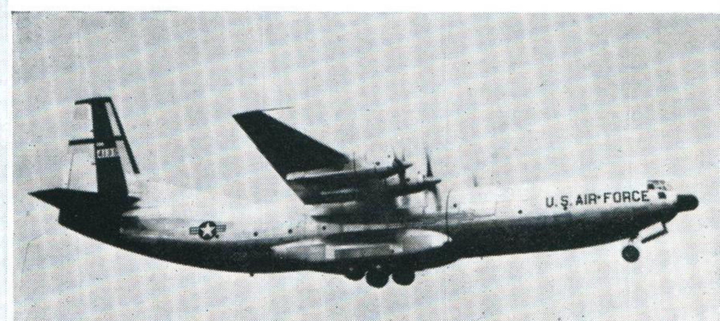
CARGOMASTER The Douglas C-133 Cargomaster, built in C-133A and C-133B versions of similar configuration, is exclusive to the U.S.A.F. Span 180 feet
