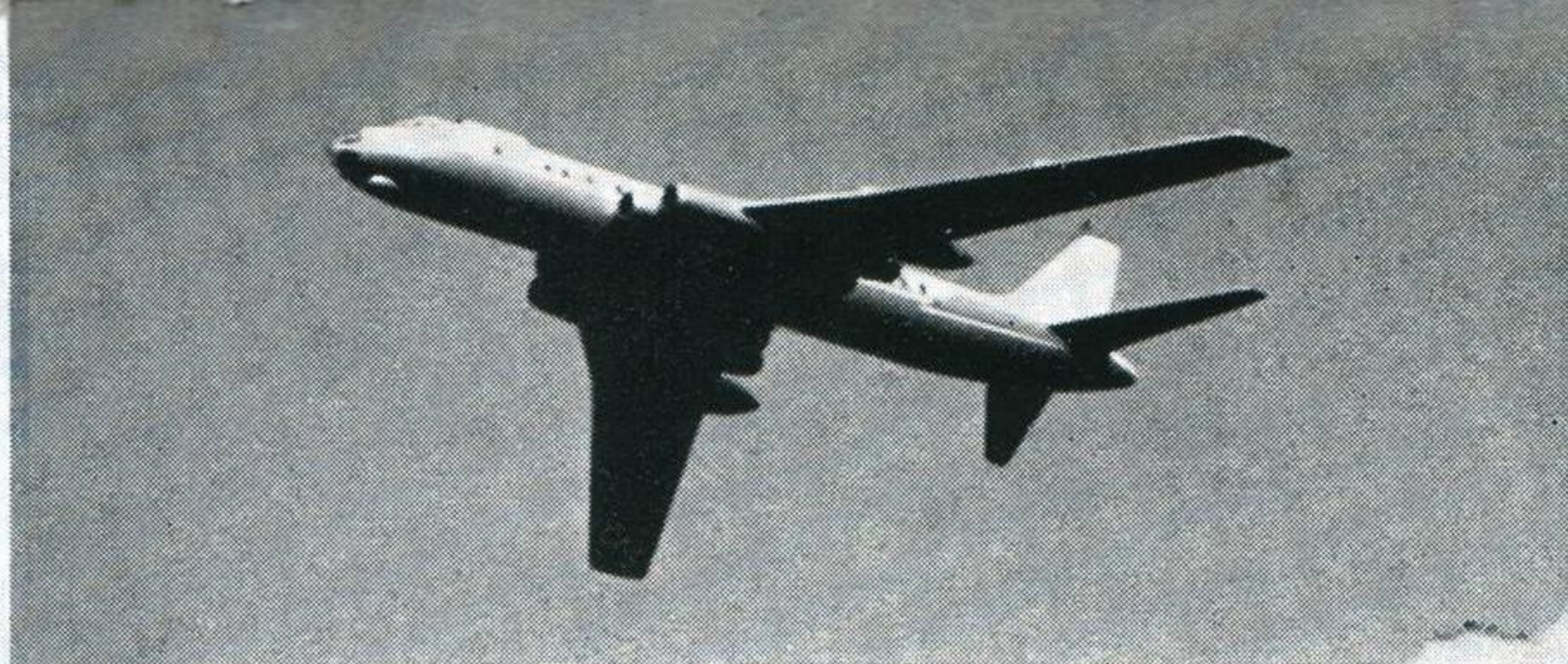
COOKER A four-jet version of the Camel with lengthened fuselage that did not go into large-scale production. Span 123 feet
