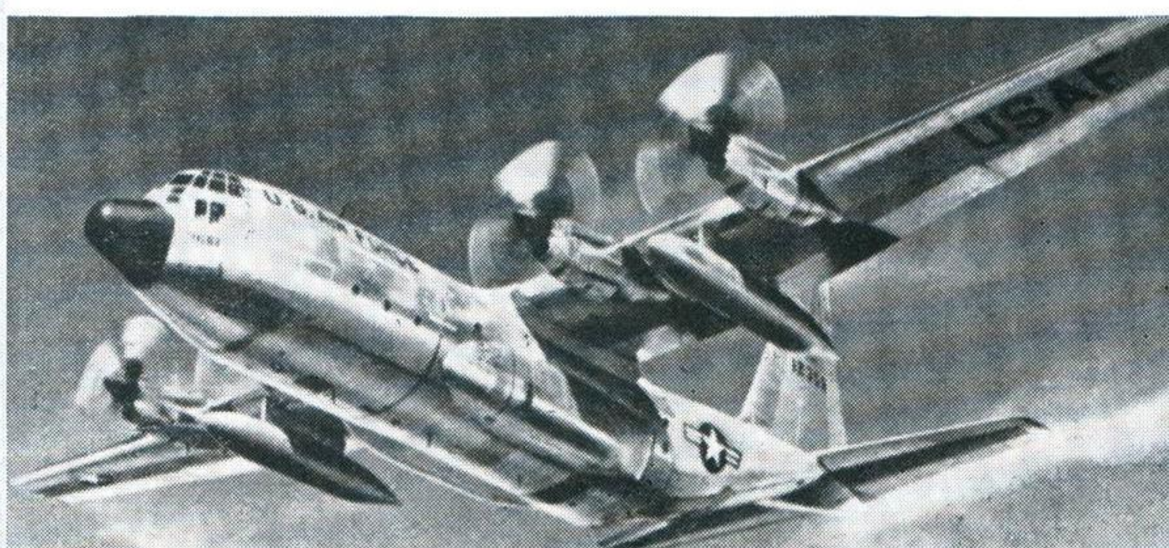
HERCULES U.S.A.F. standard transport, the C-130 Hercules, is built in several versions and is in use in the R.C.A.F., R.A.A.F. and S.A.A.F. as well as the air arms of Iran, Indonesia and Pakistan. Span 133 feet
