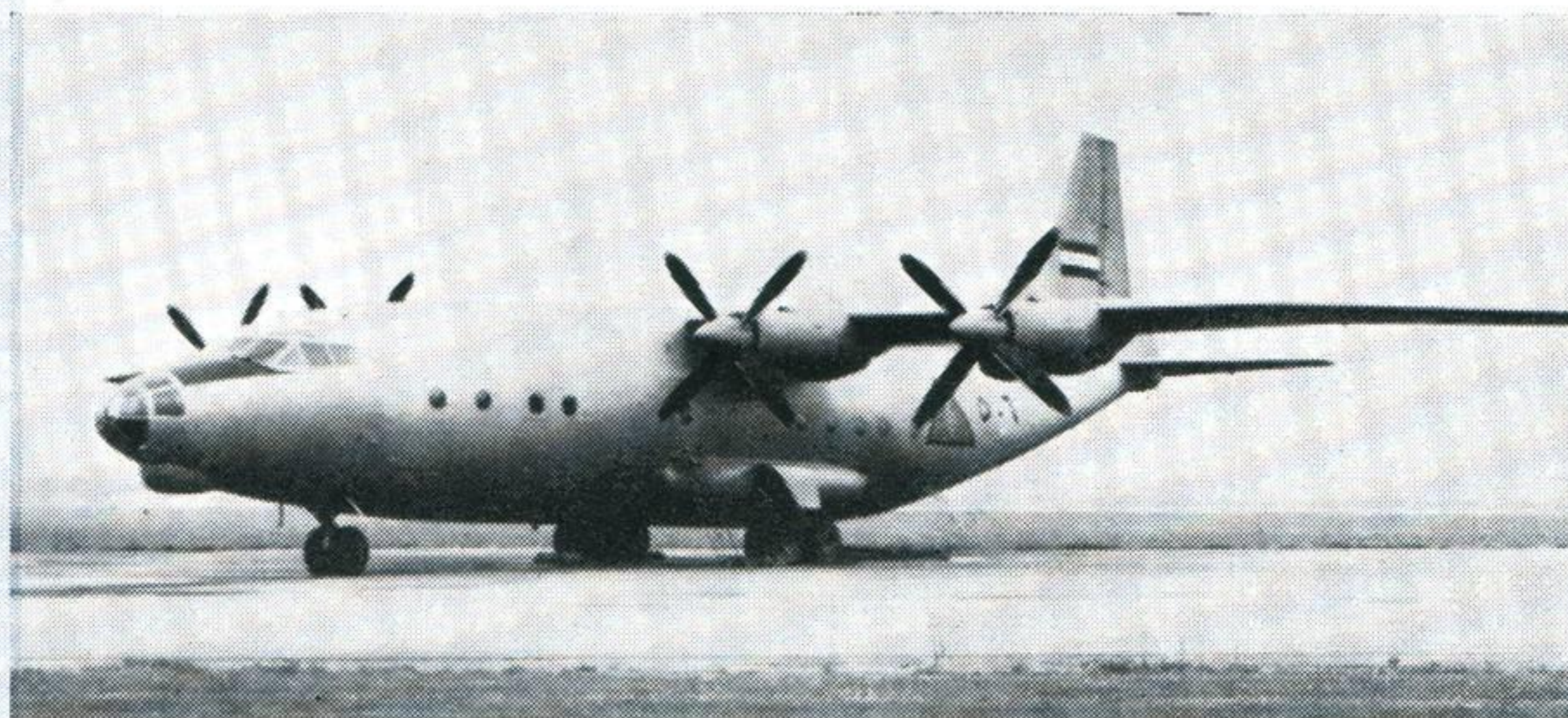
CUB Military development of Cat with raised tail to permit rear-loading, serving in Egyptian, Indian, Indonesian and Iraqi colours as well as with Red Star markings. Span 125 feet
