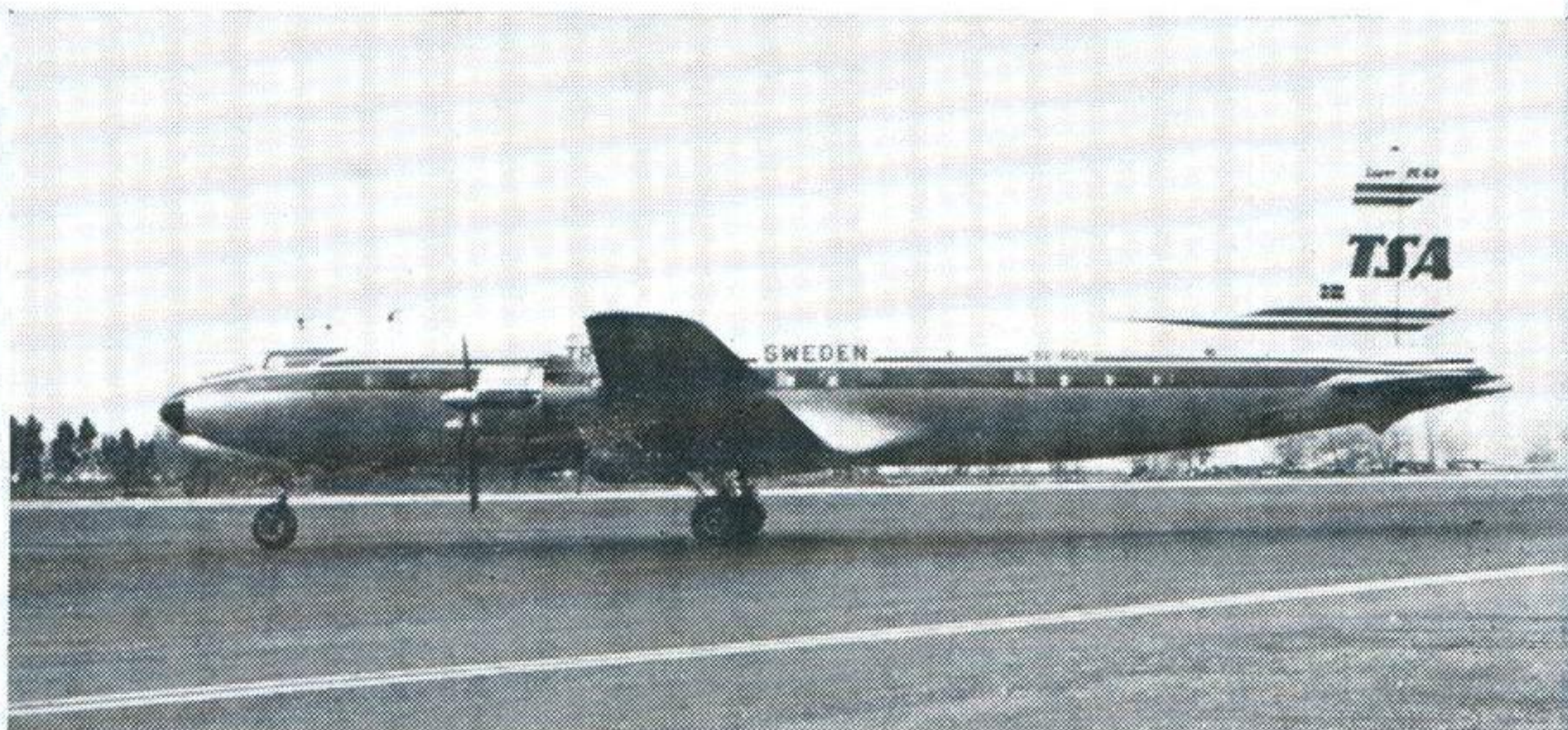
DC-6 A later version of the DC-4 with a fuselage stretch of 7 feet together with DC-6A freighter and DC-6B airliner with further length increases, are still widely used. Span 117 feet
