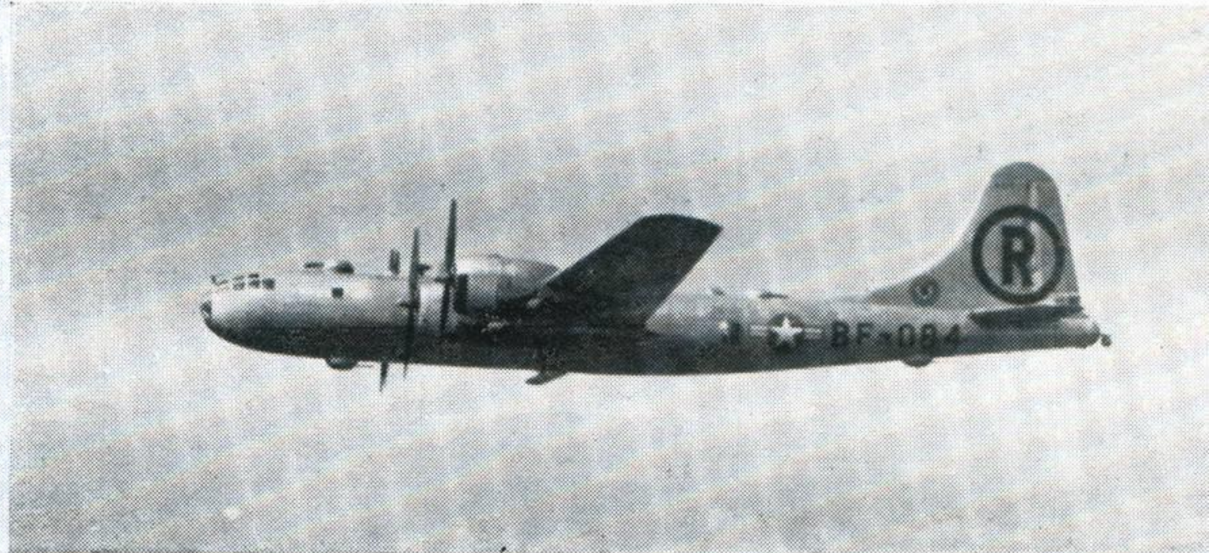
SUPERFORTRESS (B-29) Only the TB-29A version of this wartime production order veteran remains, but it is possible that some of the Russian-built models, named Bull, are still serviceable. Span 141 feet
