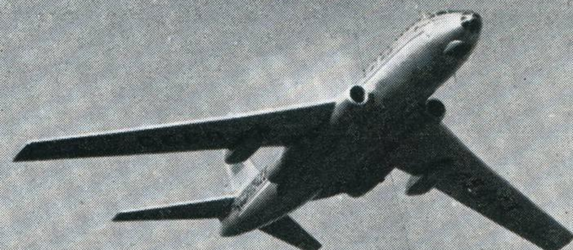
CAMEL Civil counterpart of Badger, this Aeroflot Tu-104 airliner is produced in several versions with variations of a few feet in fuselage length. Span 113 feet
