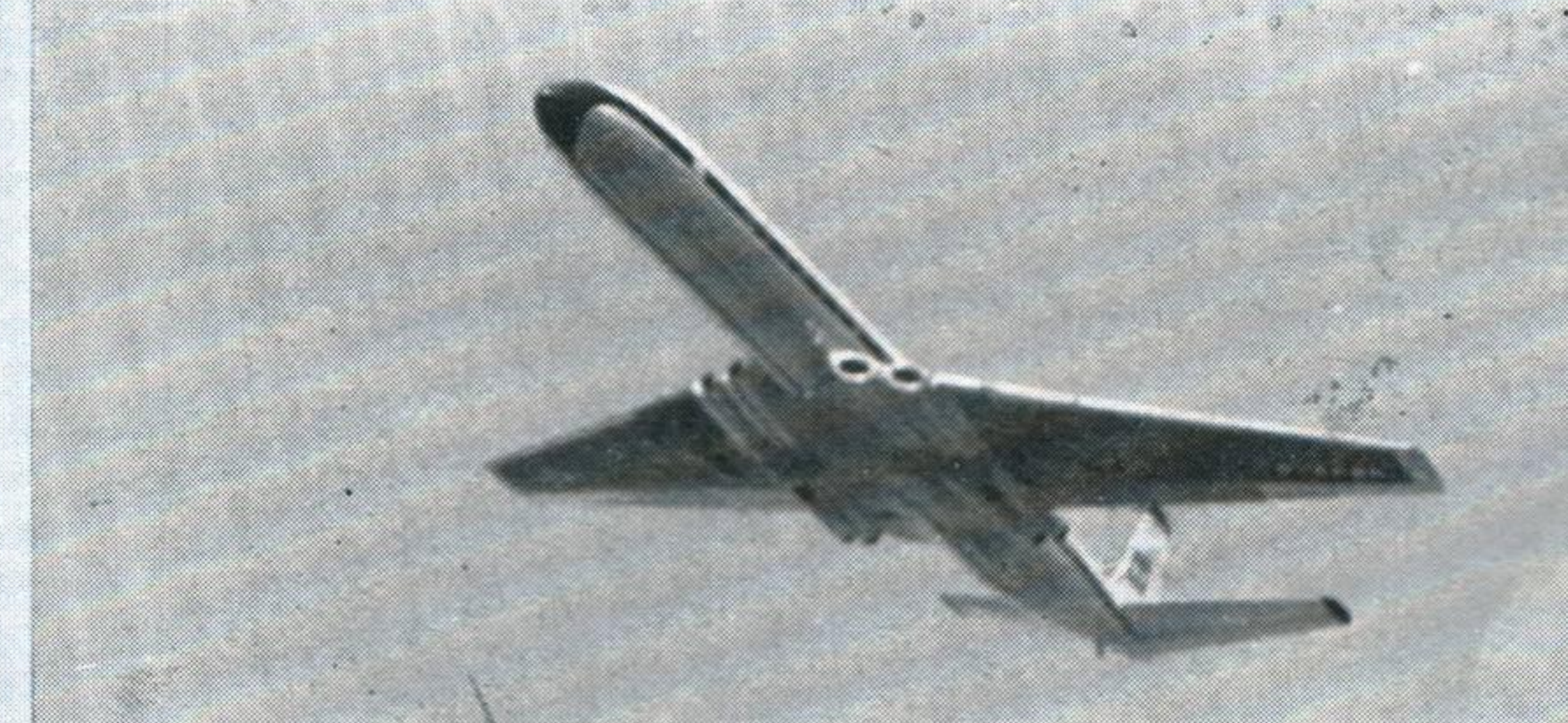
COMET 4B With a cropped wing and lengthened fuselage this is a medium range version of the Comet. Span 108 feet
