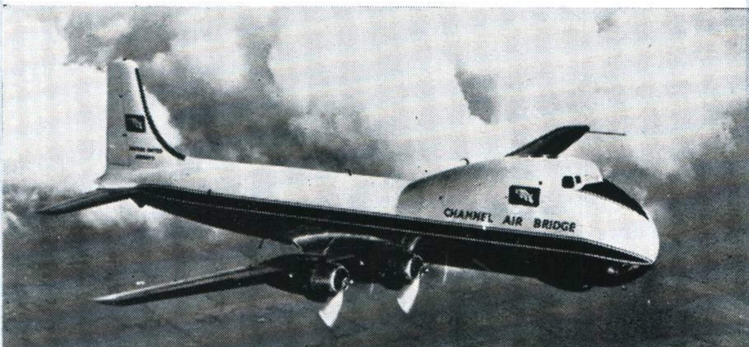
CARVAIR A British modification of the DC-4 Sky-master, with DC-7 type fin and rudder, for the conveyance of cars of which it can carry five at a time with 22 passengers. Span 117 feet
