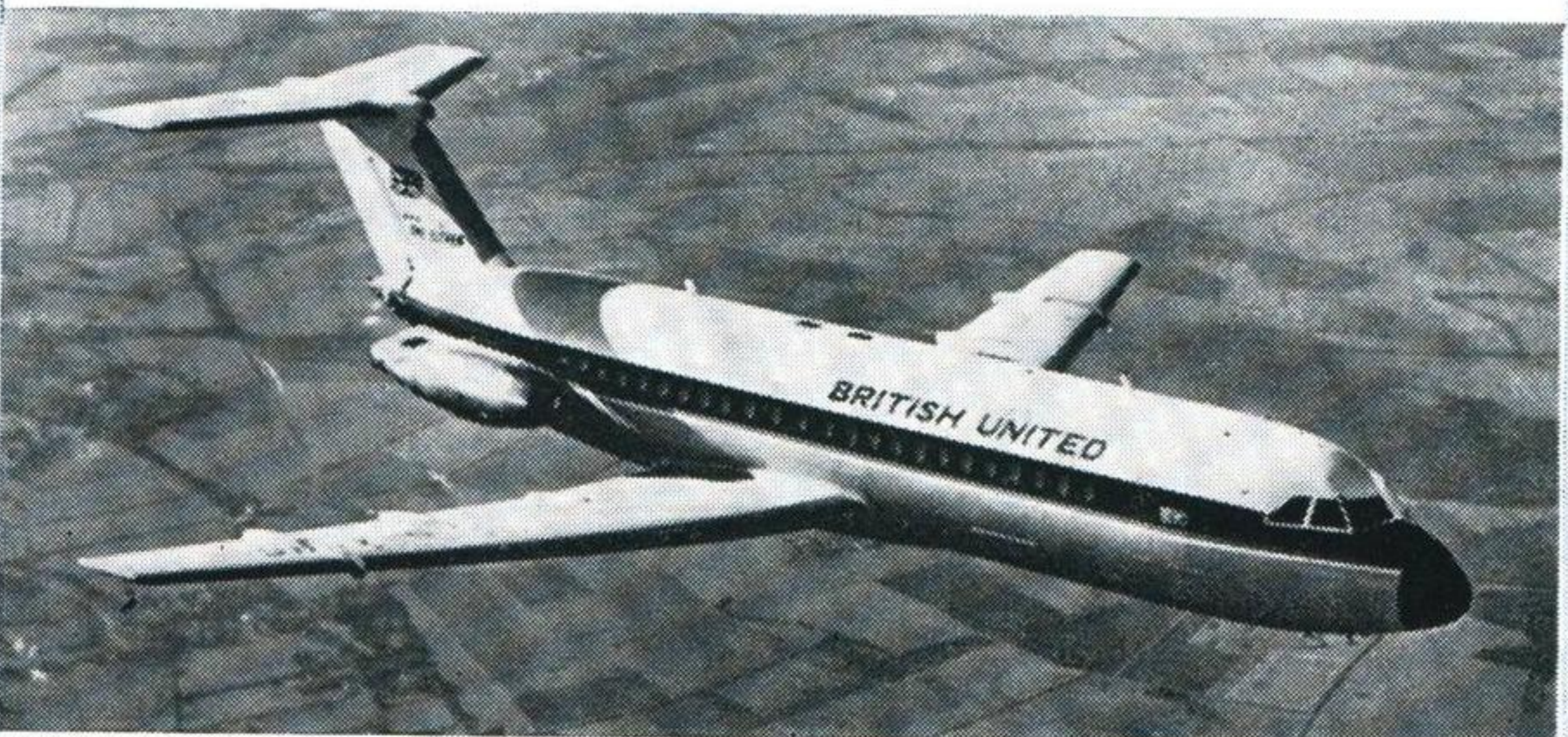
ONE-ELEVEN Some fifty of these B.A.C. short to medium haul transports are expected to enter service this year. Series numbers 200, 300, 400 apply according to loadings and power units. Span 88 feet
