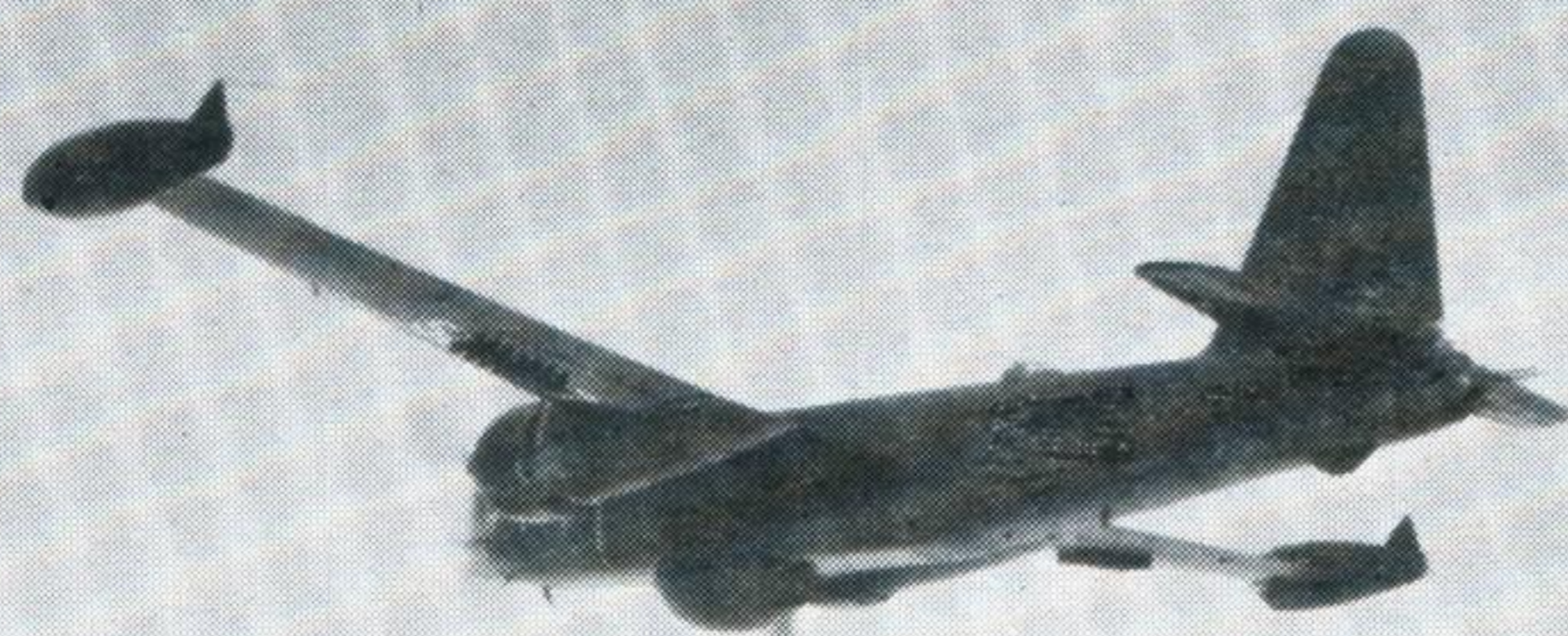
NEPTUNE A version once used by the R.A.F. and still in use in other countries for maritime reconnaissance. Span 100 feet
