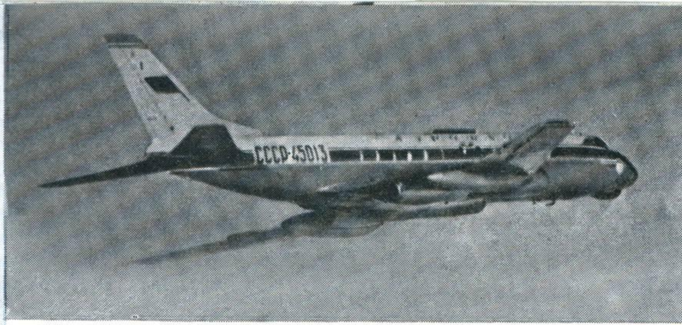
COOKPOT In effect this Tu124 is a scaled down version of Camel (see page 37) used almost exclusively on Russian internal airlines. Span 84 feet
