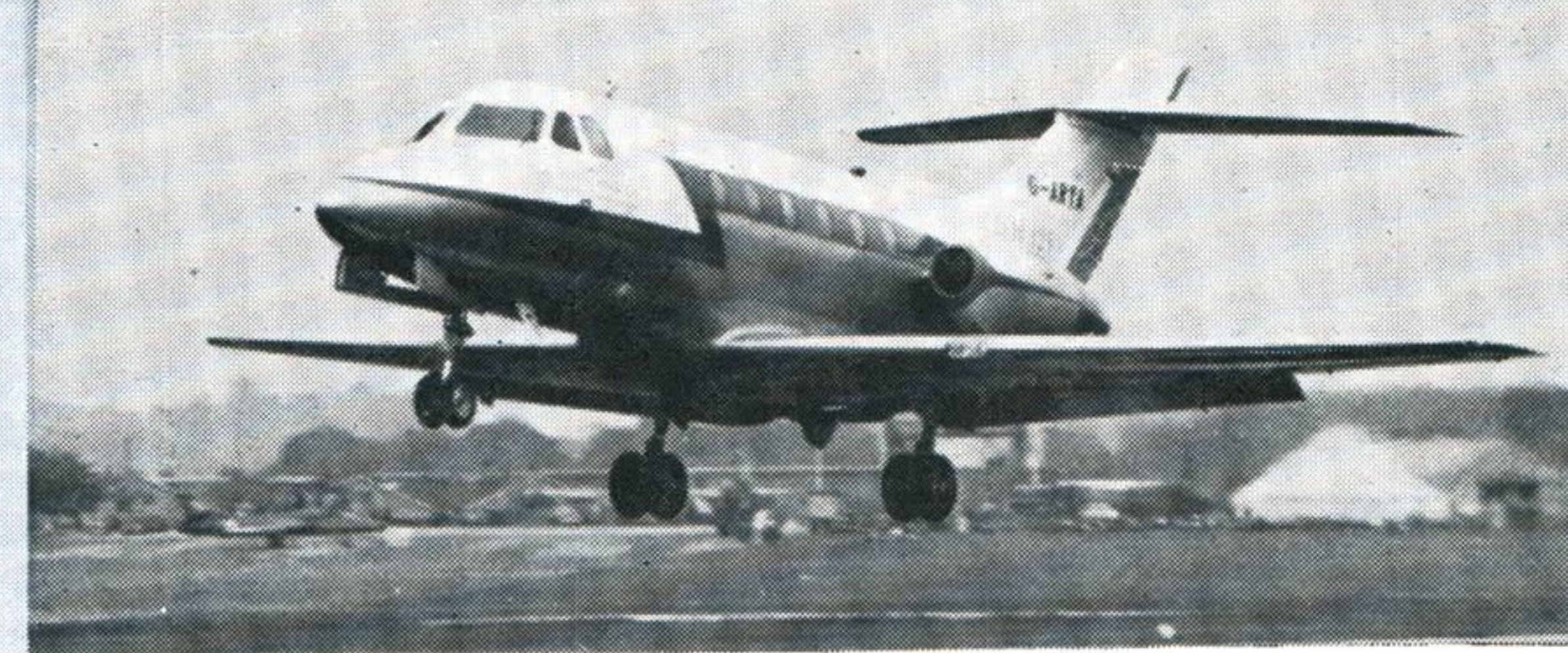
DOMINIE As Dominie T.1 the HS125 (formerly DH125) will enter the R.A.F. for navigational training and is on order as a light civil transport with several organisations. Span 47 feet
