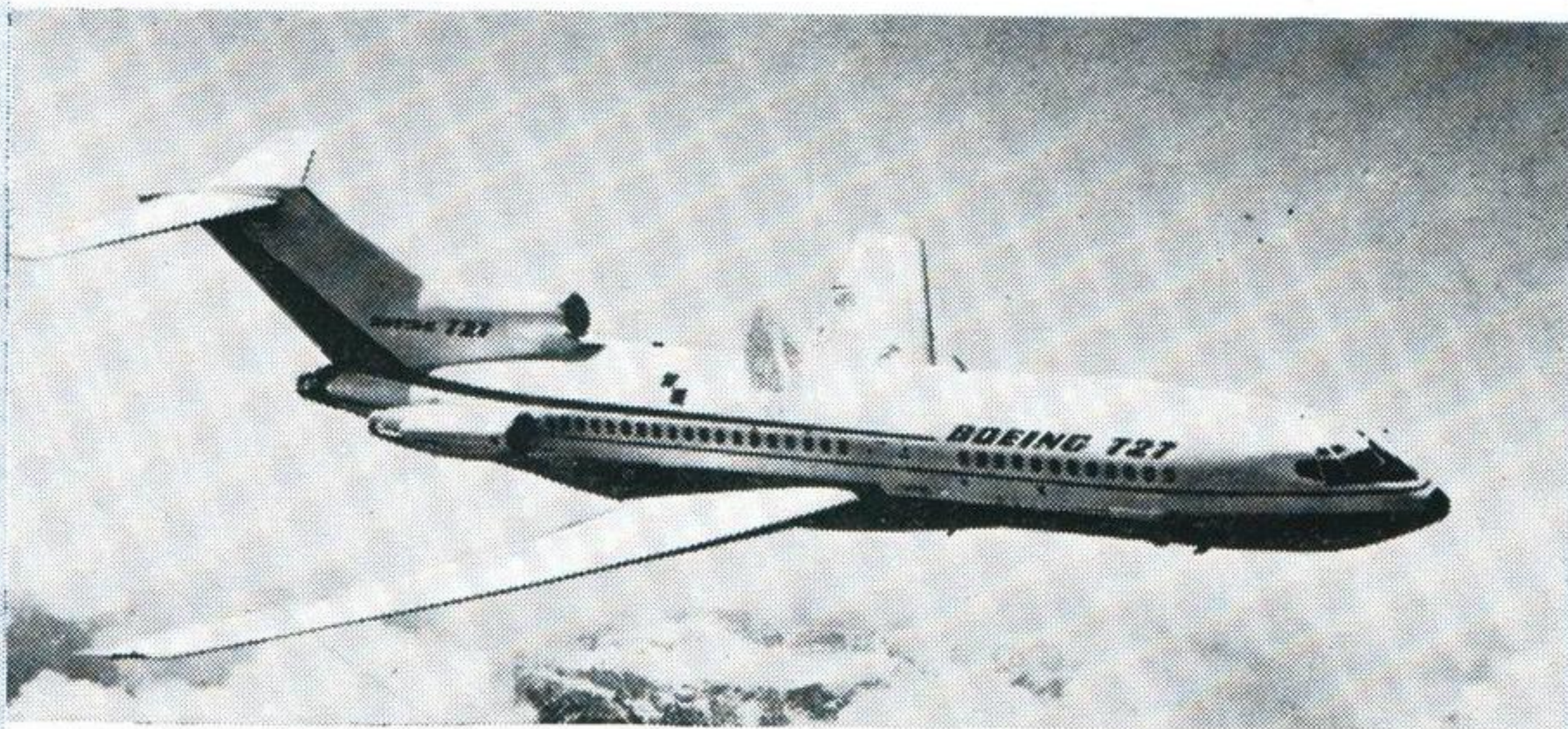
BOEING 727 In the same class as the Trident, this Boeing is on order for various airlines world-wide, including German and Japanese lines. Span 108 feet
