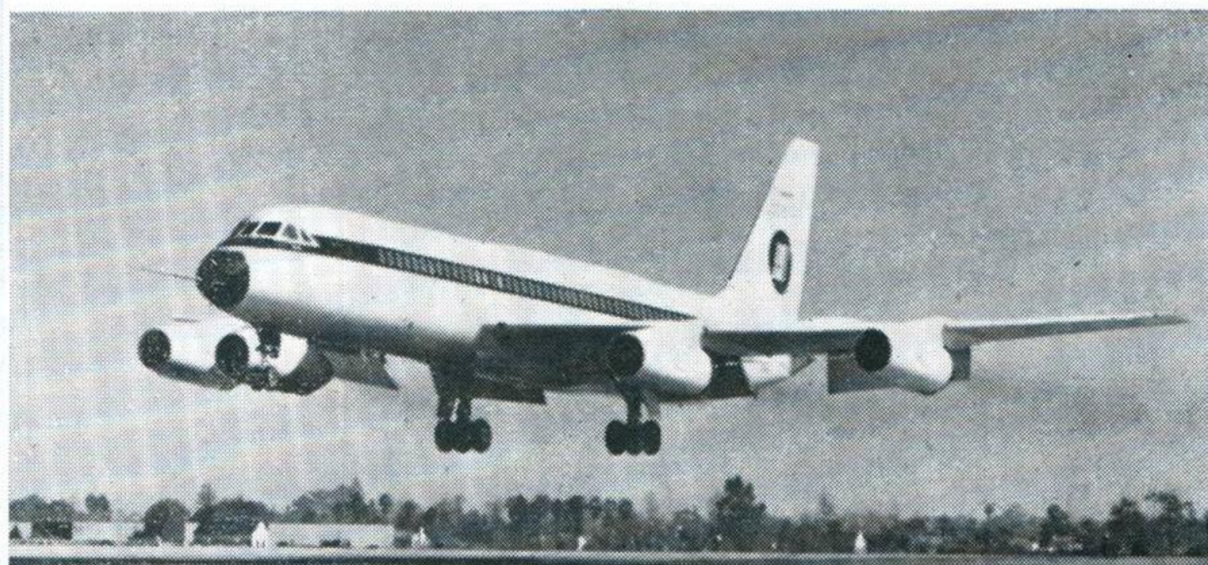
CONVAIR 990A Developed from the Convair 880, the 990 has a large fuselage with increased accommodation. Modifications prior to service has resulted in the designation 990A. Span 120 feet
