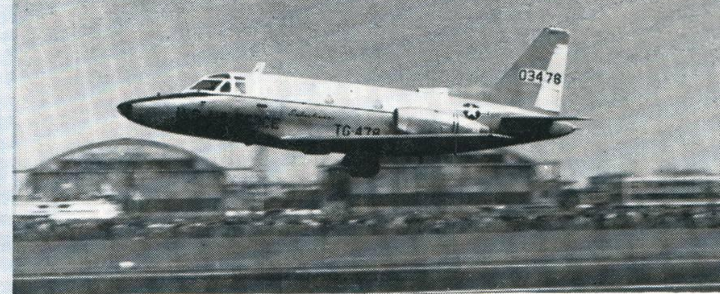
SABRELINER The North American T-39 of the U.S.A.F. and U.S. Navy is used both as a combat and a utility trainer in three basic versions of similar configuration. Span 44 feet
