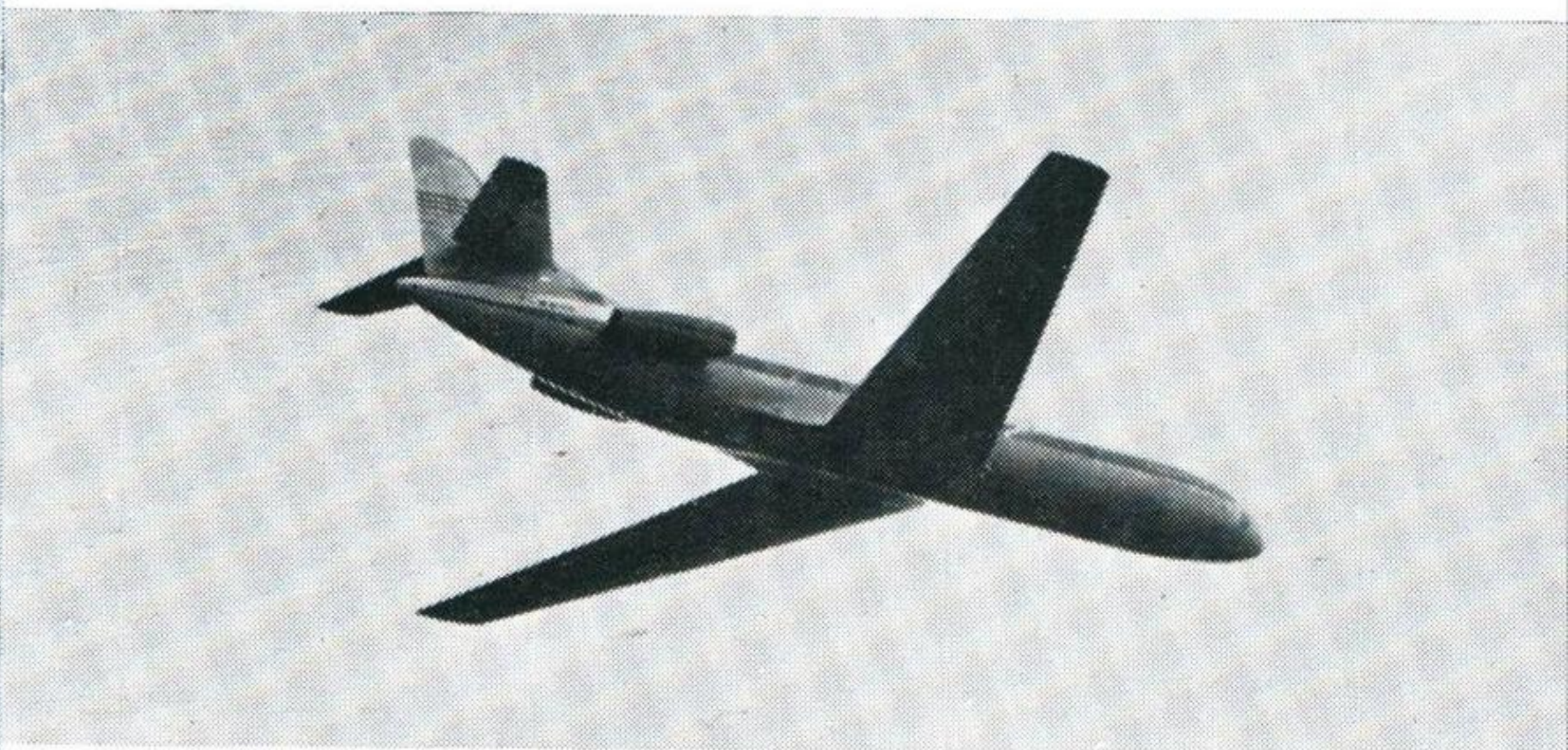
CARAVELLE First of rear-jet civil transports, this French airliner is produced in several versions with only minor variations, but see also Caravelle Super. Span 112½ feet
