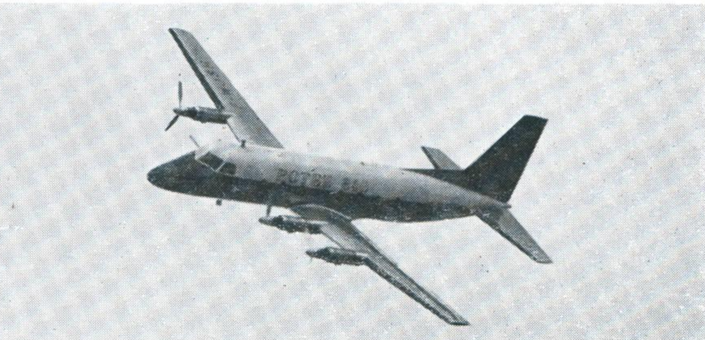
POTEZ 842 From the prototype Potez 840, a production series designated Potez 842 is being prepared in two versions with variations in fuselage length. Span 64 feet
