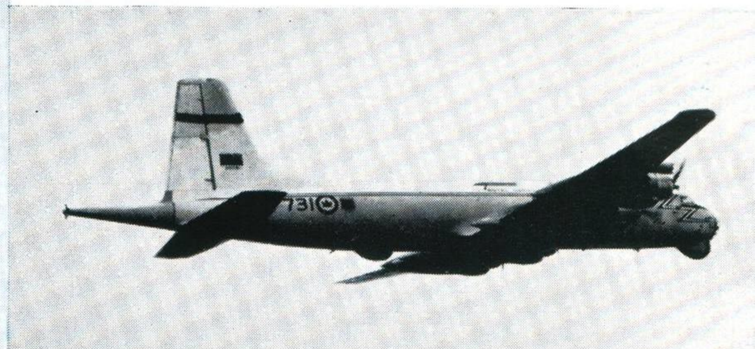
ARGUS The R.C.A.F.'s counterpart of the maritime reconnaissance Shackleton was based on the Bristol Britannia. Size of chin radome varies accordingly to Mk. 1 or 2 versions. Span 142 feet
