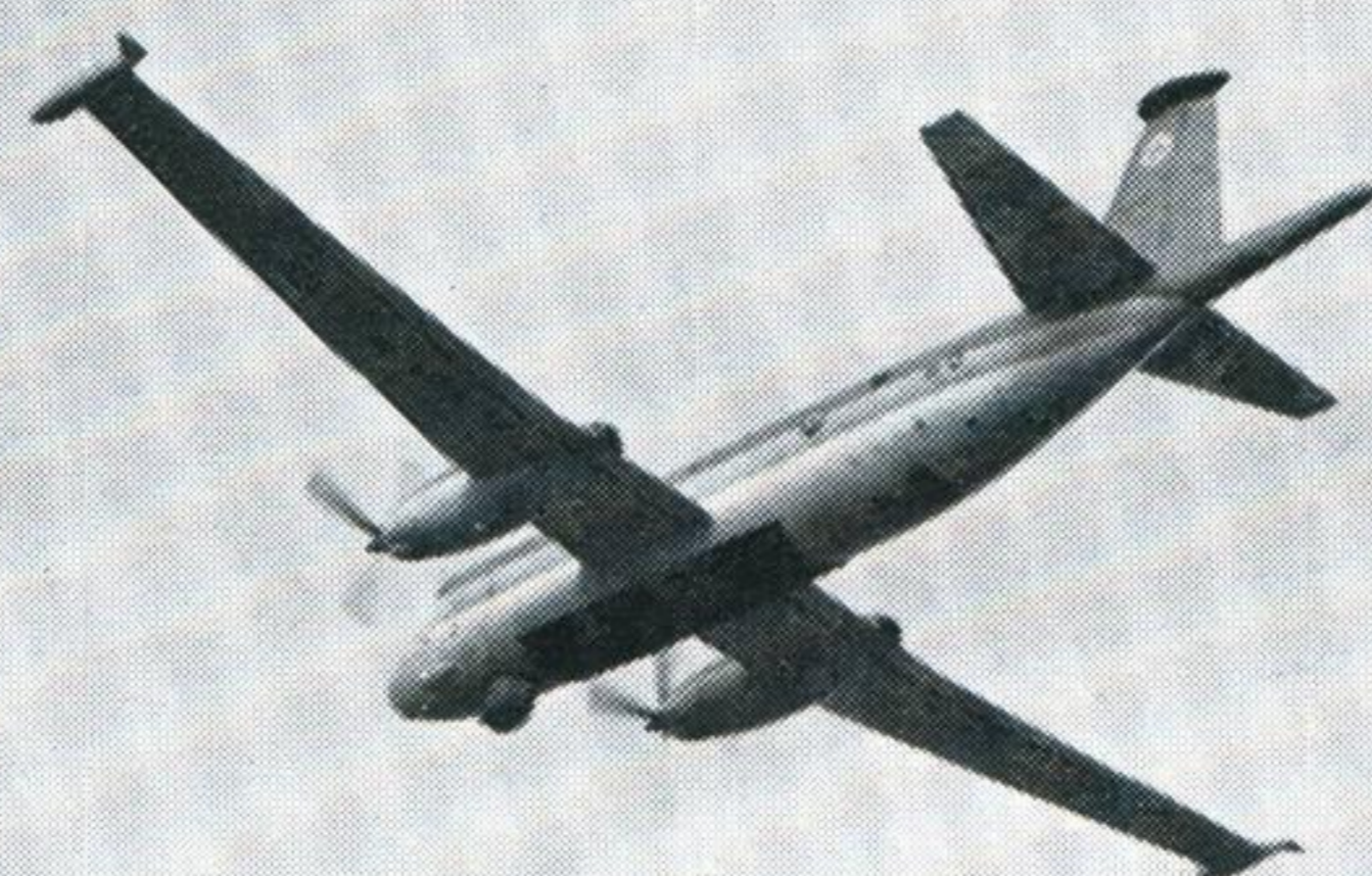
ATLANTIC Built by Breguet under joint Dutch, Belgian, German and French co-operation, this maritime reconnaissance aircraft is expected to enter service towards the end of the year. Span 119 feet
