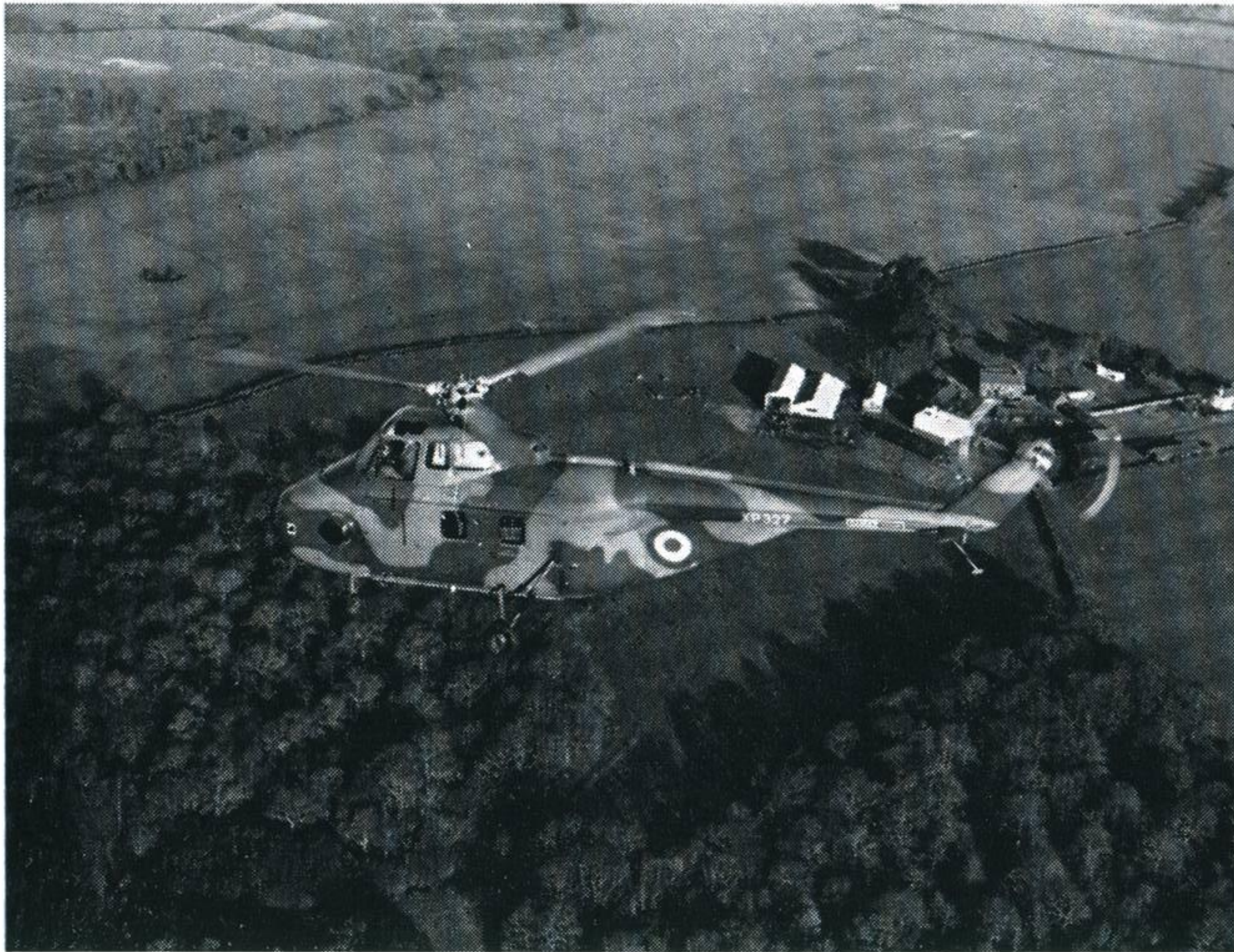
Cover Photo: A Whirlwind H.A.R.10 of the R.A.F.; some earlier Mk. 2 and 4 have been converted to this standard by replacing their piston engines with turbine power.
