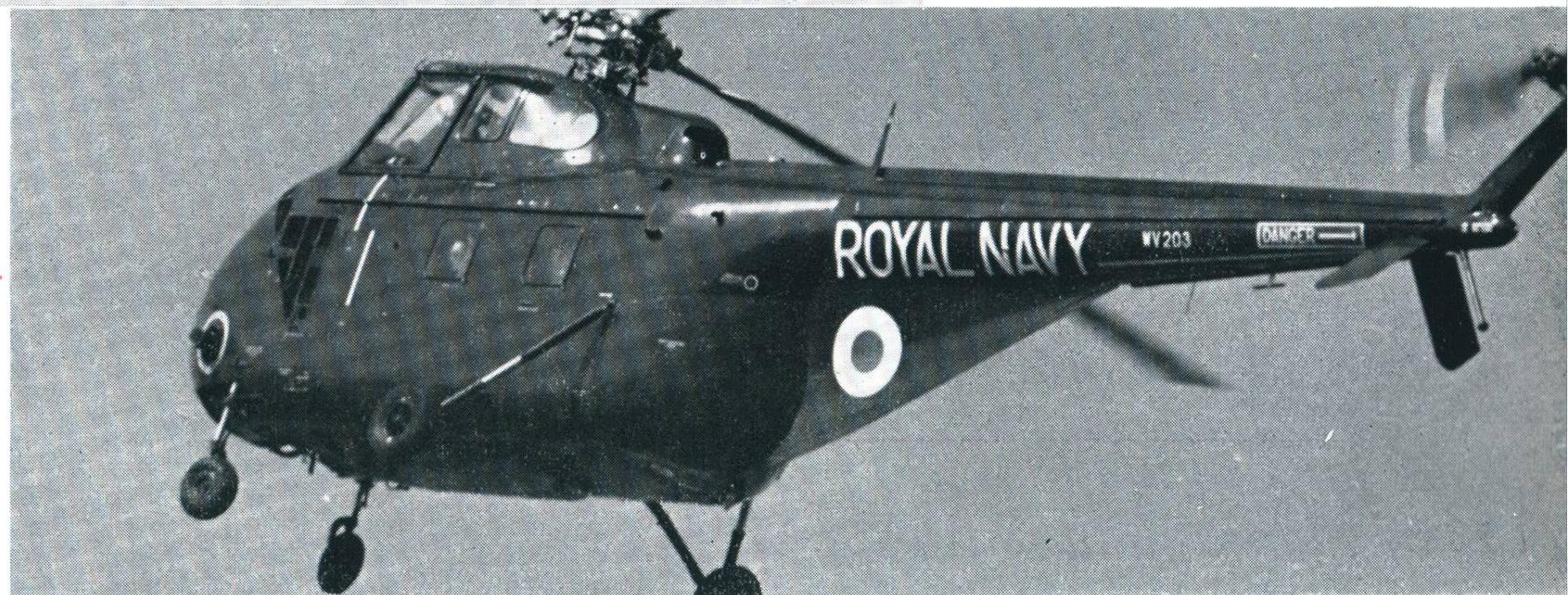
▶ The H.A.R.10, the first of the Service versions of the Series 3 Gnome-engined Whirlwinds is in service with Coastal, Transport and Flying Training Commands of the R.A.F.
