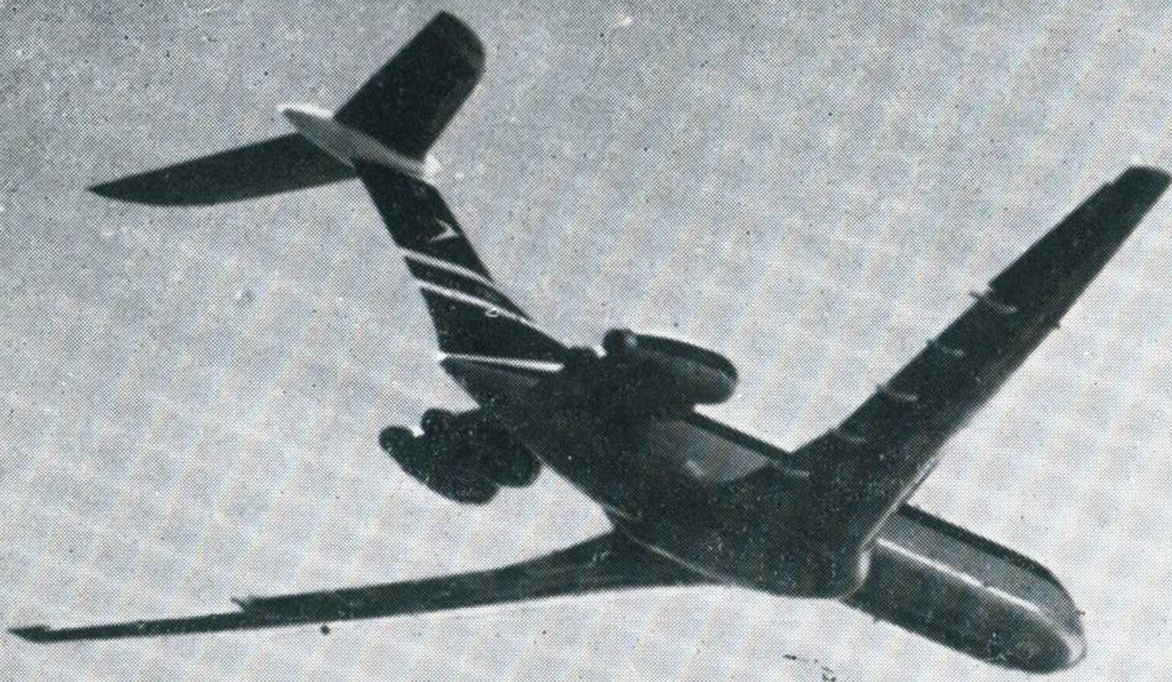
Two four-engined rear-jet airliners with similar configurations, the British Vickers VC10 and Russian Il-62 Classic.
