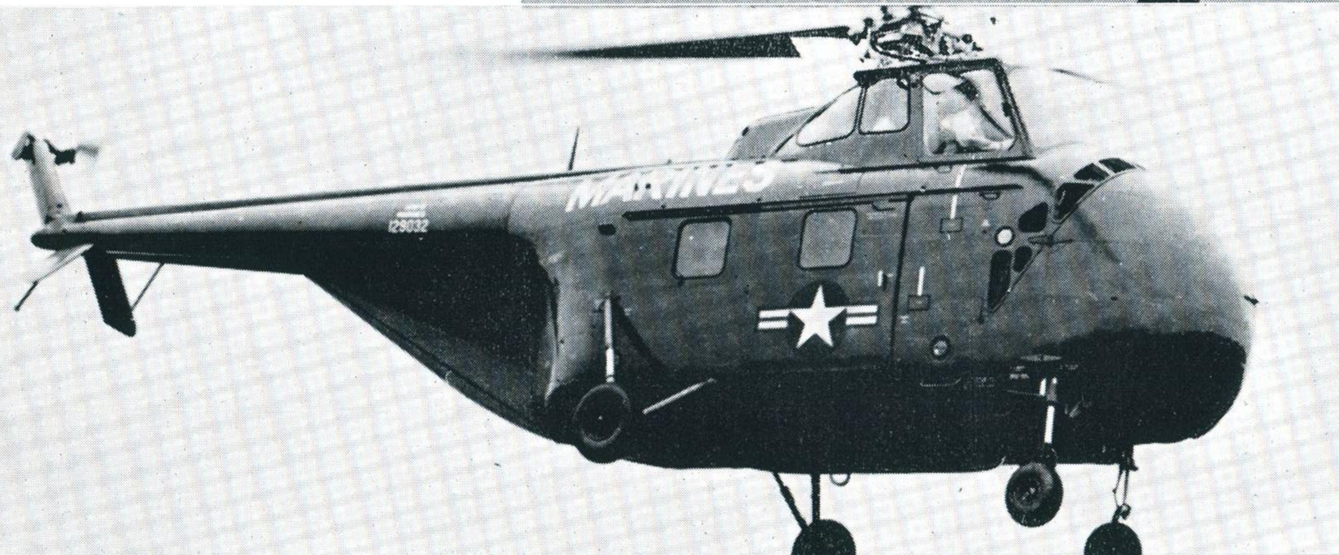
▶ Early versions of the Whirlwind, including the American-built S-55s supplied under Mutual Defence Aid arrangements are still in limited R.N. use as the H.A.S. 22 (as shown).
