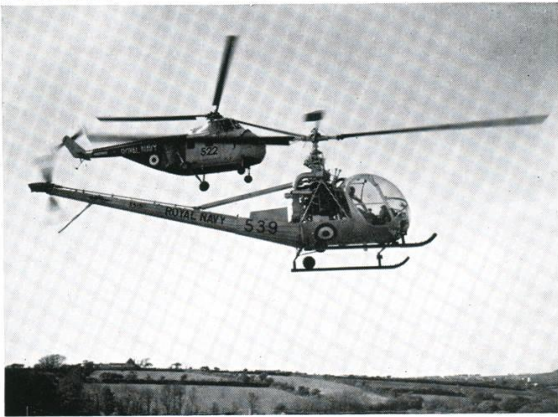
A Hiller 12E of the Royal Naval Helicopter School at Culdrose in company with a Whirlwind. These new Hillers have completely superseded the earlier HTV-2 type operated by the Royal Navy.
