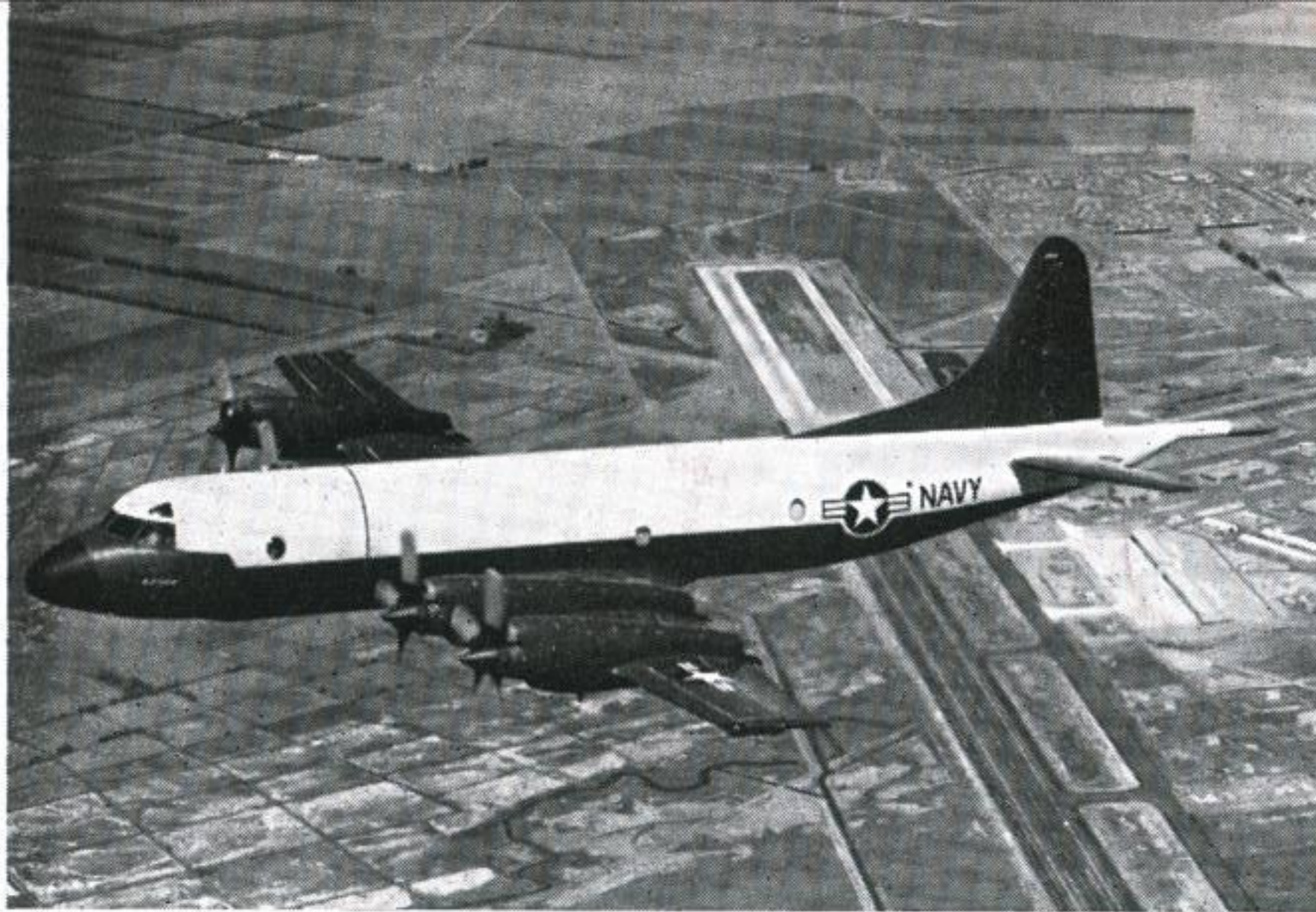
Cover Photo: Orion. In rather the same way that the basic Britannia design was adapted for the Royal Canadian Air Force as their Argus, so the turbo-prop Lockheed Electra airliner has been adapted as the U.S. Navy's latest anti-submarine patrol aircraft, the P-3A Orion.
