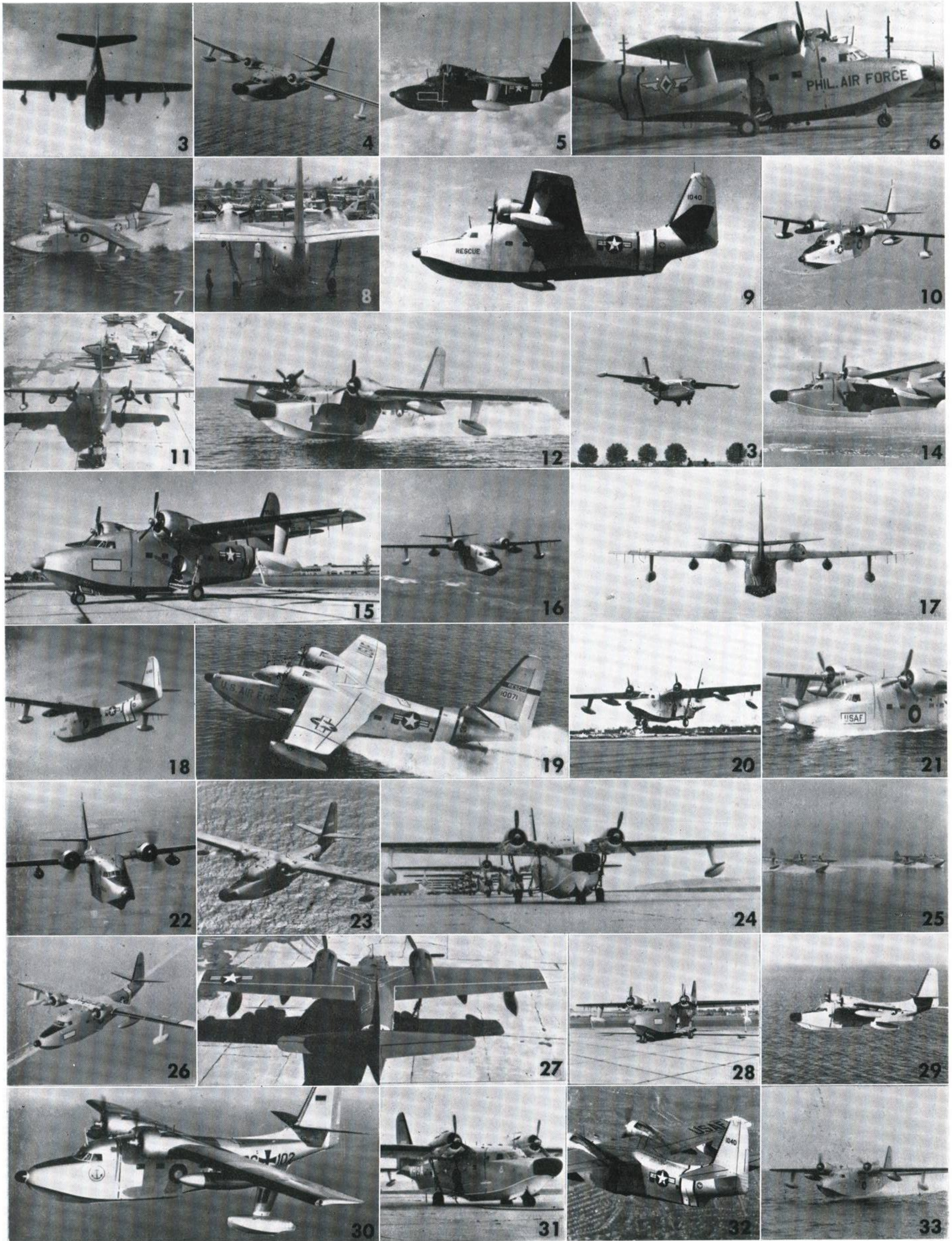
In target No. 27, the dayglo paint on the wing tips gives a false impression of wing shape.
