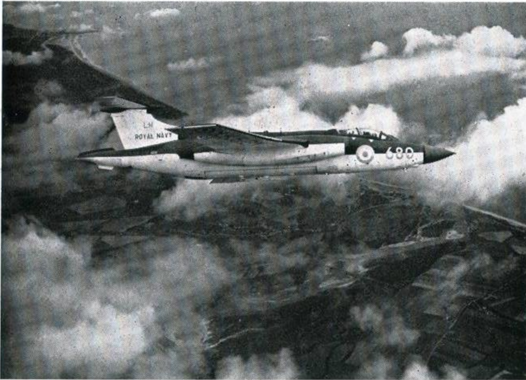
Cover photo: A Buccaneer S.1 (previously known as the Blackburn N.A.39) of the initial production order for twenty flying along the coast. In typical Royal Navy aircraft colours of white and extra-dark sea grey, it is understood that later production aircraft, like the R.A.F.'s 'V' Bombers, will be all-white. The Buccaneer S.1 is powered by two D.H. Gyron Junior turbojets, and a new version, known as the S.2, with two Rolls-Royce Spey turbofans, has been announced.
