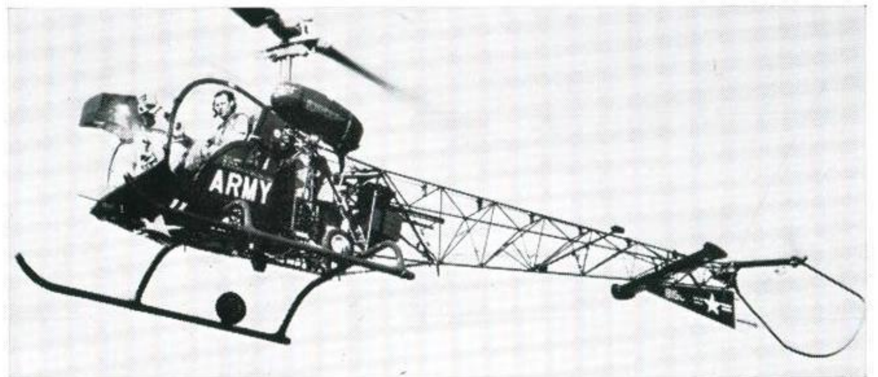
Sioux SOO. Military version of the Bell 47G Trooper helicopters which the U.S. Army have named Sioux.
