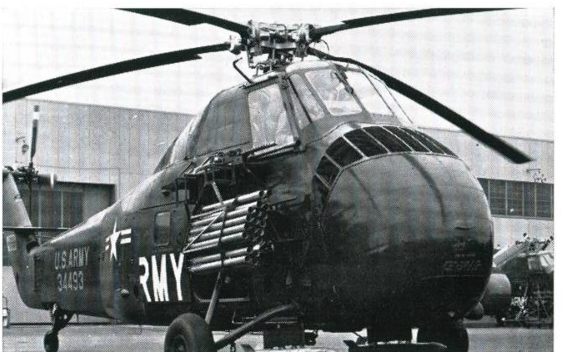
Choctaw CHOK-taw. As the H-34 Choctaw in the U.S. Army, this Sikorsky helicopter is built in Britain as the Wessex.
