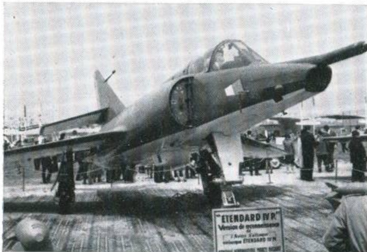
The French Étendard IV P, a version of the IV M with a nose-probe and camera pack.
