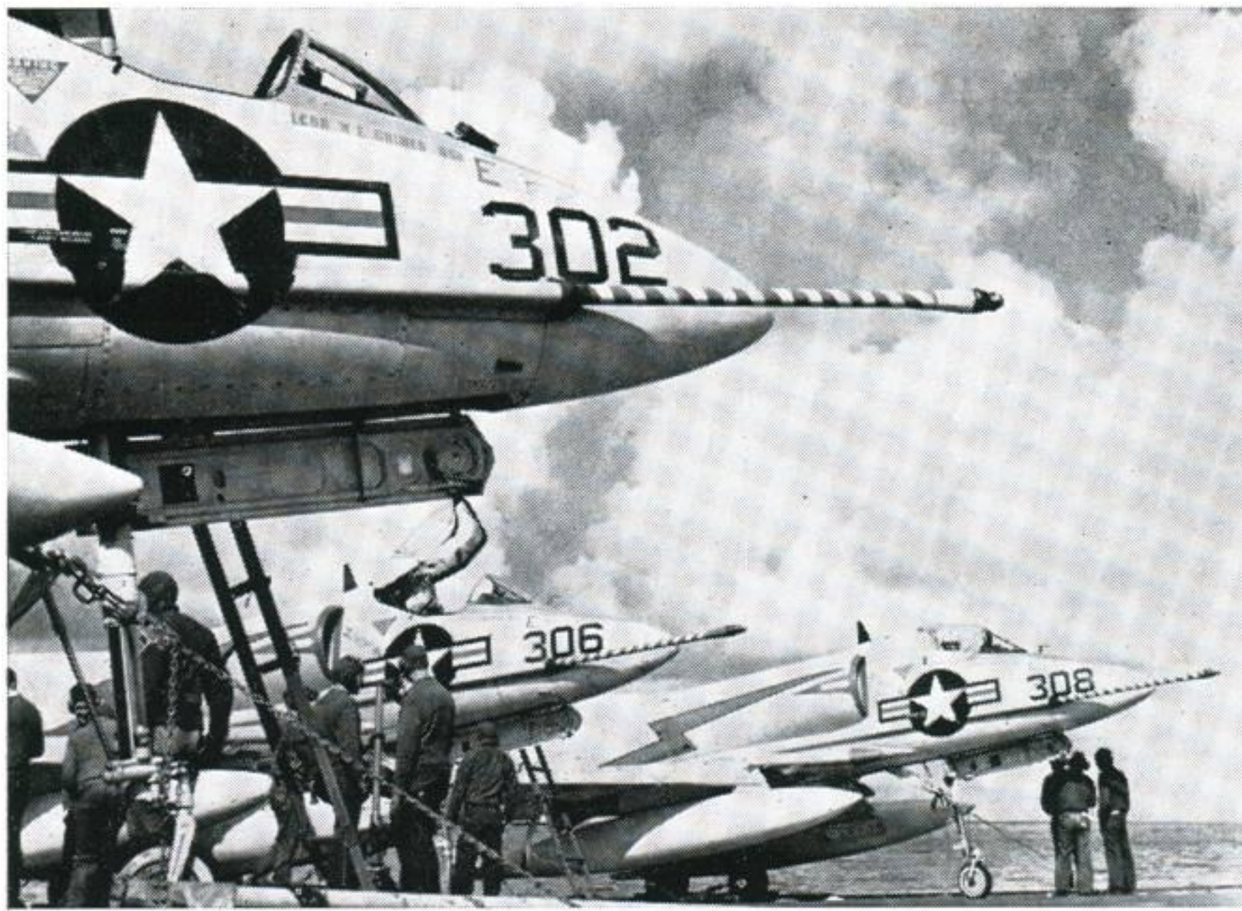
DOUGLAS A4D SKYHAWKS on the U.S.S. Franklin D. Roosevelt . Skyhawks can carry a variety of stores including nuclear and H.E. bombs, Sidewinder infra-red missiles, Zuni or Mighty Mouse air-to-air rocket packs and Bullpup air-to-surface missiles, ground attack gun pods or torpedoes, added to which there is a fixed armament of two 20-mm. Colt cannons. Carrying a 3,000-lb. weapon load under the fuselage and with racks for two 1,000-lb. weapon or fuel loads under the wings, the Skyhawk rates as—a light attack bomber!—and there's about a thousand of them!
