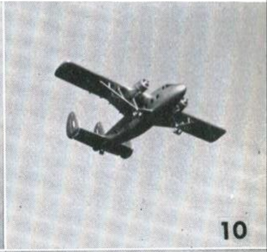
A Twin Pioneer equipped for geophysical survey duties. The wing-tip pods contain electro-magnetic equipment.
