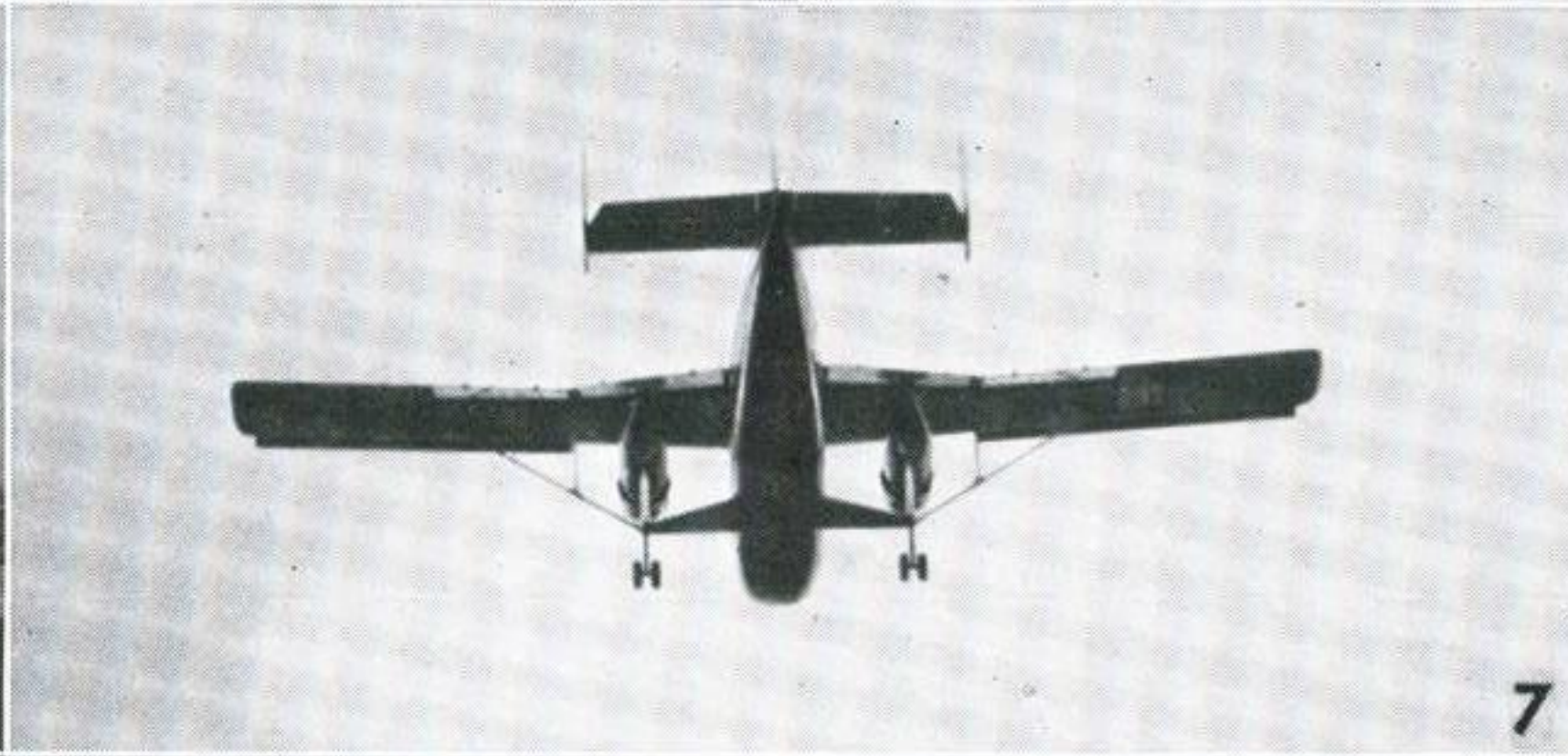
A Twin Pioneer equipped for geophysical survey duties. The wing-tip pods contain electro-magnetic equipment.
