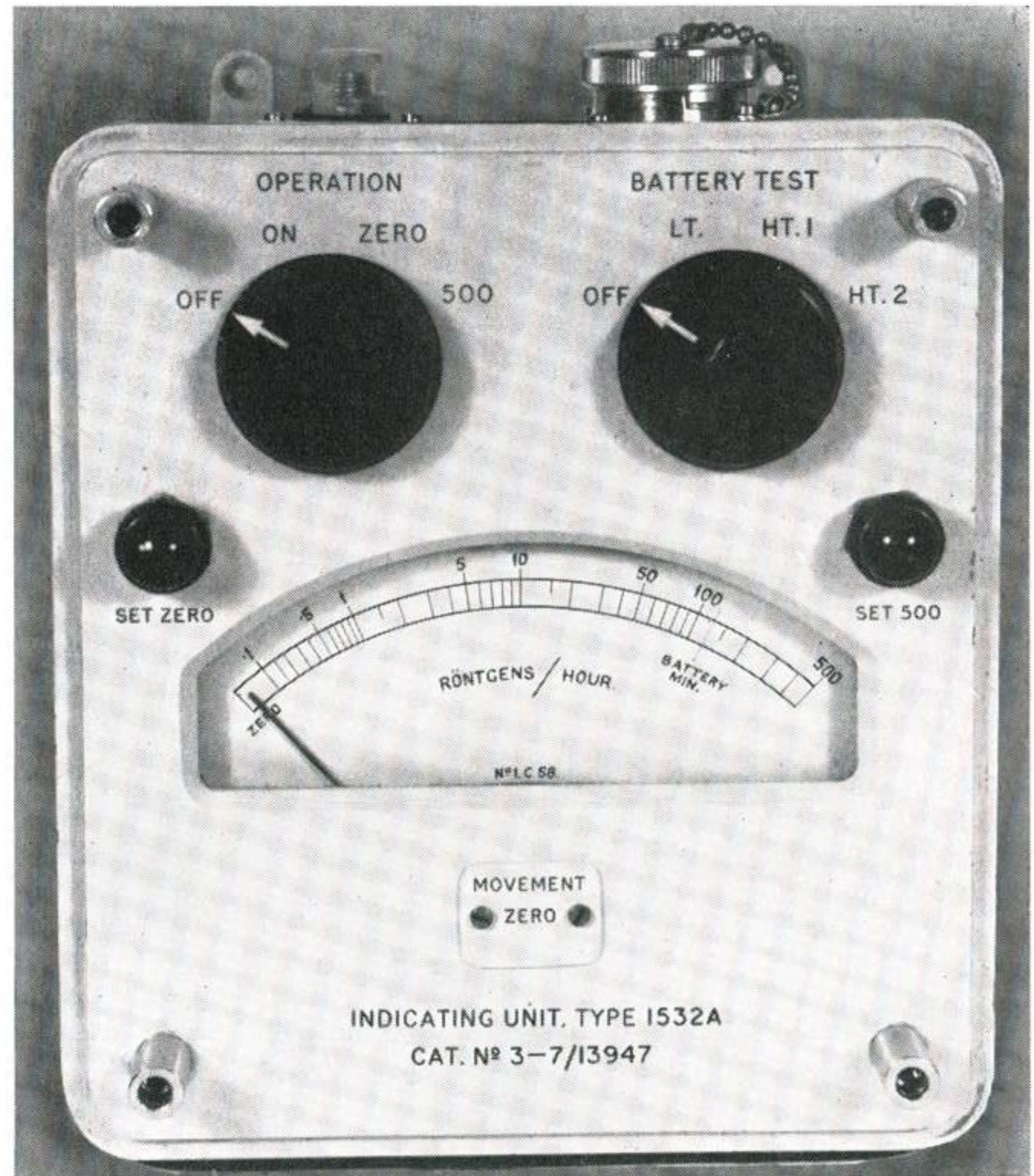
Fig. 7. The Indicator Unit. The cable socket at the top and the lugs which are used for screwing the unit to the instrument shelf can be seen; there are two similar lugs at the bottom of the unit. The scale shown on this prototype instrument is not standard, nor is the small fitting on top to the left of the cable socket.
