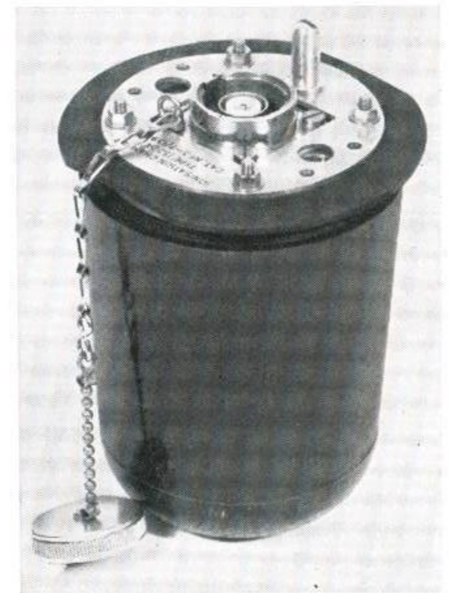
Fig. 3. The Ionisation Chamber. The cap has been removed from the connector socket.
