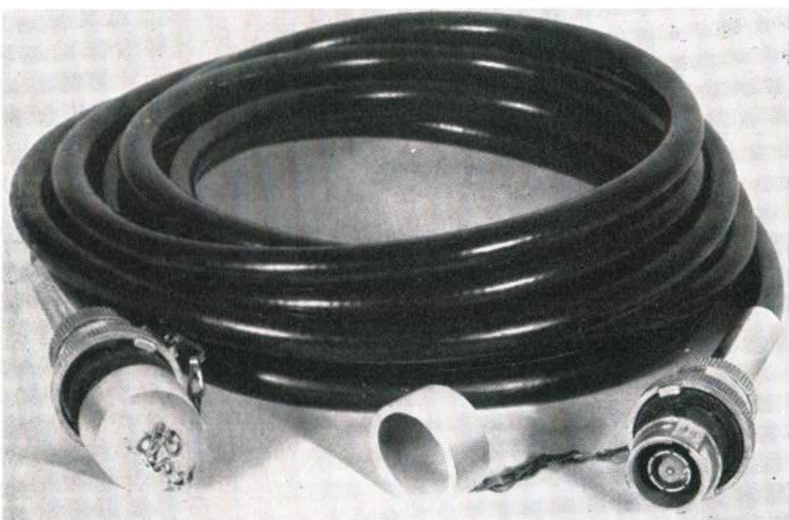
Fig. 6. The Inter-Connecting Cable. One of the connector caps is shown removed.
