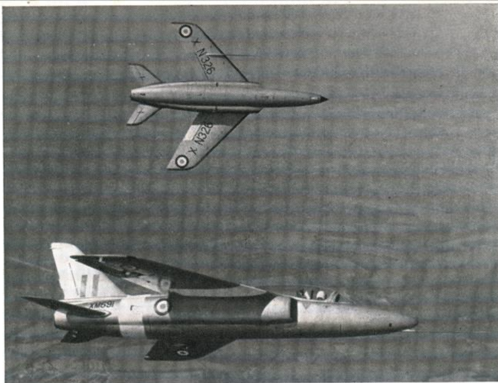
Cover Picture: Peeling off is the Folland Gnat Mark I fighter; about to do so is the two-seater transonic trainer version, being one of a development batch of 14 ordered by the Ministry of Aviation. The makers say that although the two-seater Gnat owes much to the single-seater Mark I, it is a new design and not an adaptation.
