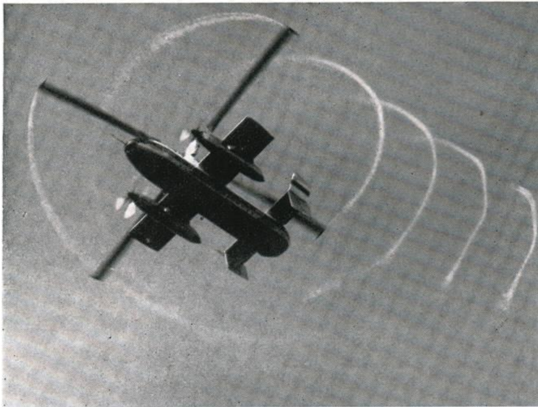
Cover Picture: The Fairey Rotodyne, tracing a spiral in the sky as it lights the tip-jets of its four-blade rotor in preparation for the transition from forward to hovering flight.
