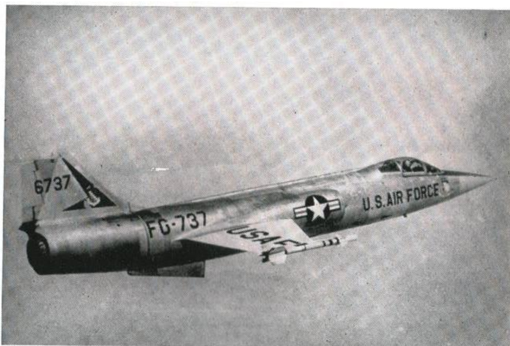
Current holder of the World's Air Speed Record, the F-104 Starfighter has already used its Sidewinder missiles (seen here at the wingtip) under operational conditions.
