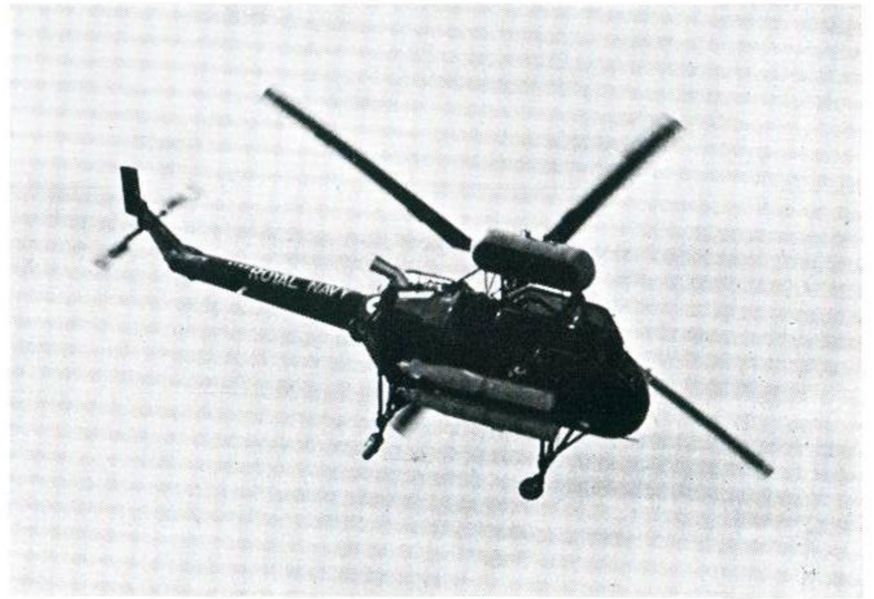
Wasp with two Mk 44 torpedoes above, and below with torpedoes and outrigger flotation gear.
