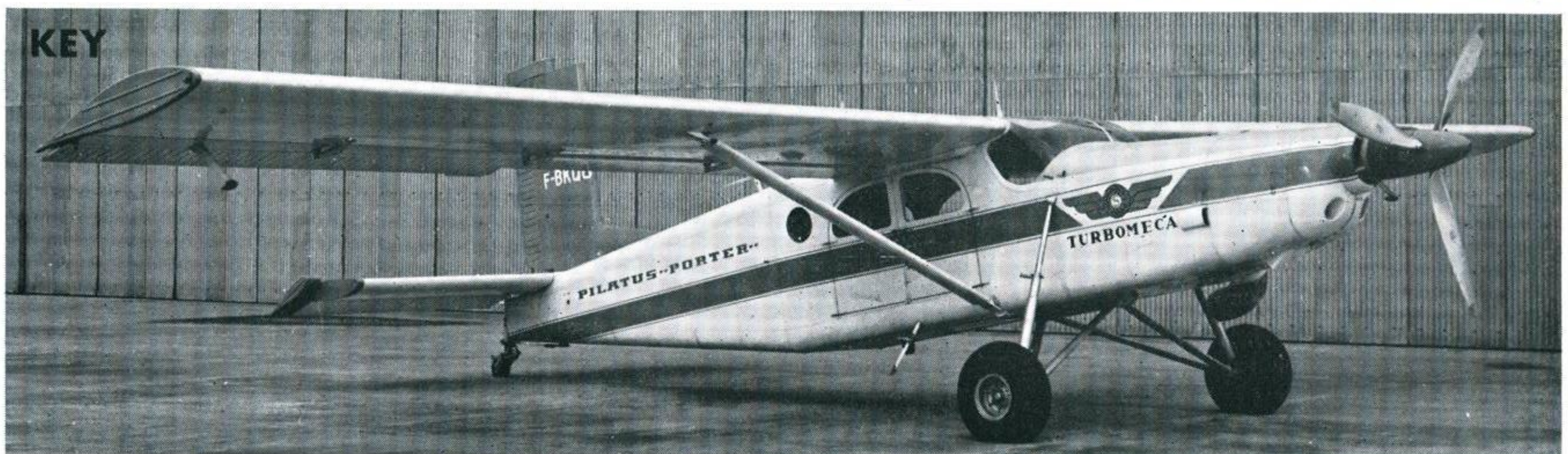
An adaptable aircraft, Porters may be seen with wheel, ski or float undercarriage
