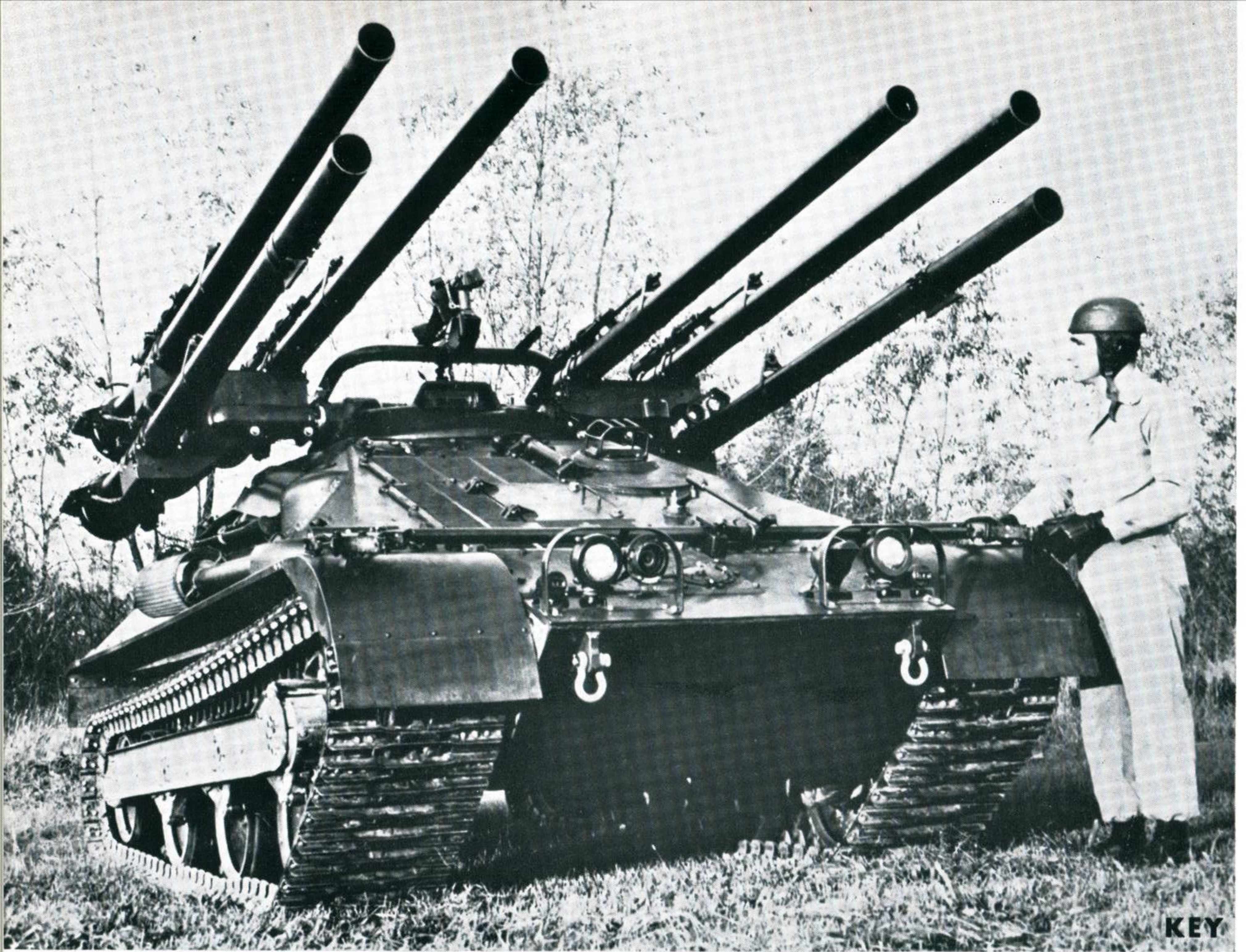
UNITED STATES M50 Ontos 106-mm Self-propelled anti-tank gun
