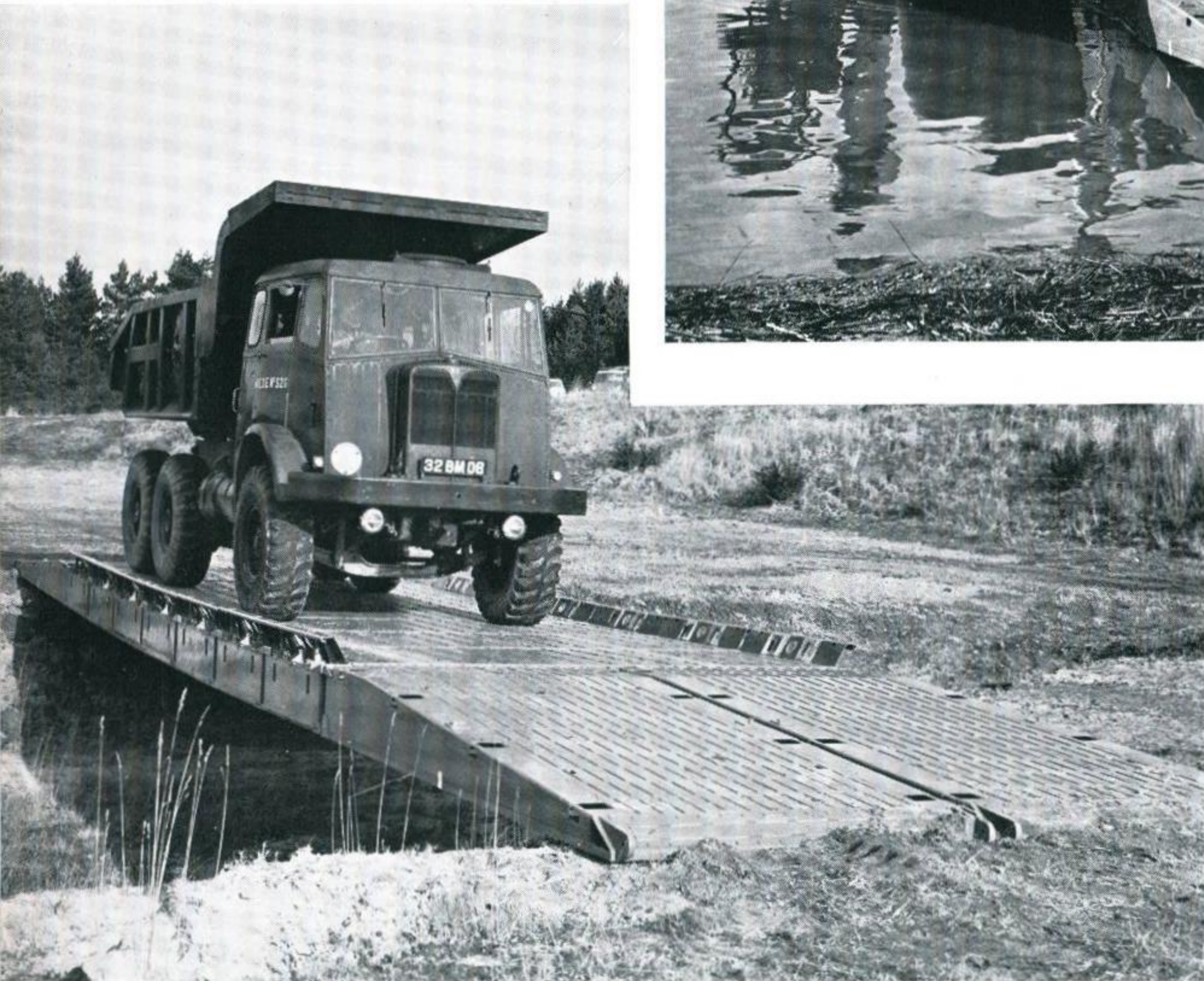
The dual roles of the Class 16 Bridge (Airportable)—as a floating bridge ferry or providing a 50-foot clear span. The picture above shows part of MEXE's waterfront at Christchurch.
