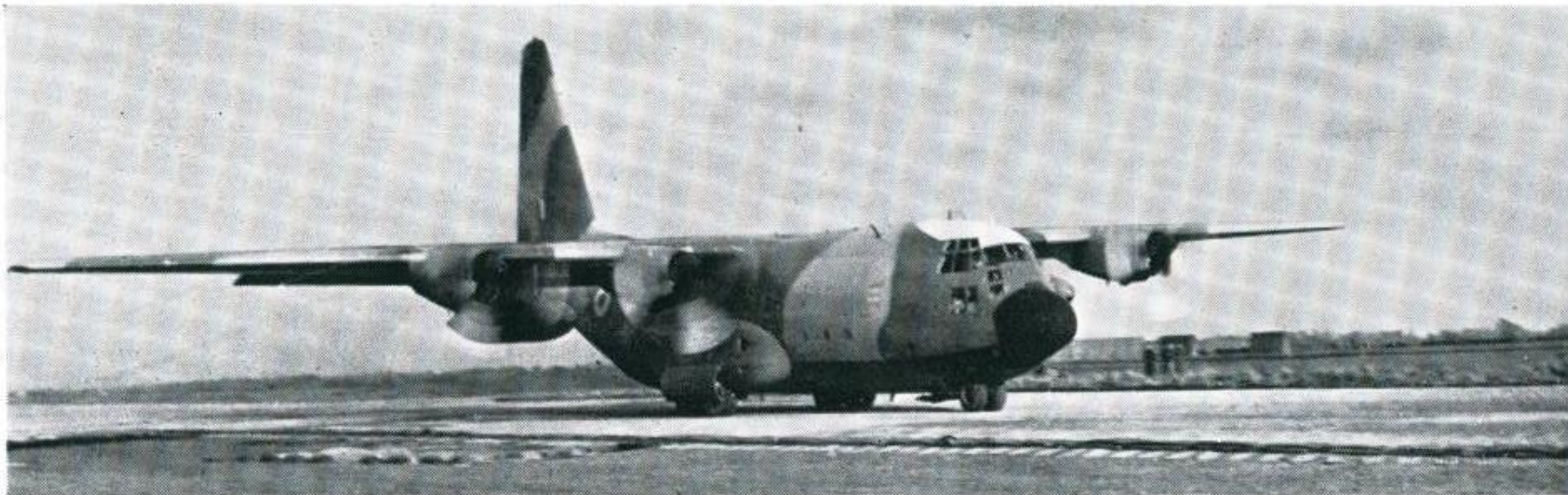
Hercules on a PSA1 runway, which is intended to provide a load bearing surface over soft ground. This is made up of 9 foot panels of interlocking light alloy extrusions laid in a brickwork pattern.
