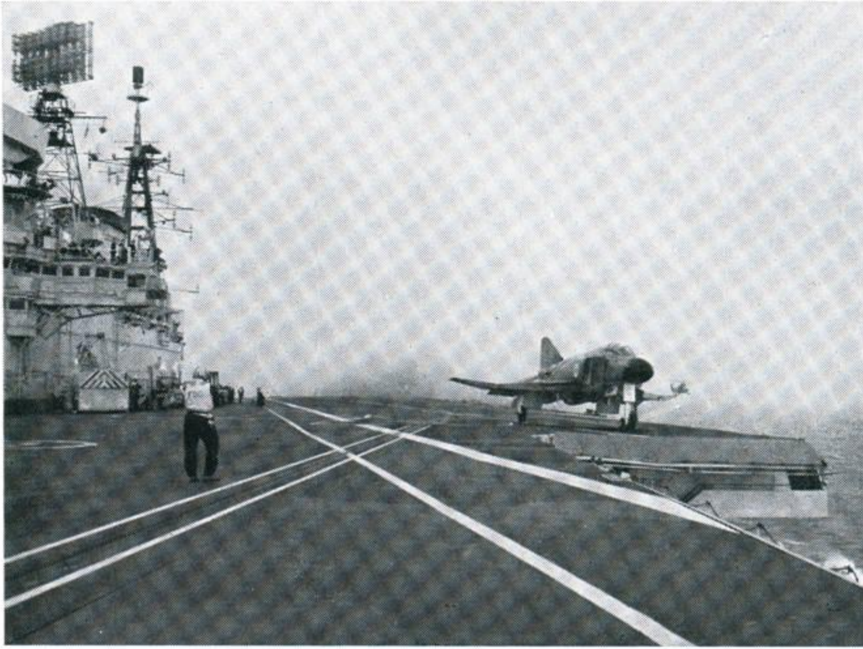
Cover Photo: A Phantom on "Touch and go" exercises aboard H.M.S. Eagle. These exercises are the preliminaries to fully arrested landings which take place later.
