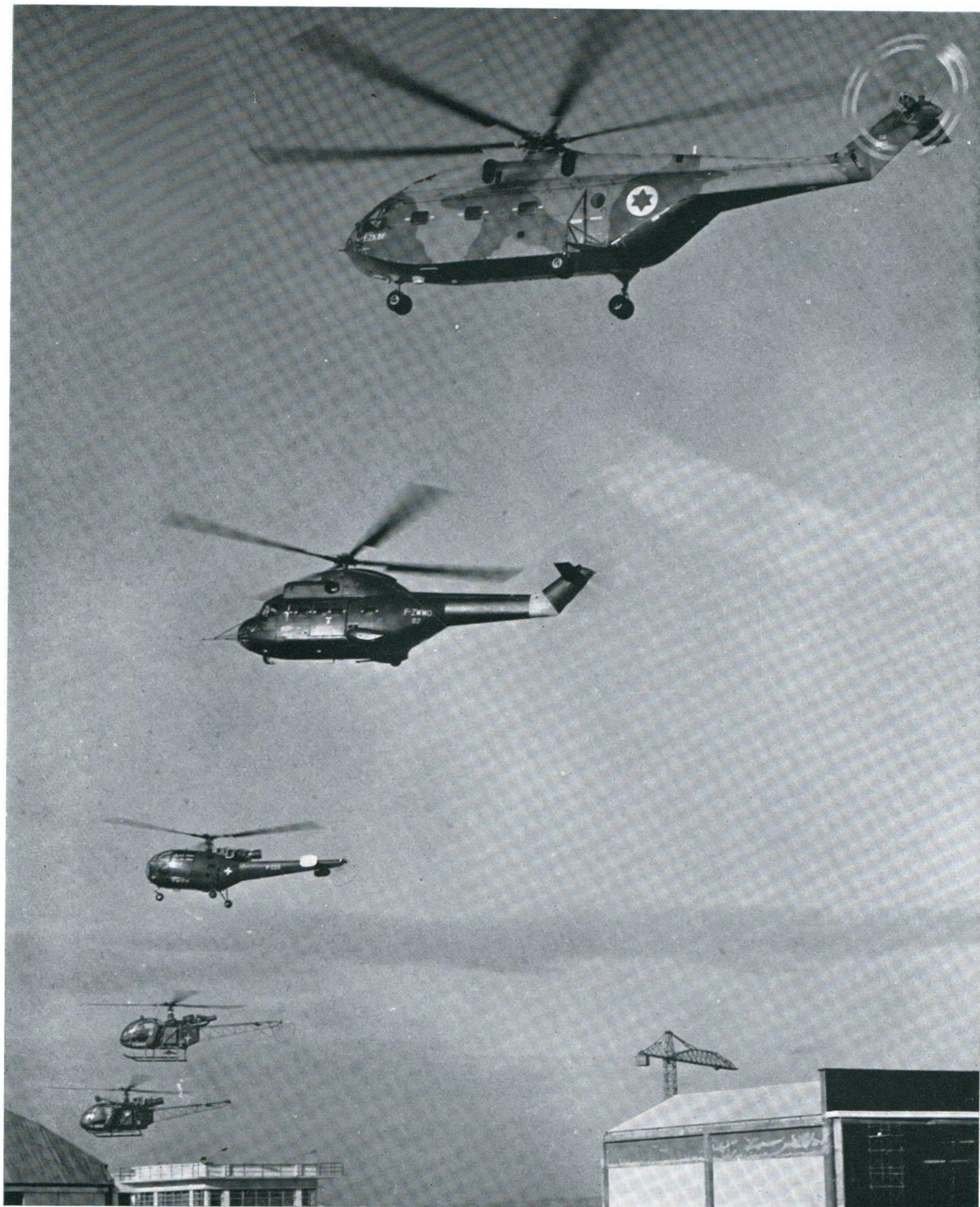
A FORMATION OF SUD-AVIATION HELICOPTERS. Left to right: SE313B Alouette II (Artouste IIC engine), SA318C Alouette II (Astazou engine), Alouette III, SA330 transport helicopter and Super Frelon in Israeli military insignia.
