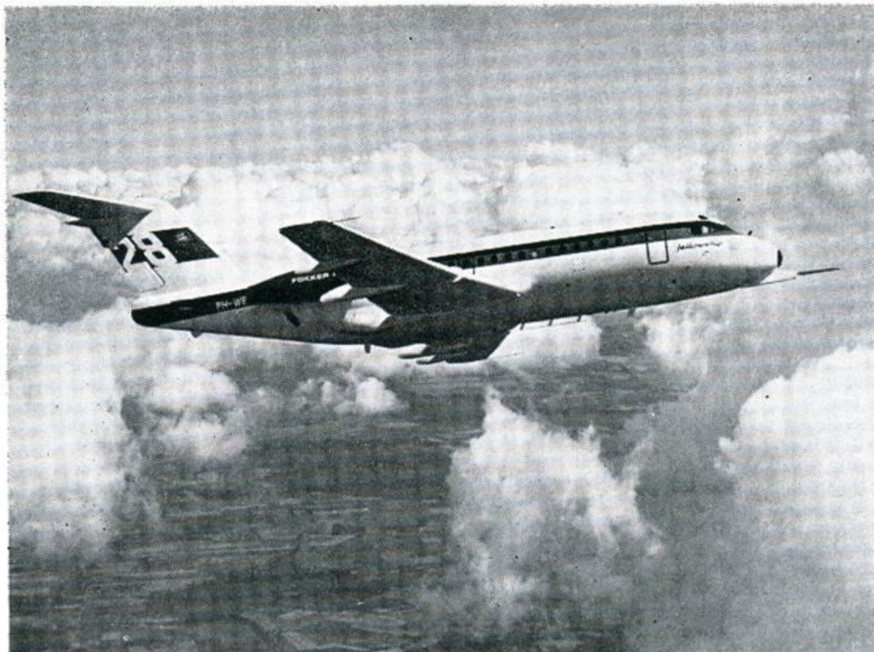
Cover Photo: The Fokker Fellowship is a high performance transport for short and medium ranges and is powered by two turbofan engines. Equipped with low pressure tyres it is able to use runways of small carrying capacity and a length as short as 3,900 feet. It can carry up to 65 passengers and is an ideal feeder airline.
