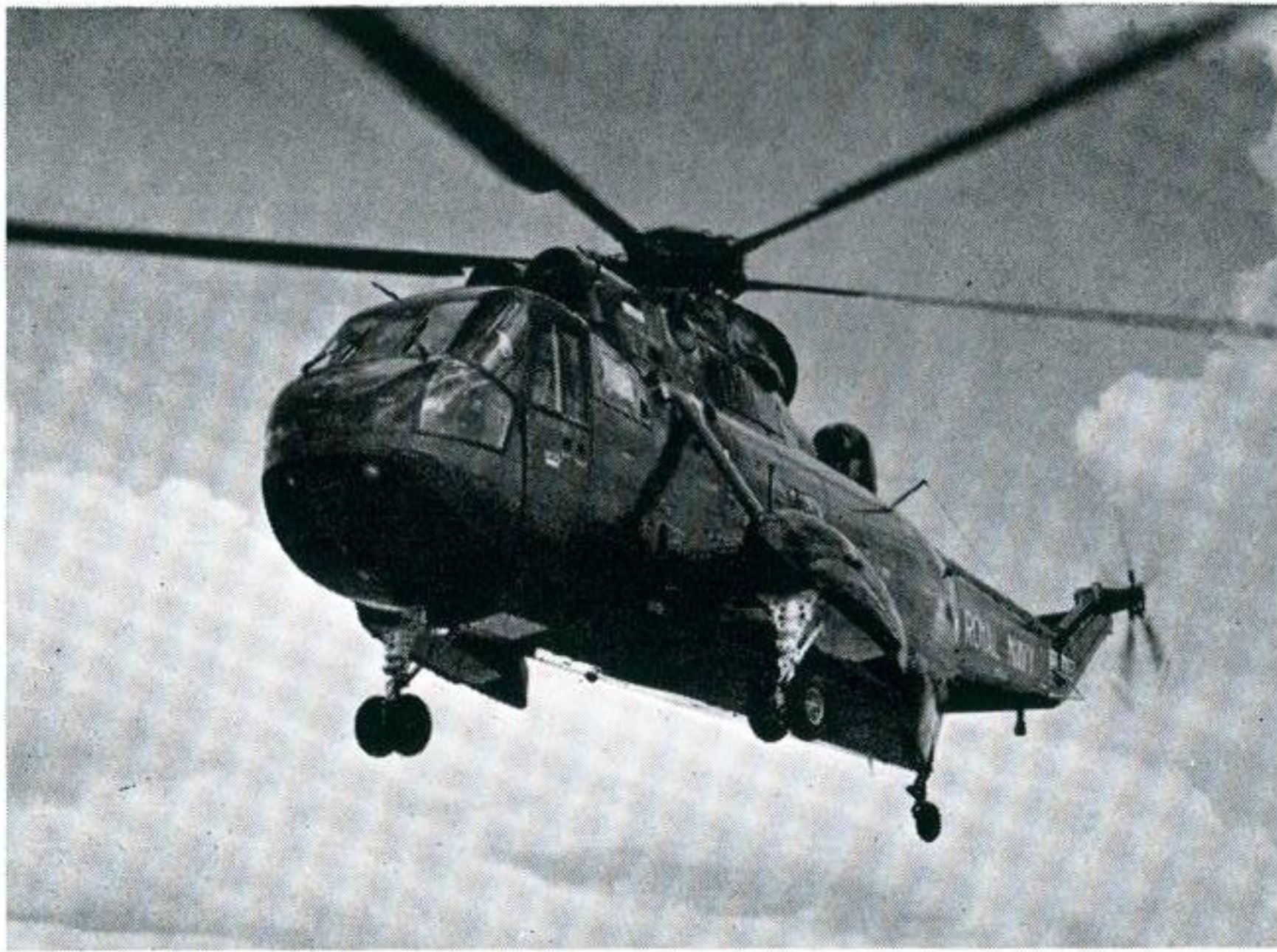
Cover Picture: The Westland Sea King helicopter powered by two Rolls-Royce Gnome gas turbine engines is intended for operation with the Royal Navy in anti-submarine search and strike roles.
