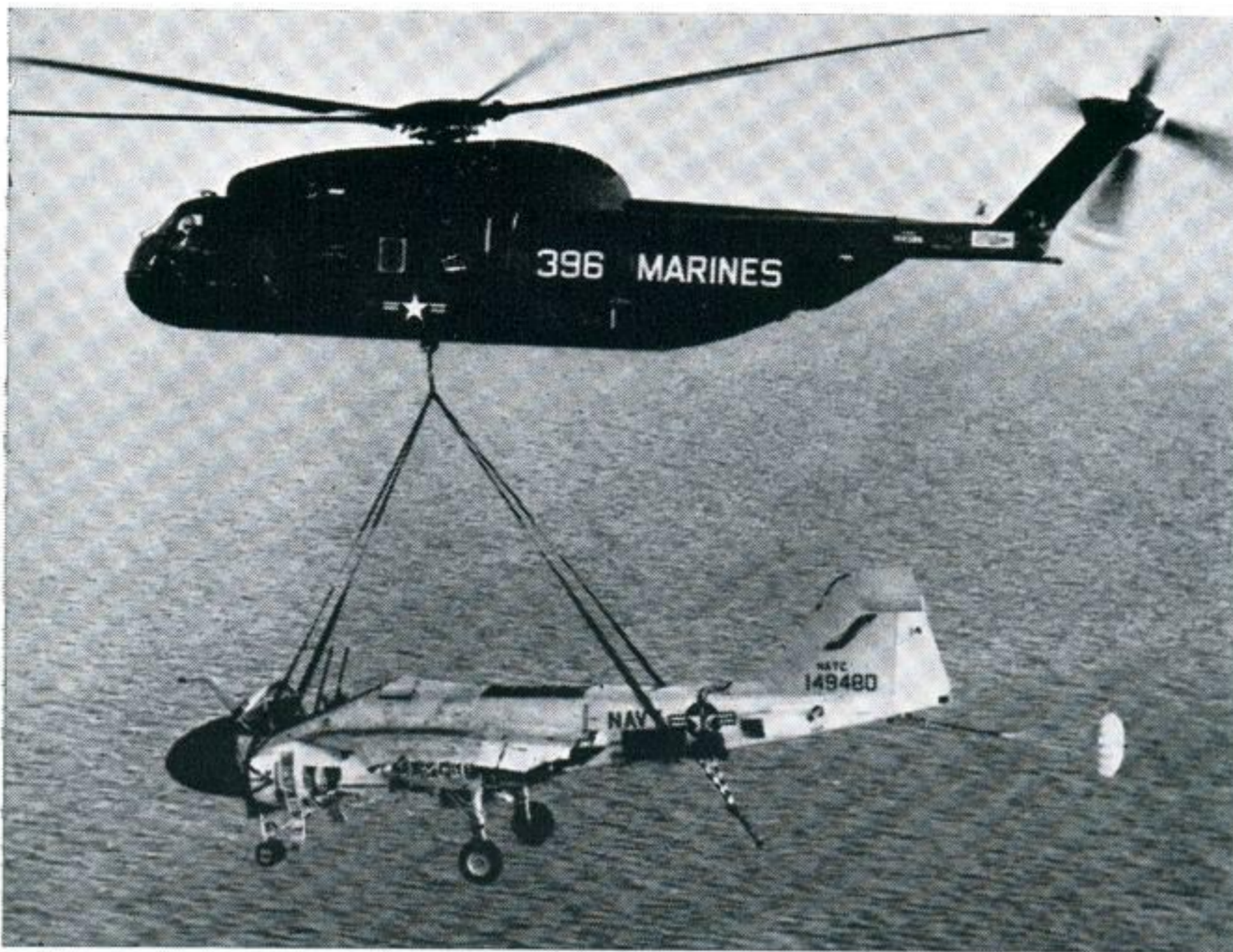
Cover Photo: United States Marine Corps Sikorsky CH-53A Sea Stallion airlifts an A-6A Intruder jet back to the U.S. Naval Air Station, Patuxent River, after the A-6A had made a forced landing in a nearby swamp. The CH-53A is used in Vietnam for troop and cargo transportation and/or aircraft retrieval.
