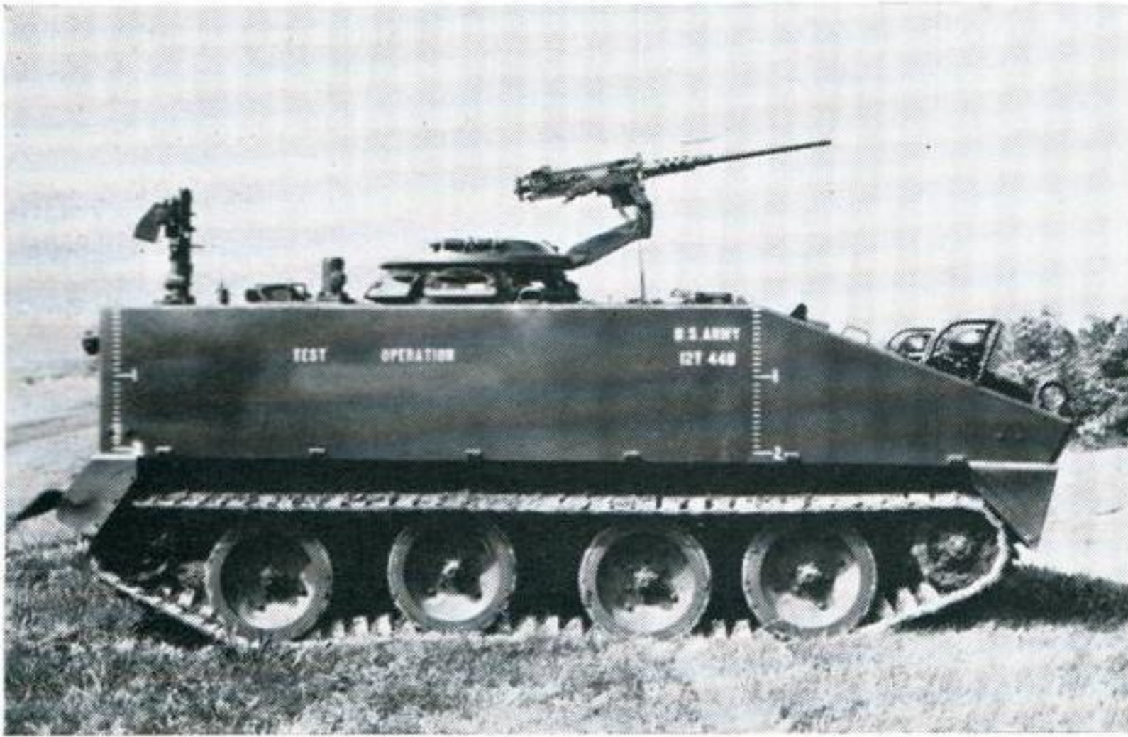
A small armoured carrier somewhat similar to the U.S. M113 armoured personnel carrier but intended for a reconnaissance role rather than carrying infantrymen for dismounted action. Some fitted with a 20-mm. gun.
