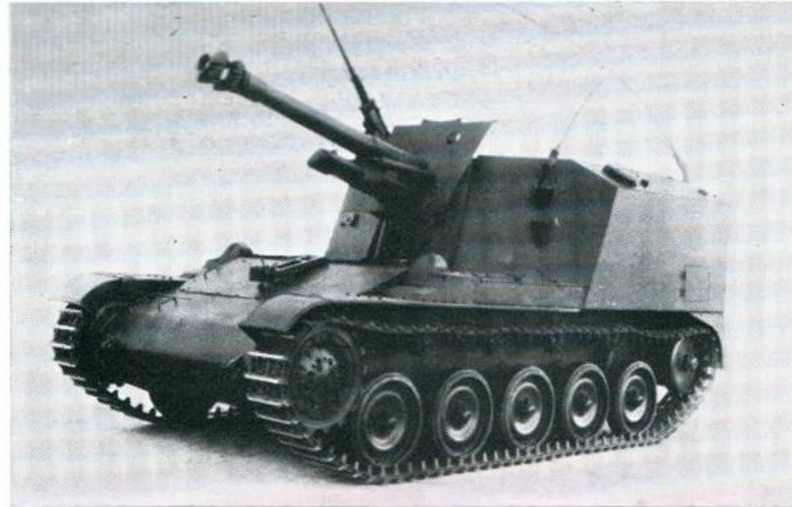
Self-propelled howitzer based on the chassis of the AMX 13 light tank. Succeeded by an improved model, somewhat similar to the Abbot, with gun mounted in a turret with all-round traverse, instead of a fixed superstructure.
