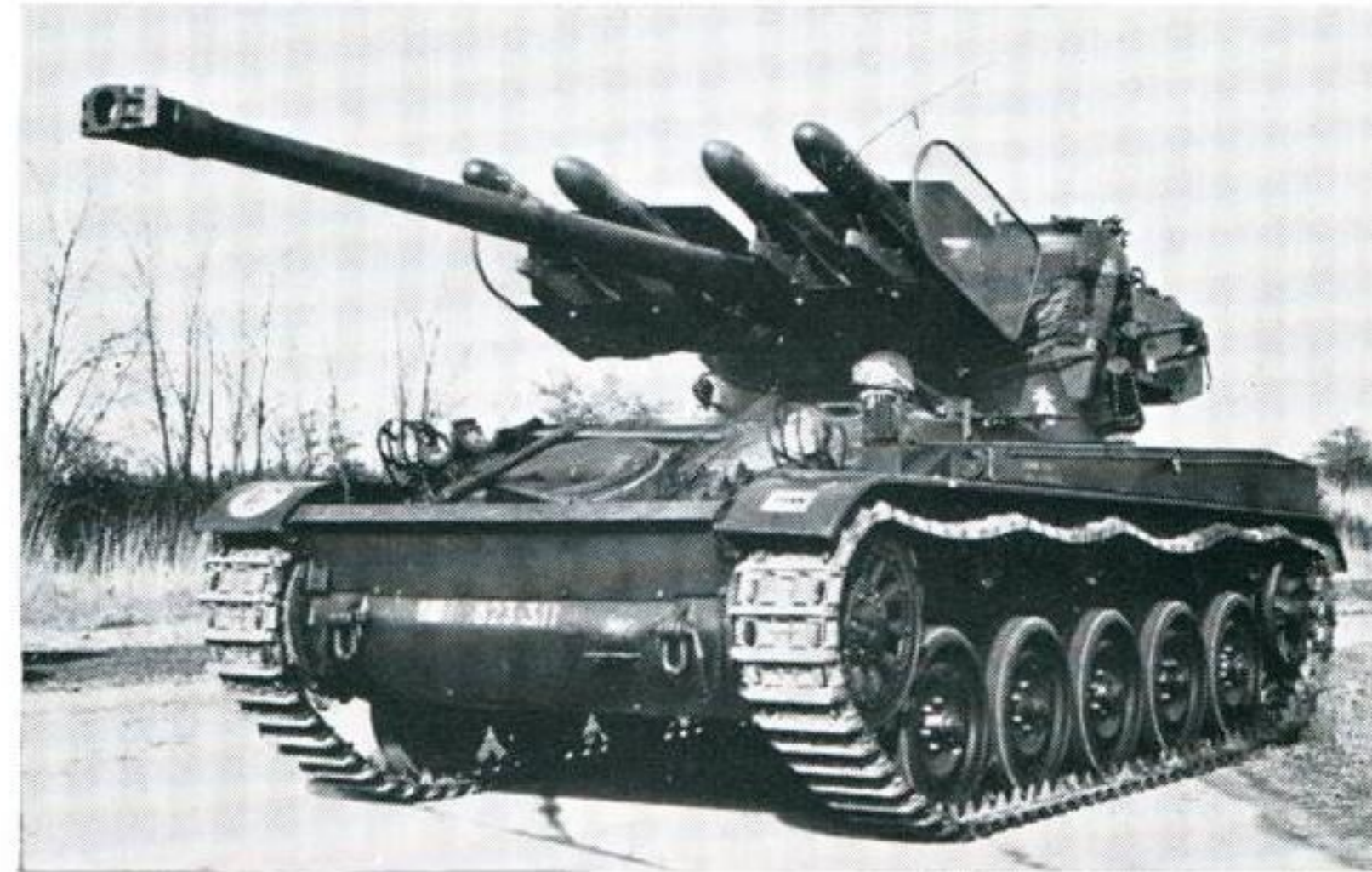
AMX 13 fitted with a launch and guidance system for four ENTAC anti-tank guided missiles which converts this light tank into a long-range tank destroyer. Retains the original high-velocity 75-mm. gun for engaging targets at shorter ranges.
