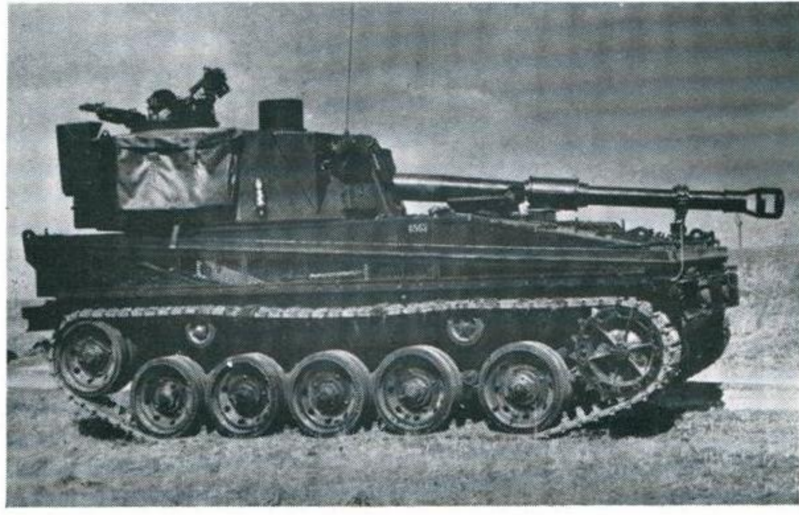
Self-propelled 105-mm. gun with the main armament mounted in a turret with all-round traverse. Chassis similar to that of the F.V.432 armoured personnel carrier and like the latter carries a collapsible flotation screen.
