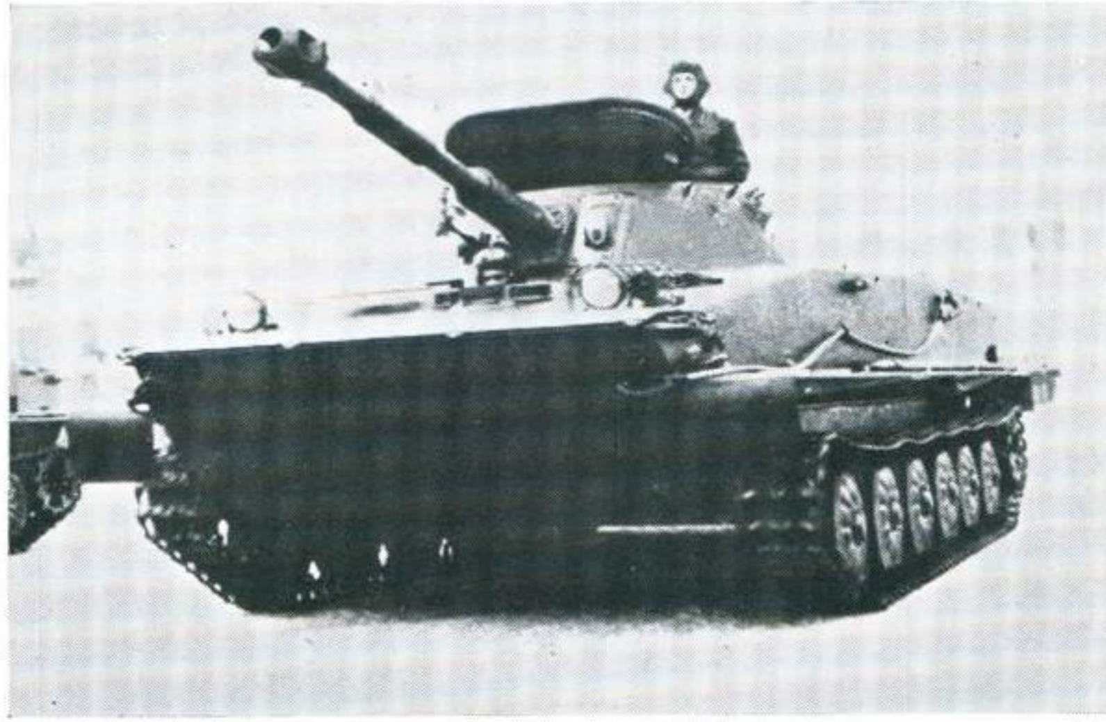
Widely used amphibious reconnaissance tank. Relatively large in relation to its weight and armed with a medium-velocity 76-mm. gun. Swims with the aid of a water jet propulsion unit.
