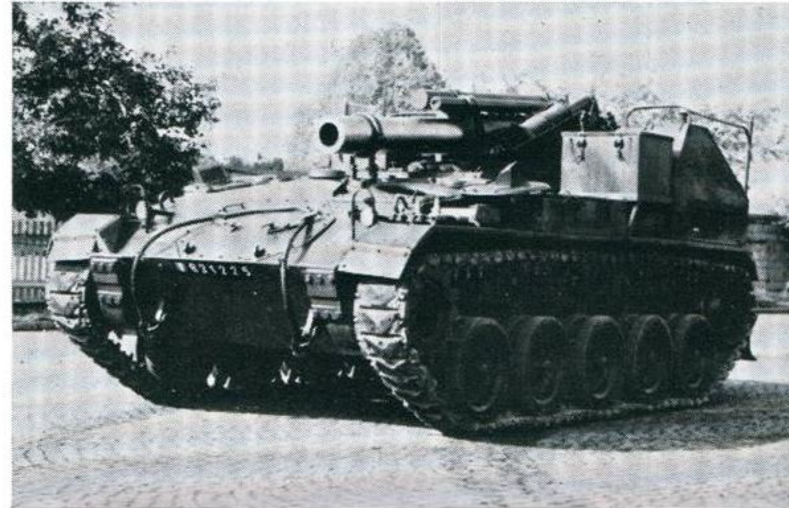
Ageing, United States-built 155-mm. self-propelled howitzer still used by the French Army. Chassis similar to that of the U.S. M24 light tank. Offers limited protection to its crew.
